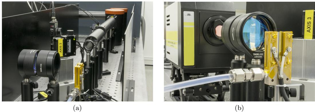
Figure 3.5: Photographs of (a) beamline with attenuation stage, photodiode pulse energy detection stage, and APPJ. (b) shows the APPJ mounted vertically on the 3-axis motorised stage, detection optics, and iCCD with filter.
