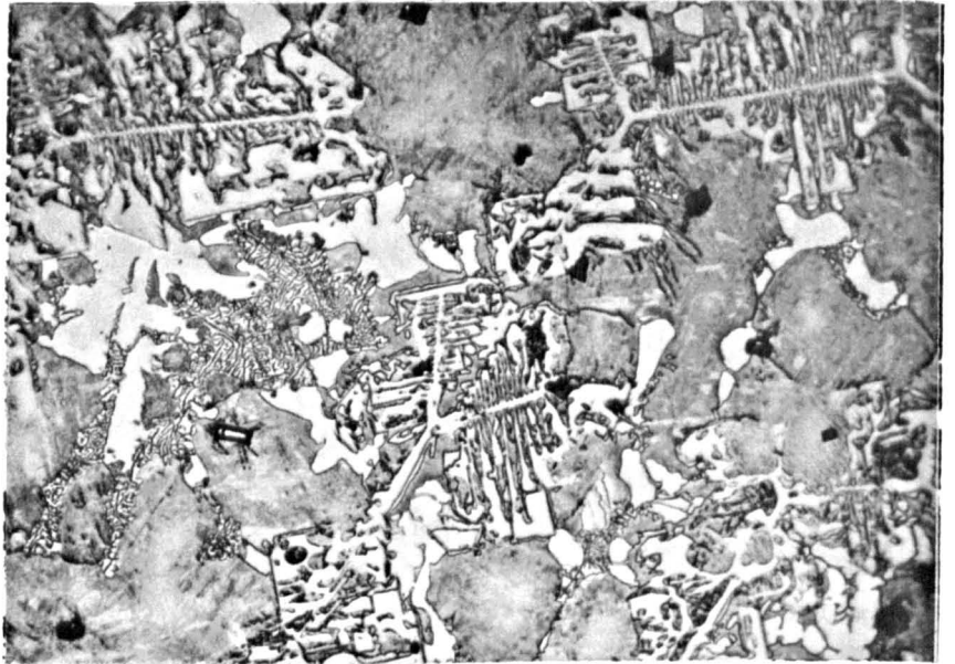
REGIONS OF FINE SCALE DENDRITIC, FACETTED AND EUTECTIC STRUCTURE BETWEEN PRIMARY DENDRITES x 200 SAMPLE 133 FIG. 3.26b
