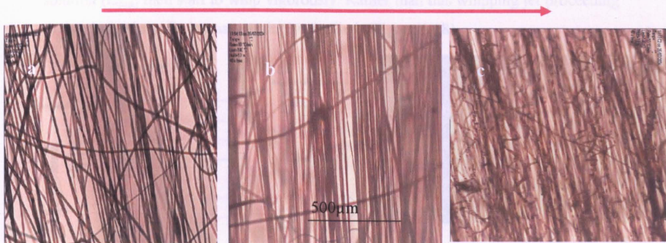
Figure 6.17 PDLA fibres spun from a solution of 40wt% PDLA in DMF. a)rotation speed 200 r.p.m b) 550 r.p.m c) 650 r.p.m.
