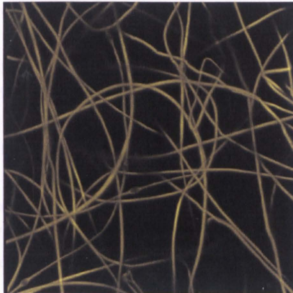
Figure 5.12 Rhodamine-laden PLLA fibres(spun from 7.5wt% PLLA in DCM with 0.5wt% rhodamine) showing even distribution of dye throughout the fibres. It is expected that a drug which was soluble in the spinning solvent would be distributed as evenly as the rhodamine is in this system.
