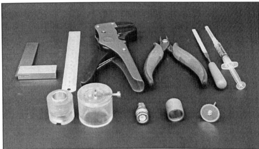
Figure A2: Some materials, accessories and tools for making bender element probes (left to right)-
