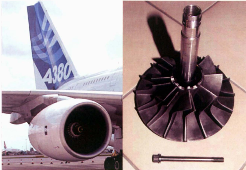
Figure 2.1 The turbine engine of an Airbus A380 containing large amounts of Titanium and an example of a titanium compressor section taken from a Solar T-62T-32 engine ( www.technologie-entwicklung.de /Gasturbines.html , 2005).
