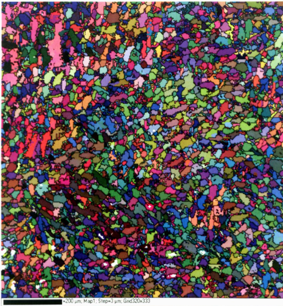
Figure 6.19 OIM of heat treated sample
