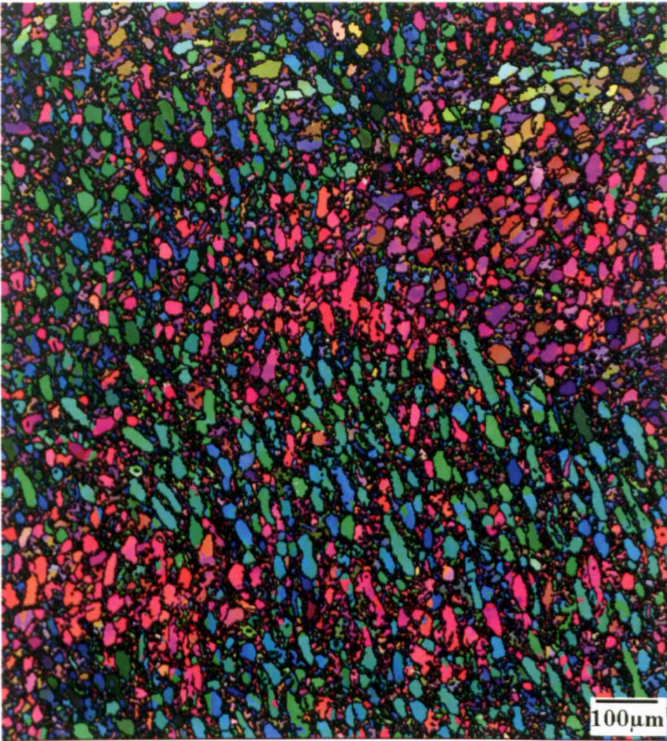
Figure 6.30 Euler colouring OIM of specimen T17 having received \epsilon=0.55
