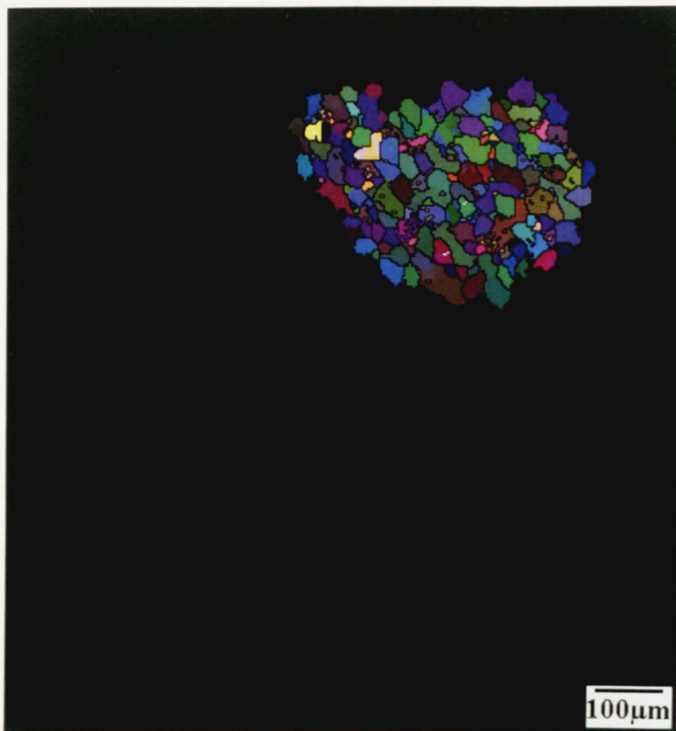
Figure 8.7 Clustered zone of similarly orientated grains
