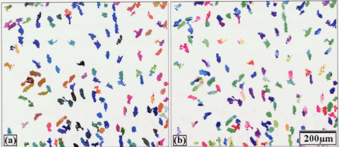
Figure 8.84 \alpha_p OIM's of the D8 sample in (a) Euler and (b) IPF colouring
