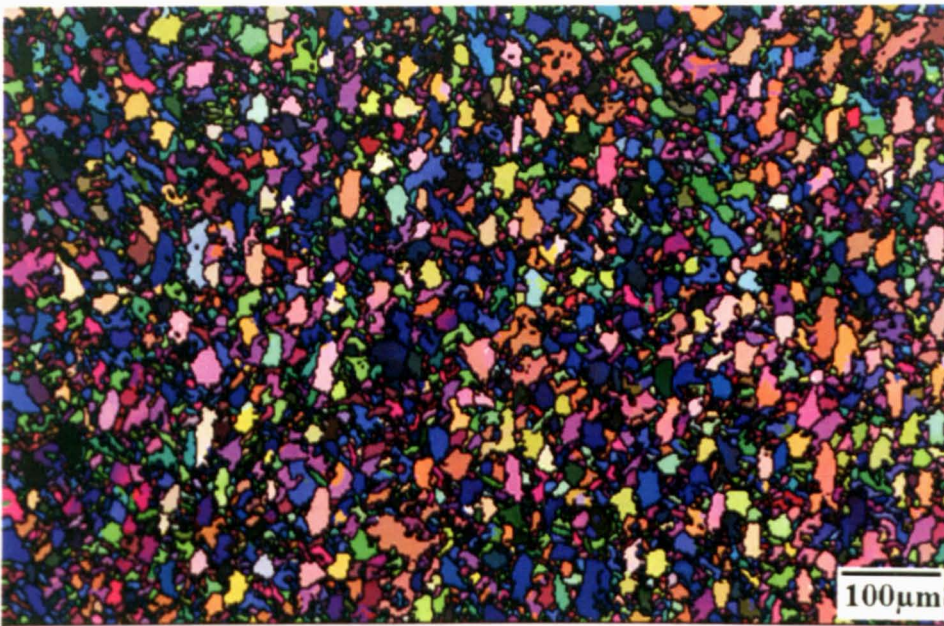
Figure 6.46 A10 Euler colouring OIM of specimen D10
