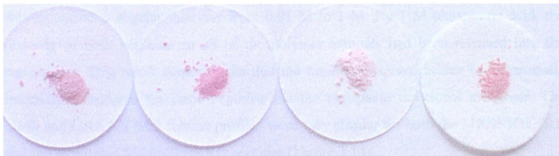
Figure 3.13: Polymer samples with bound MRSSSDKPRR peptide at 0.05 M phosphoric acid showing colour change (L-R) DKPRR CS-MIP, Blank CS-MIP, core particles, GAA CS-MIP. DKPRR-imprinted CS-MIP remains orange, whereas the other three samples turned red/pink, which is associated with the protonated form of methyl red.
