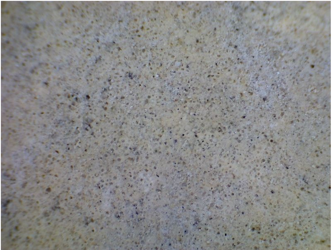
Figure 108: Tadcaster magnesian limestone, late fourteenth century (x50 approx.)
