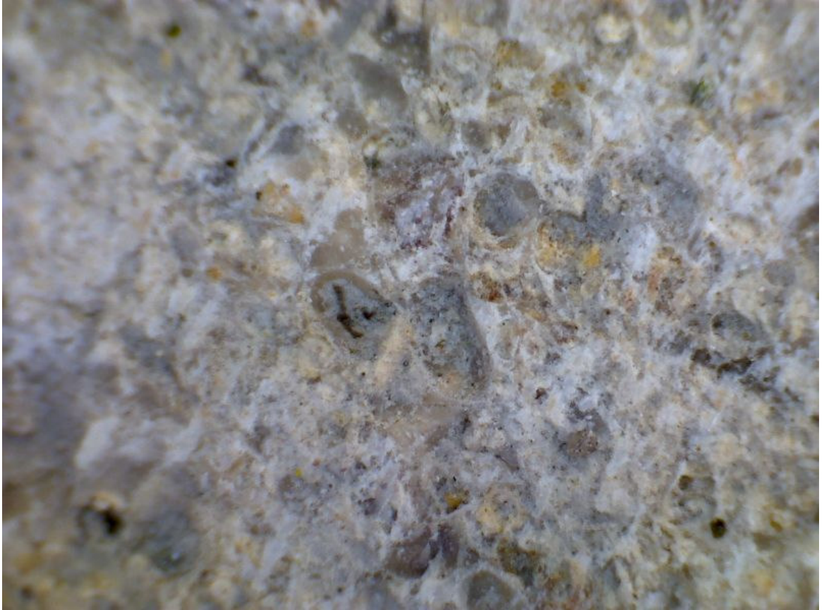
Figure 122: Clipsham oolitic limestone, 1920s-1960s (x50 approx.)
