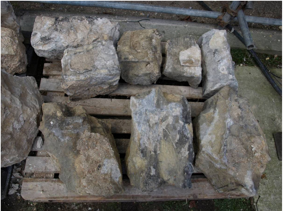
Figure 297: Re-used fragments of previous corona (?eighteenth century) found within core of upper courses of south buttress, Level F
