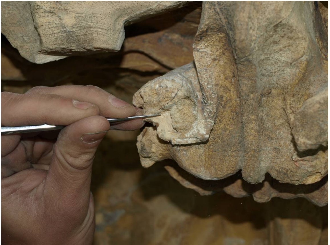
Figure 152: Carved stone treated with linseed oil showing powdering substrate beneath
