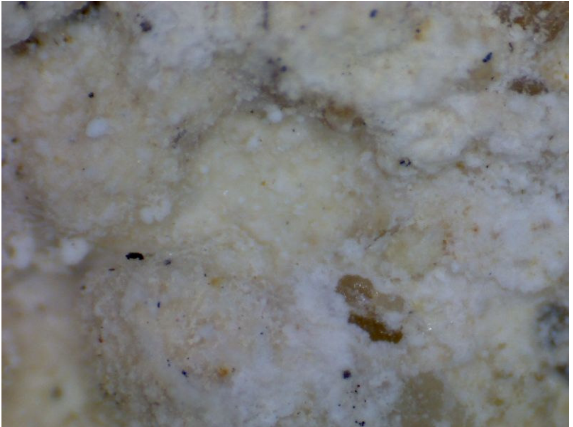
Figure 140: Early nineteenth-century lime mortar, 1820s (x200 approx.)
