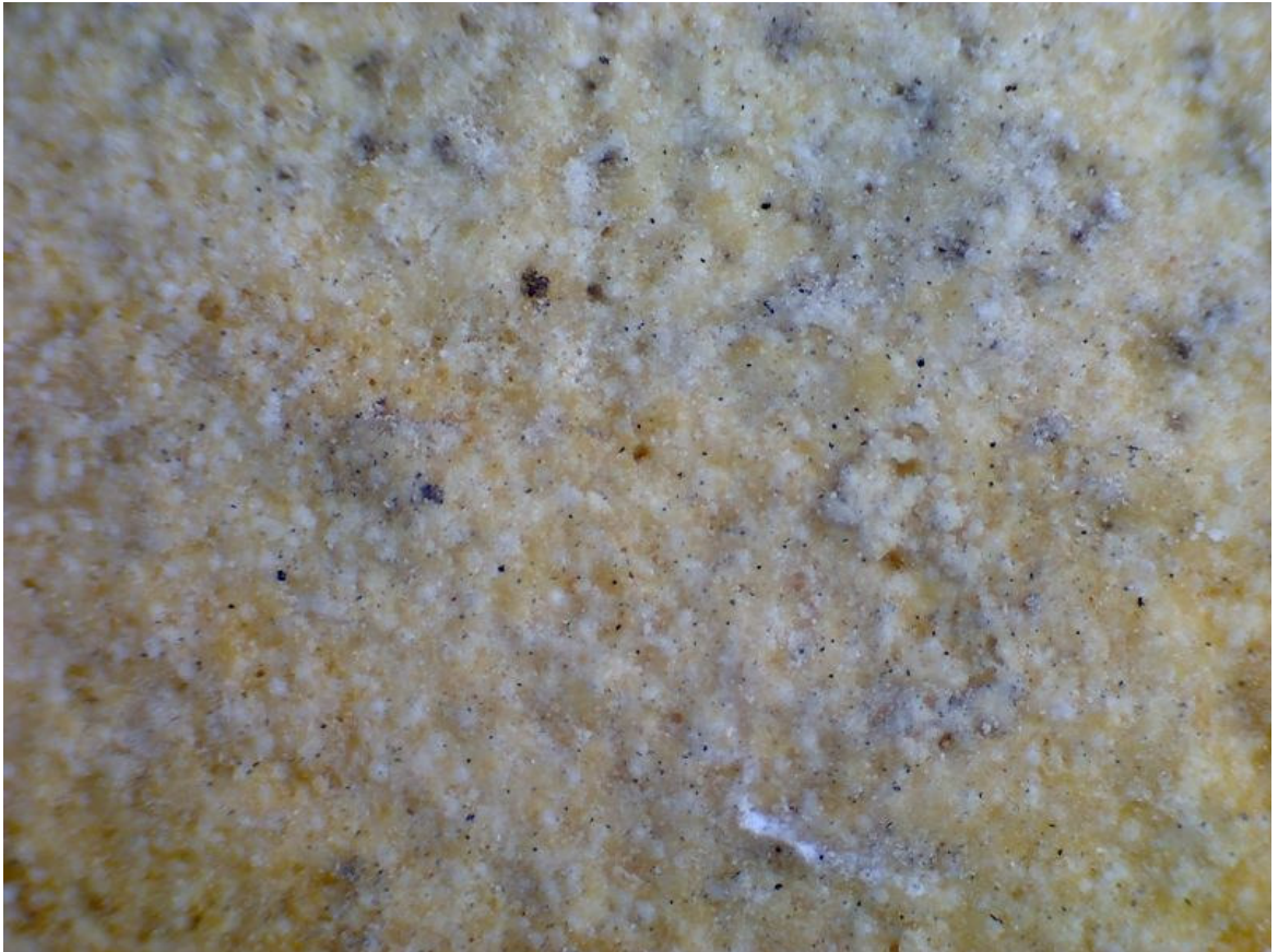
Figure 110: Tadcaster magnesian limestone, 1820s (x50 approx.)
