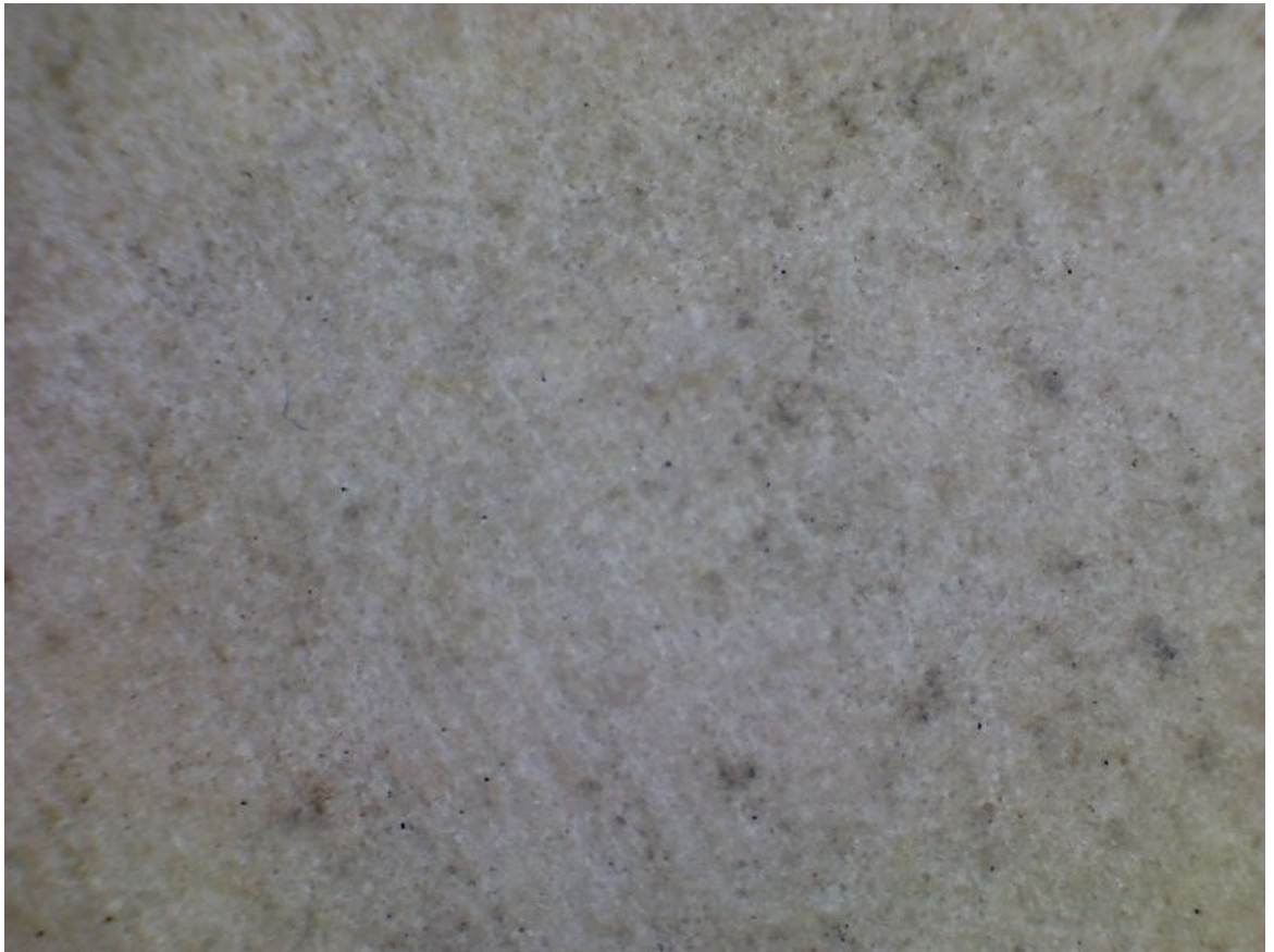
Figure 112: Huddleston magnesian limestone, late fourteenth century after 1385 (x50 approx.)
