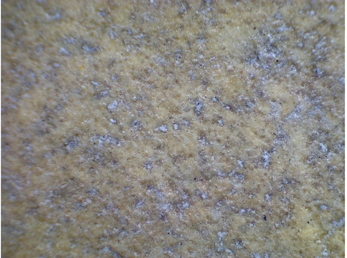
Figure 118: Cadeby magnesian limestone, 1970s-1980s (x50 approx.)
