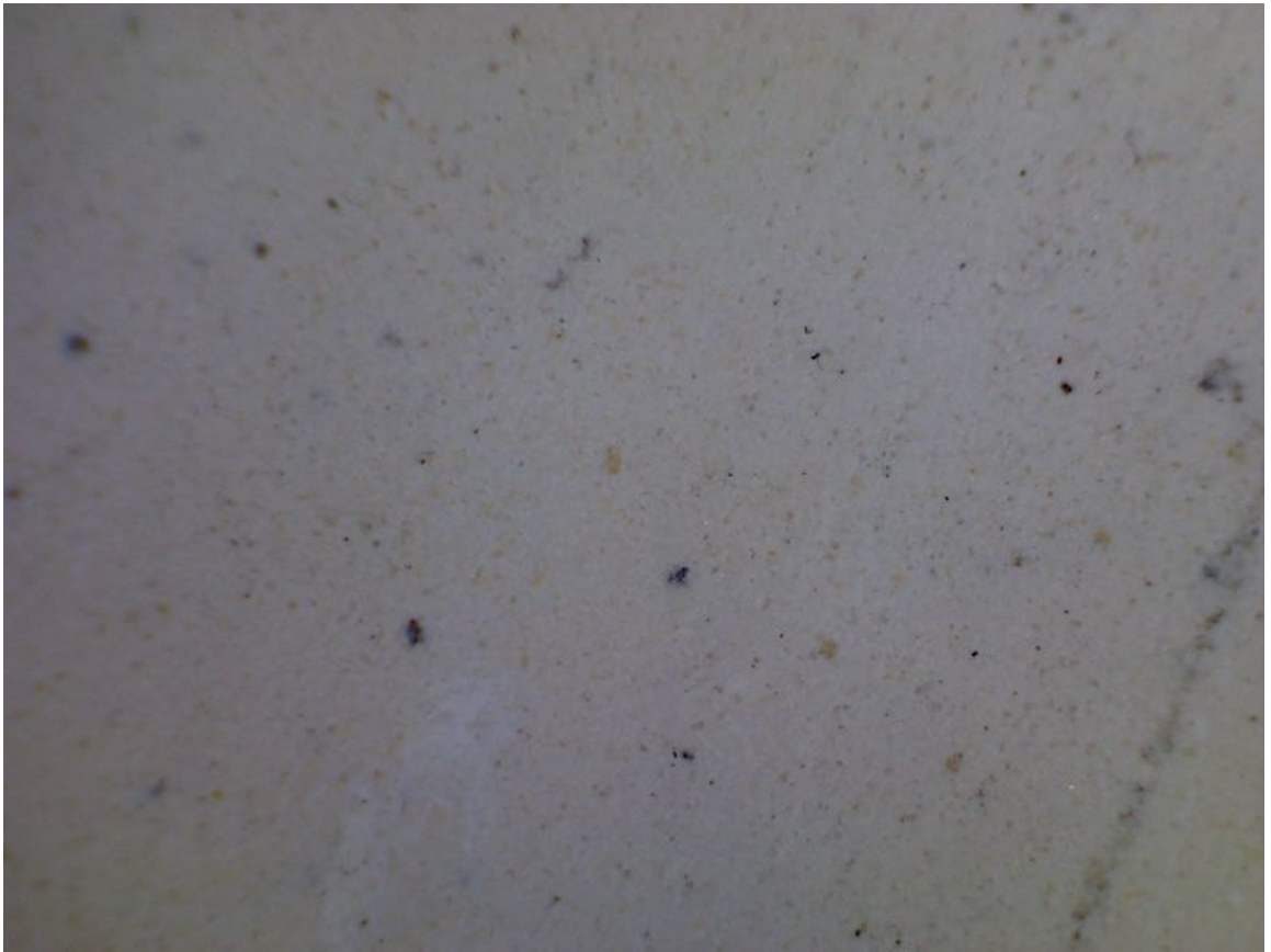
Figure 126: Warmsworth magnesian limestone, c.2006 (x50 approx.)
