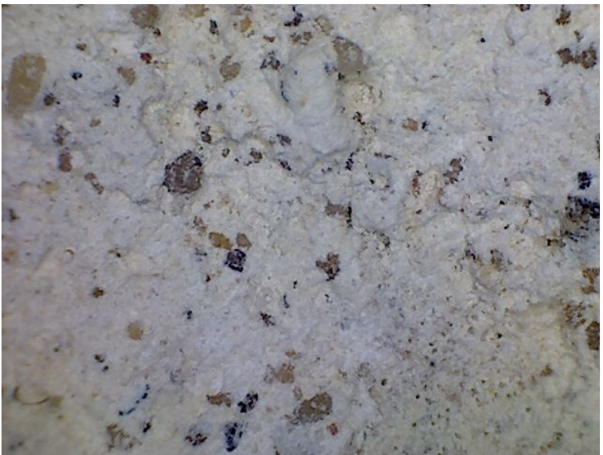
Figure 135: Fourteenth-century lime mortar (x50 approx.)
