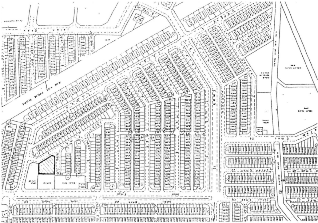
Figure 5.7 Typical grid-iron layout of urban housing neighbourhood planning. Note the provision 10% green open spaces in meeting requirement of planning regulations.
