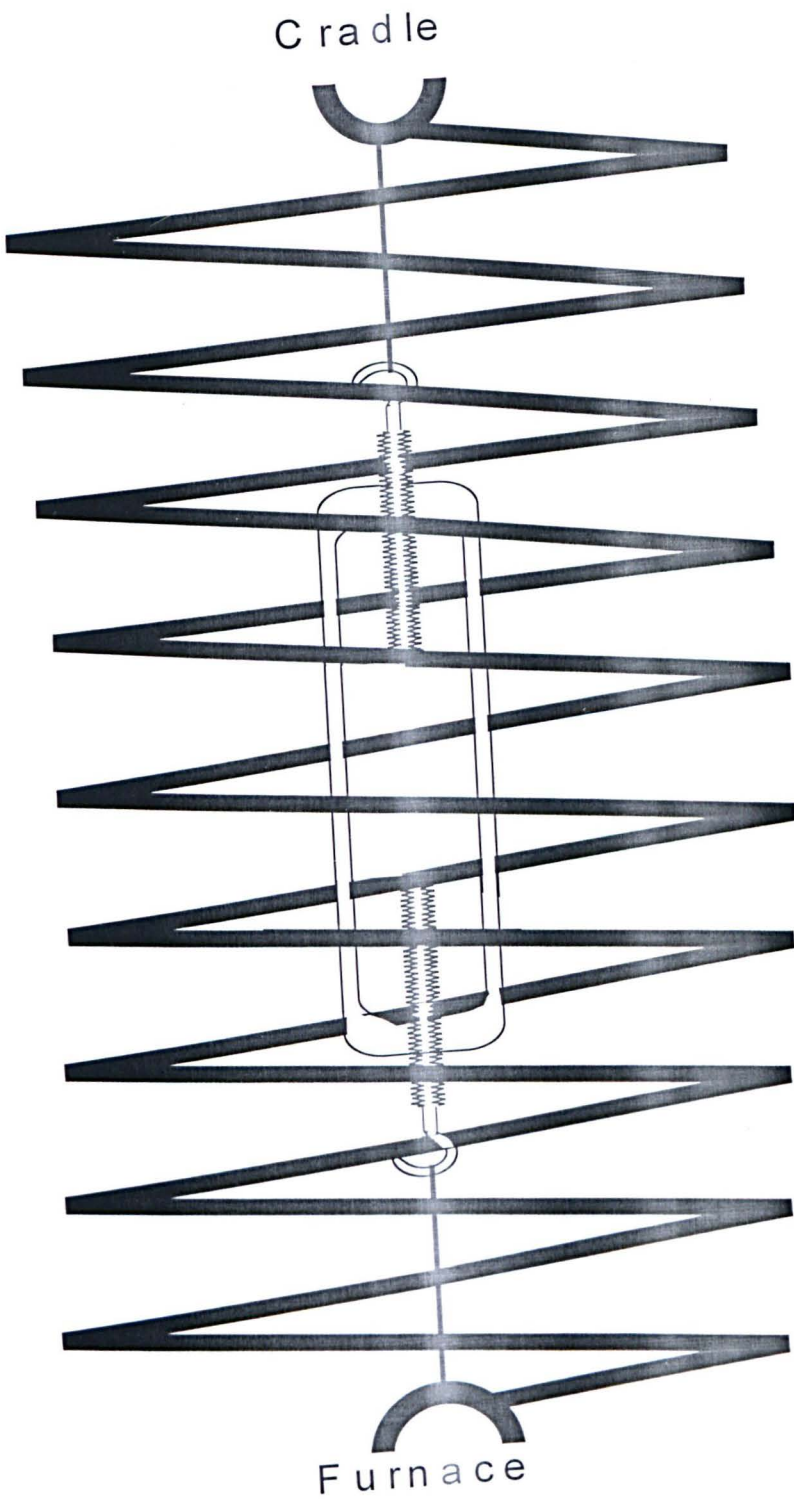
Figure 8.3 Sketch of the furnace suspension system
