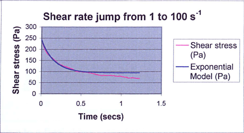
Figure 6.1.4f: Curve fitting of shear rate jump starting from an initial shear rate of 1 s -1
