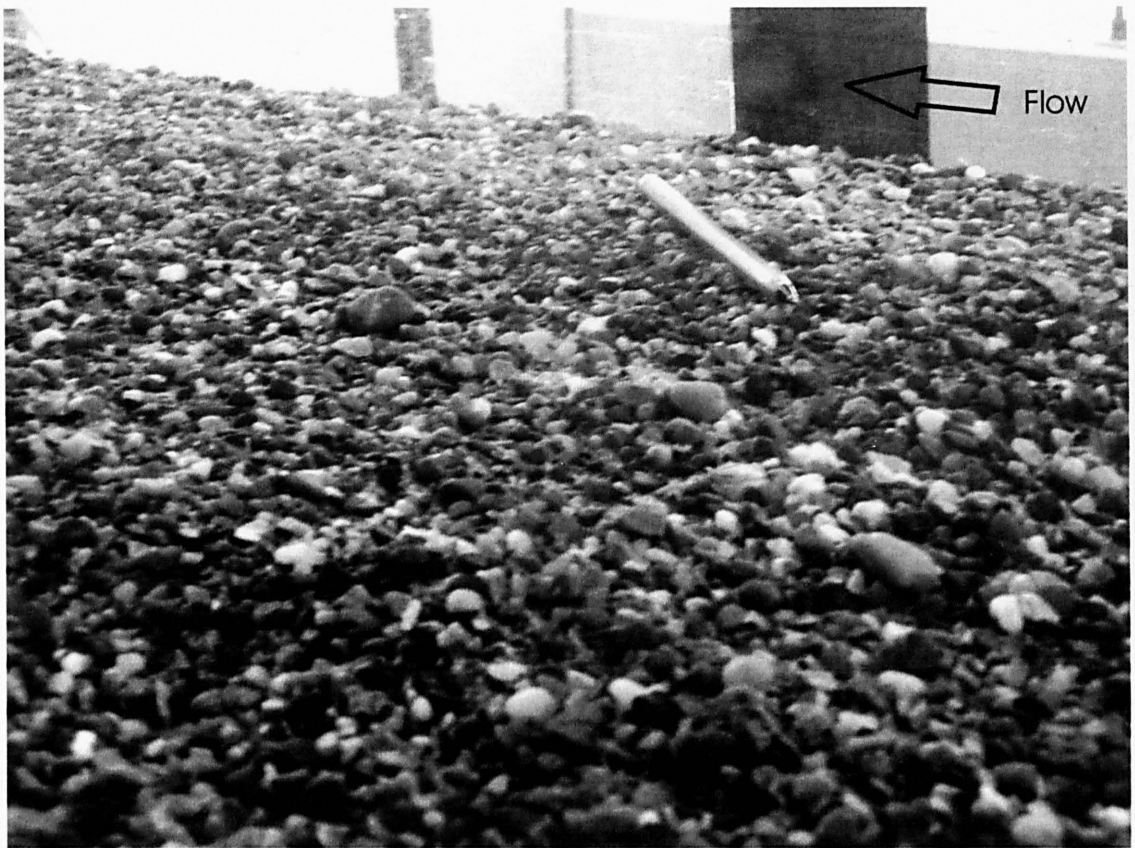
Figure 3.8. The surface of the sediment deposit formed through feeding of the unimodal mixture after 3 hours. Even after a short period of feeding the surface exhibits properties of a water-worked bed with a high level of particle imbrication, preferential alignment of the particles in the direction of the flow (diagonally from right to left) and the presence of particle clusters. This was later covered through further feeding, demonstrating that the whole depth of the deposit has an imbricated form. A pen is added for scale.
