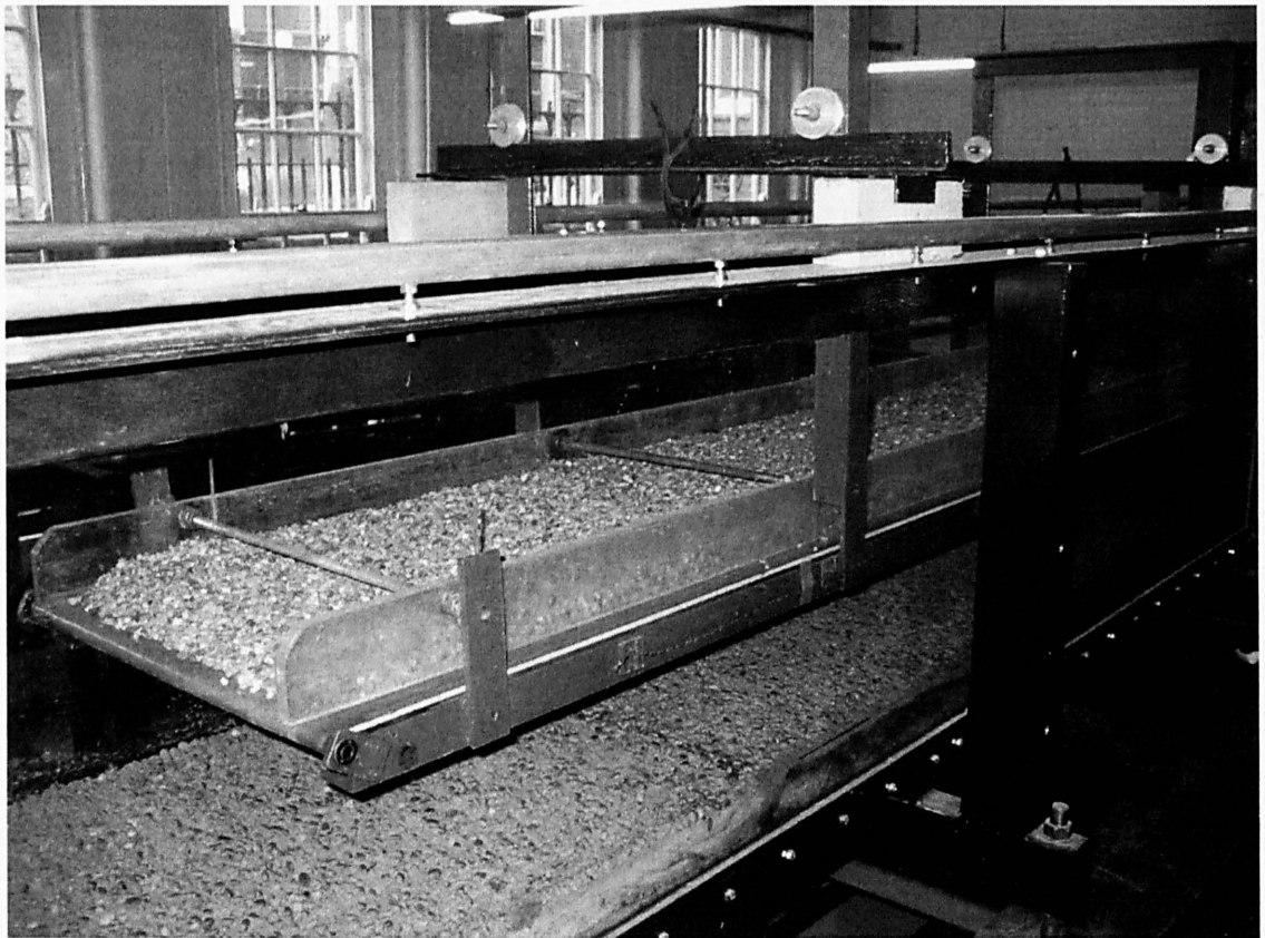
Figure 3.6. The conveyor belt loaded with sediment that was used to form each of the two water-worked gravel-beds. A fixed bed section is shown underneath on which the sediment fell and saltated over until falling into the steel floor section of the flume.
