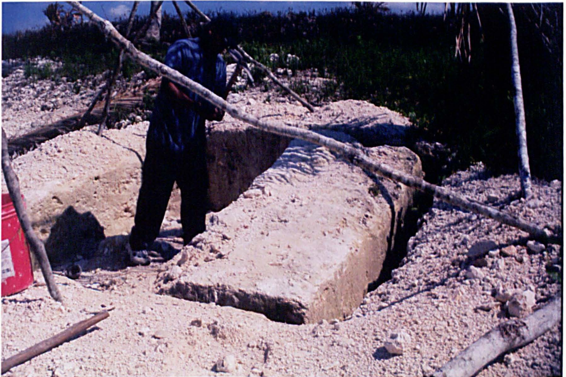
Plate VII.8: Quarried block of sascab, solidified after exposure to sun and air.
