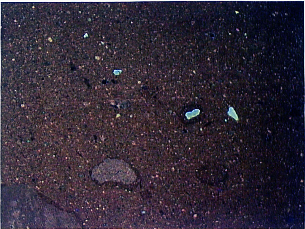
Plate VII.18: Photomicrograph of T HAR2 (fired) showing fewer aplastic inclusions (x25).
