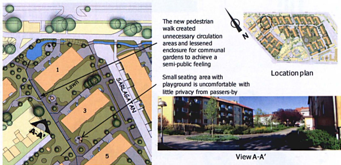
Figure 5.14 Plan and photograph showing new pedestrian walk that has contributed to the public feeling of the communal gardens in the open layouts 1 of Augustenborg (plans from ISS Landscaping; photograph by author)
