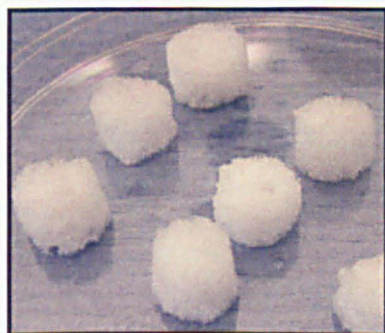
Fig. 2.4: Cylindrical PU scaffolds. Size of PU is 10 mm of diameters and 10 mm of heights.
