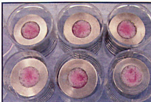
Fig. 2.5: Sterilized PU scaffolds. The scaffolds were pre-soaked with basal media in 1 cm internal diameter stainless steel rings.
