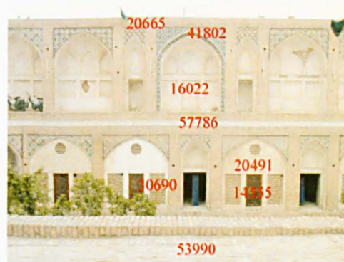
Fig 6.9. C.No.1 and C.No.15 vertical and horizontal illuminance levels in the courtyard
