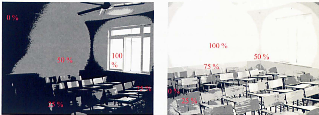
Fig 6.31. Five-zone lighting pattern of north-east classrooms under overcast sky(left) & clear sky(right)
