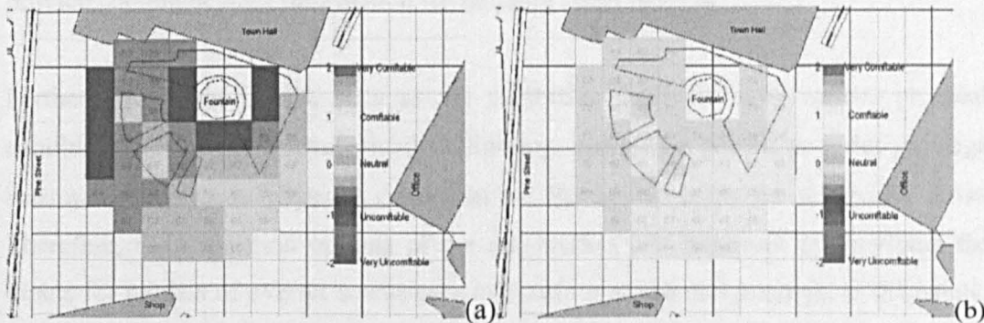
Fig. 6.3 Acoustic comfort evaluation map for different sound level experience (a) People from noisier home; (b) People from quieter home
