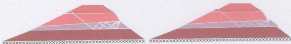
FIGURE 6.6: DLO Slope problem: optimum layout of slip lines and displaced failure mechanism
