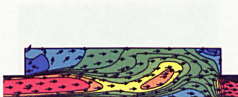
(c) – Large scale manhole ( Q = 22 l/s; Froude scaled Q = 7.98 l/s)
