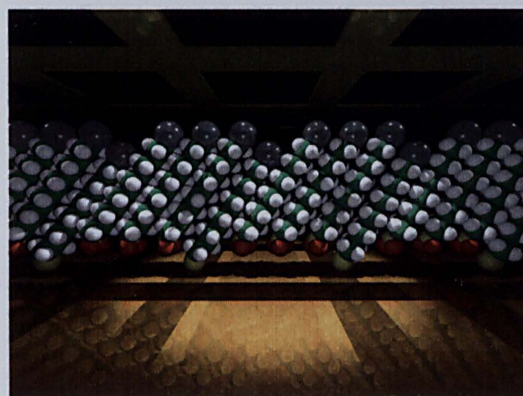
(b) In the regions of the SAM irradiated by UV, thiolates are converted to sulfonates, which are less strongly bound than thiolates
