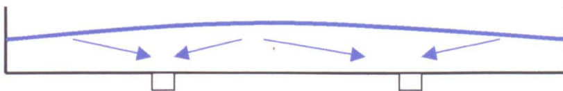
Water profile within a gutter installed with a syphonic system operating at design flow capacity.
