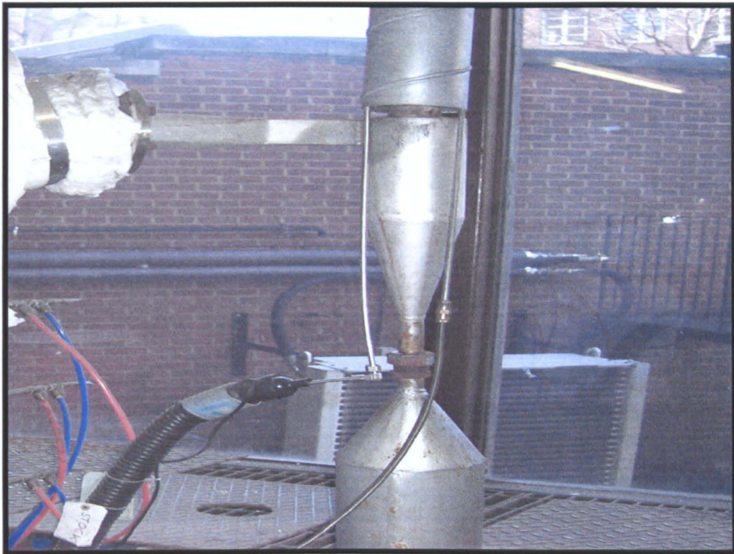
Plate 2 Cyclone and catch-pot
