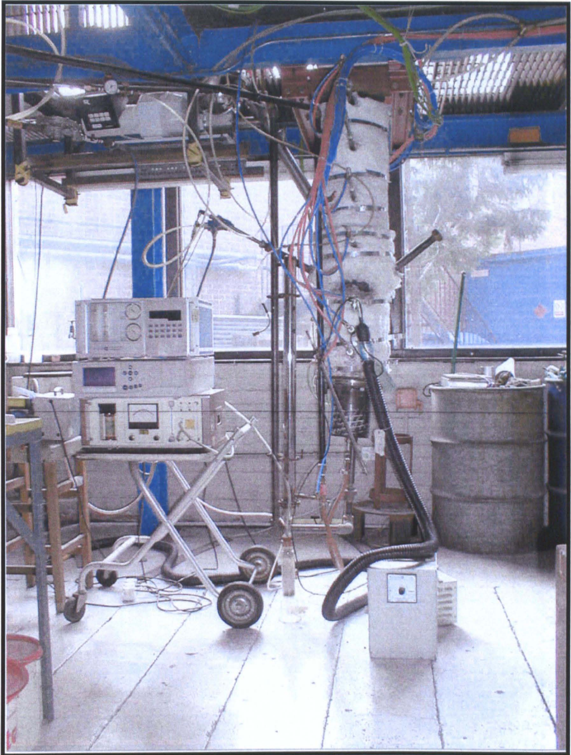
Plate 1 Rig of Fluidised bed combustor
