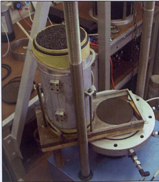
(a) Mould containing the compacted specimen placed with its base level with the porous disc sitting directly on top of the triaxial cell pedestal.
