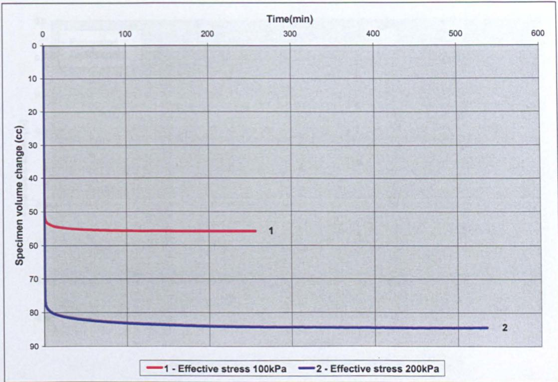
Figure 5.45 Consolidation curves at effective stresses of 100 and 200kPa for the specimens of minimum particle size of 5mm used in test series D.
