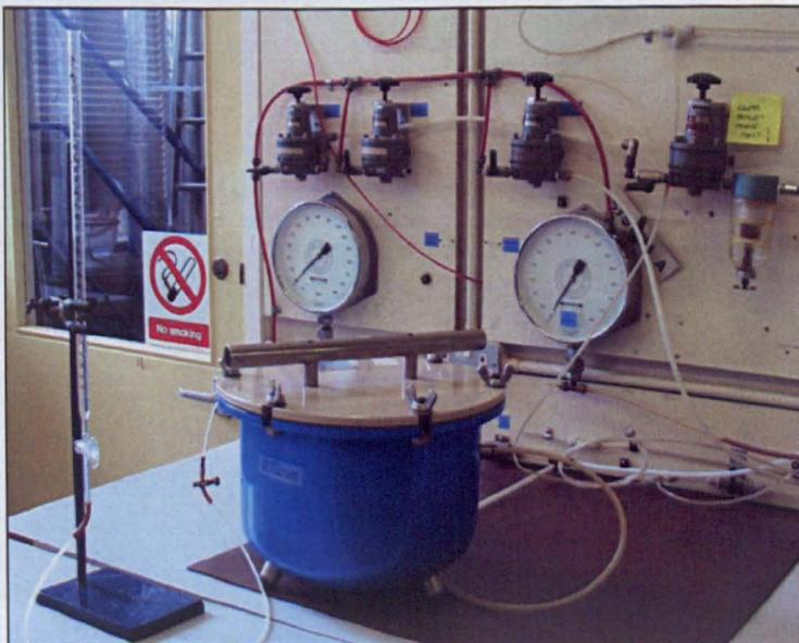
(c) Pressure plate extractor connected to a burette to collect excess water during equalization.
