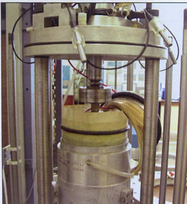
Plate 4.17 Two O-rings and the second membrane stretched around the split rings ready to be installed after the application of a vacuum and subsequent mould removal.
