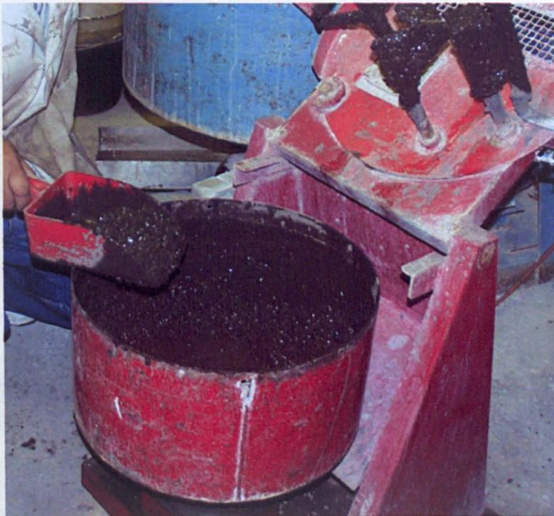
(a) The soil sample after being ground for 10 minutes to crush down the soft particles of shale.
