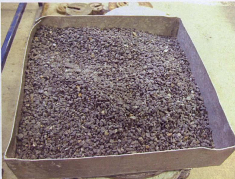
(b) Washed sample freshly removed from the oven to be cooled down before carrying out the specimen compaction.
