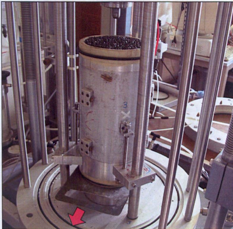
(d) The clamp system is assembled to hold the mould rigidly in place before the plate is pulled out.
