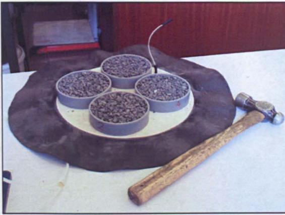
(a) Test material contained in circular rings and compacted by tapping lightly with a hammer placed directly on the 3-bar ceramic disc.
