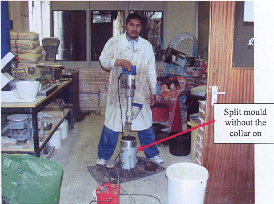
Plate 4.2 Hammer held vertically and vibrated under its own weight as a standard compaction procedure for the triaxial test specimens.
