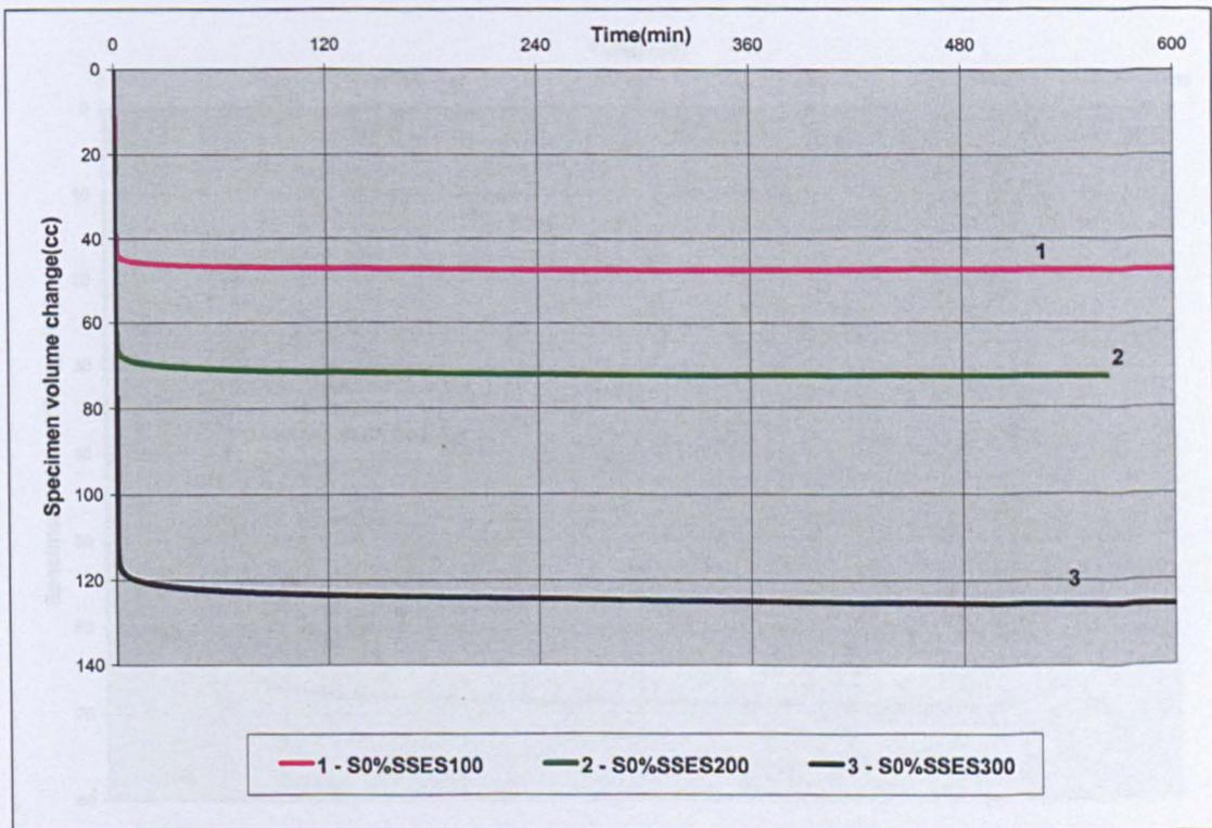
Figure 5.6 Consolidation curves for specimens prepared with loose poured dry soil (Test series B).
