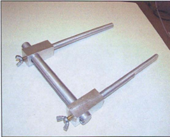
(a) Gauge calliper used to measure specimen diameter.
