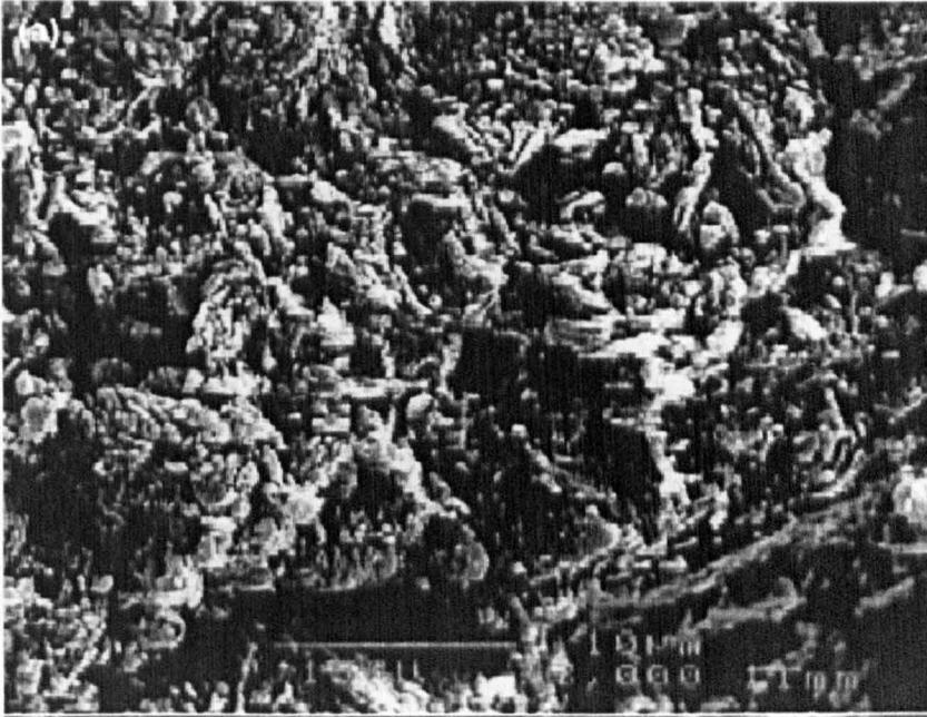
Figure 2.17 Electron micrographs of kaolin showing void spaces indicated by the dark coloured areas (Penumadu and Dean, 2000).
