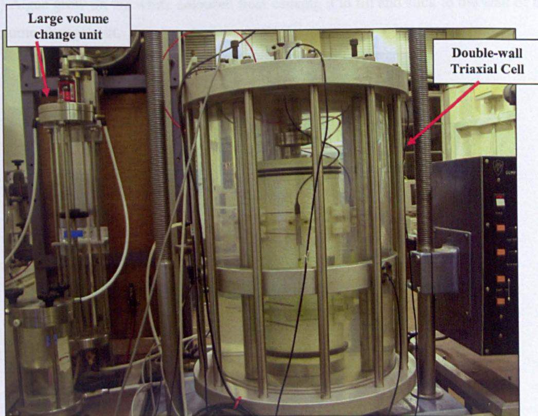
Plate 4.6 Double-walled triaxial cell for testing unsaturated coarse grain soil (Salman, 1995) and the large volume change unit (Fair, 2004) connected to the inner cell to measure specimen volume change during testing.
