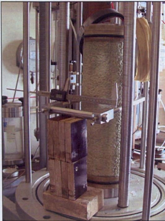
(b) Measuring the mid height specimen diameter using the fabricated gauge calliper with the aid of the electronic vernier scale ruler.
