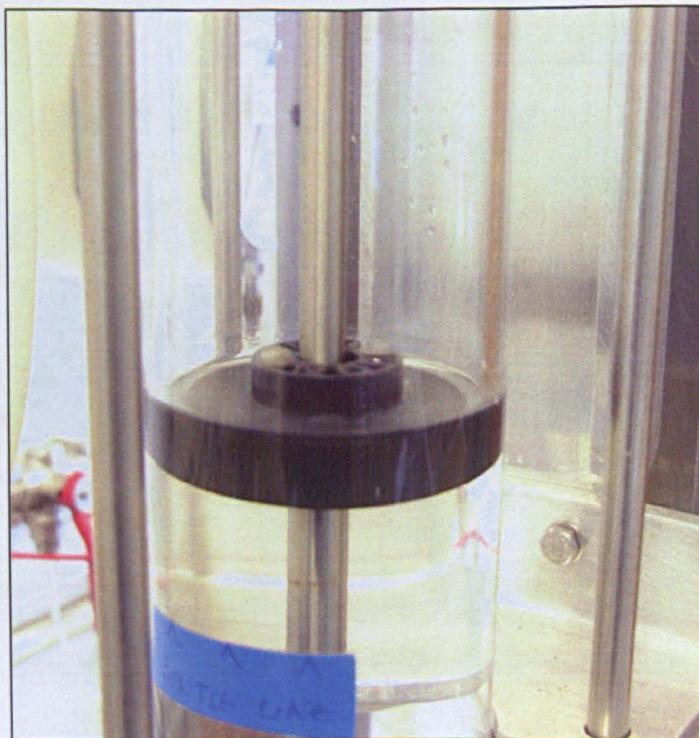
(b) New improved dark coloured hollow float of smaller diameter.
