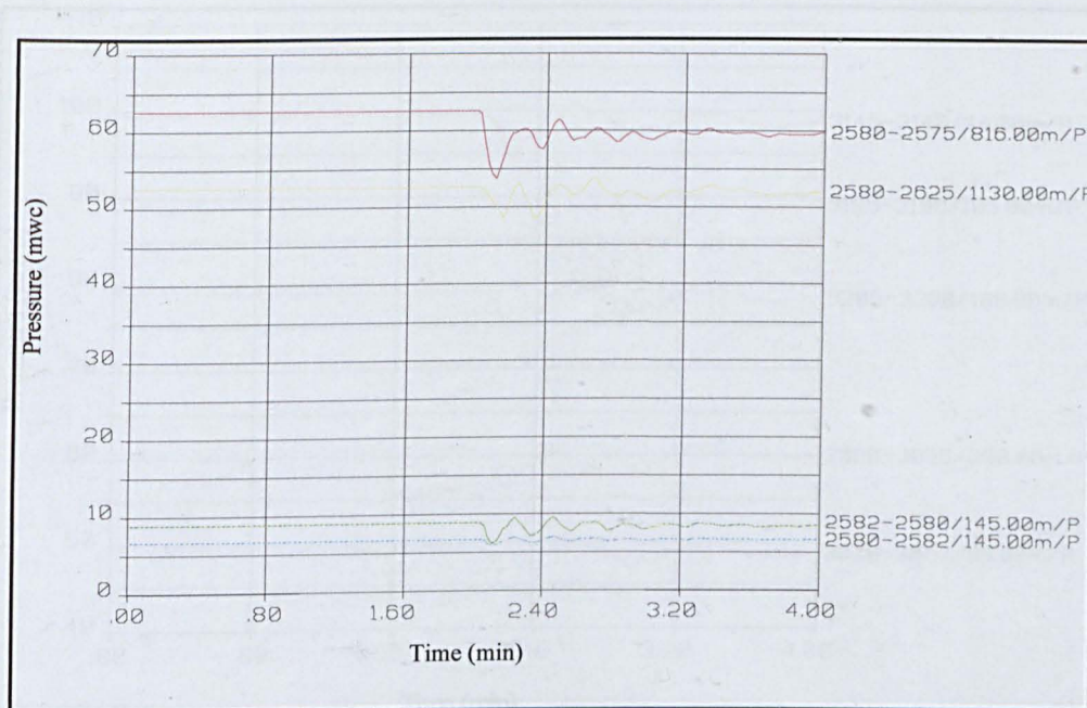
Figure 6.12 Pump switch off Area 8
