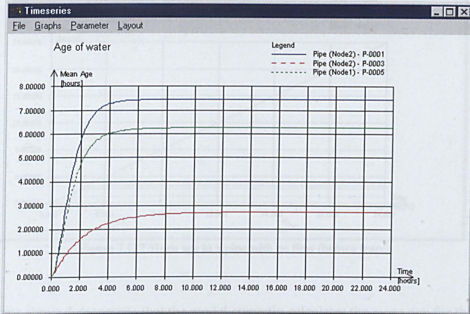
Figure 7.126 Age of 7.45 hours mixes with age of 2.70 hours giving mean age of 6.25 hours
