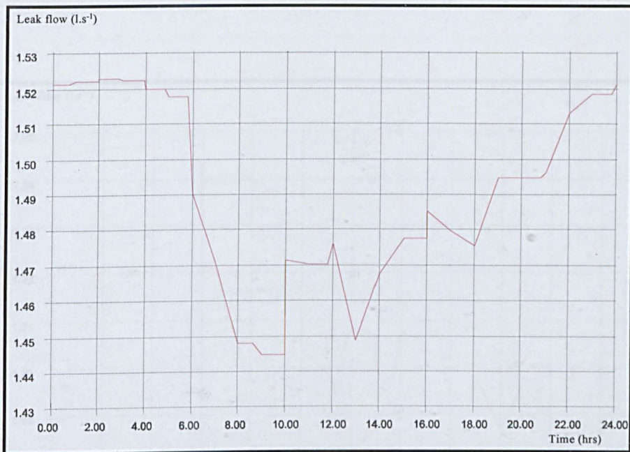
Figure 5.69 Time series of leak flow at node 3147 - Traditional approach
