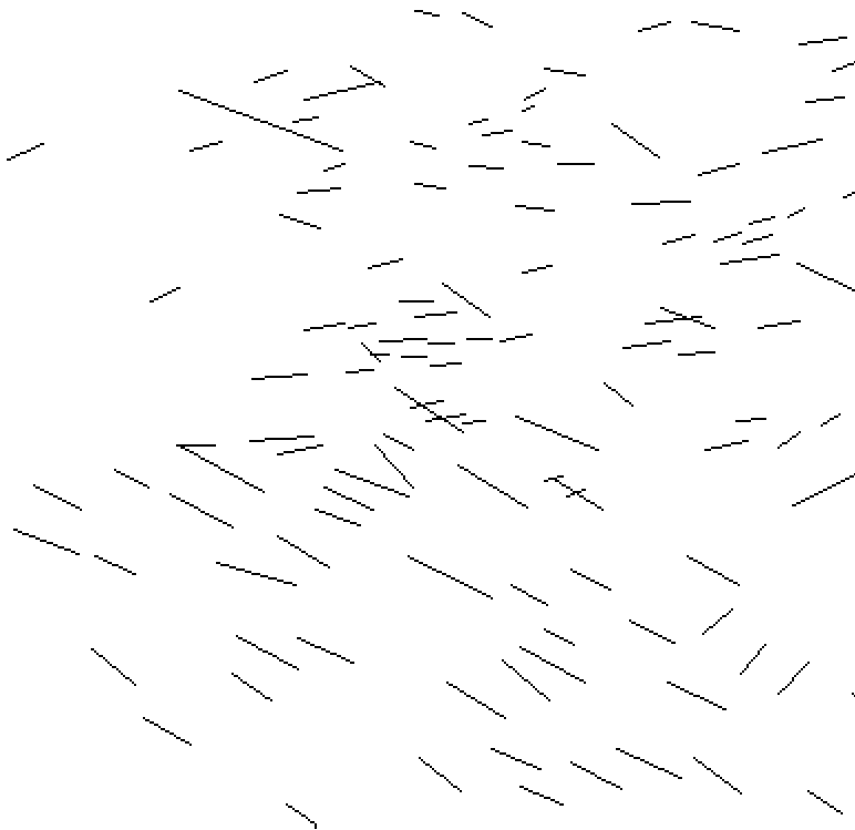
Figure 2.5 a. Example of cross-cutting lineaments depicted on SPOT satellite imagery (Lough Gara, Ireland). The arrows in the top diagram highlight two dominant lineament directions. The circled region shows cross-cutting lineaments. The image is 8.5km across. b. The bottom diagram shows lineaments that have been mapped from the above image.
