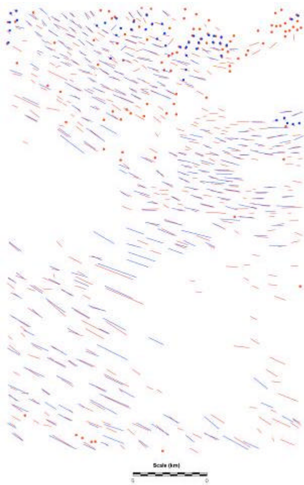
Figure 6.12 a Overlay of lineaments and hillocks mapped from Local Contrast Stretch (blue) and Truth imagery (red).
