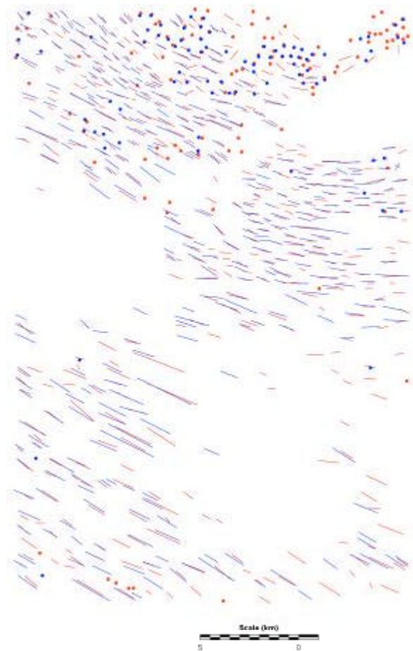
b Overlay of lineaments and hillocks mapped from Curvature (blue) and Truth imagery (red).
