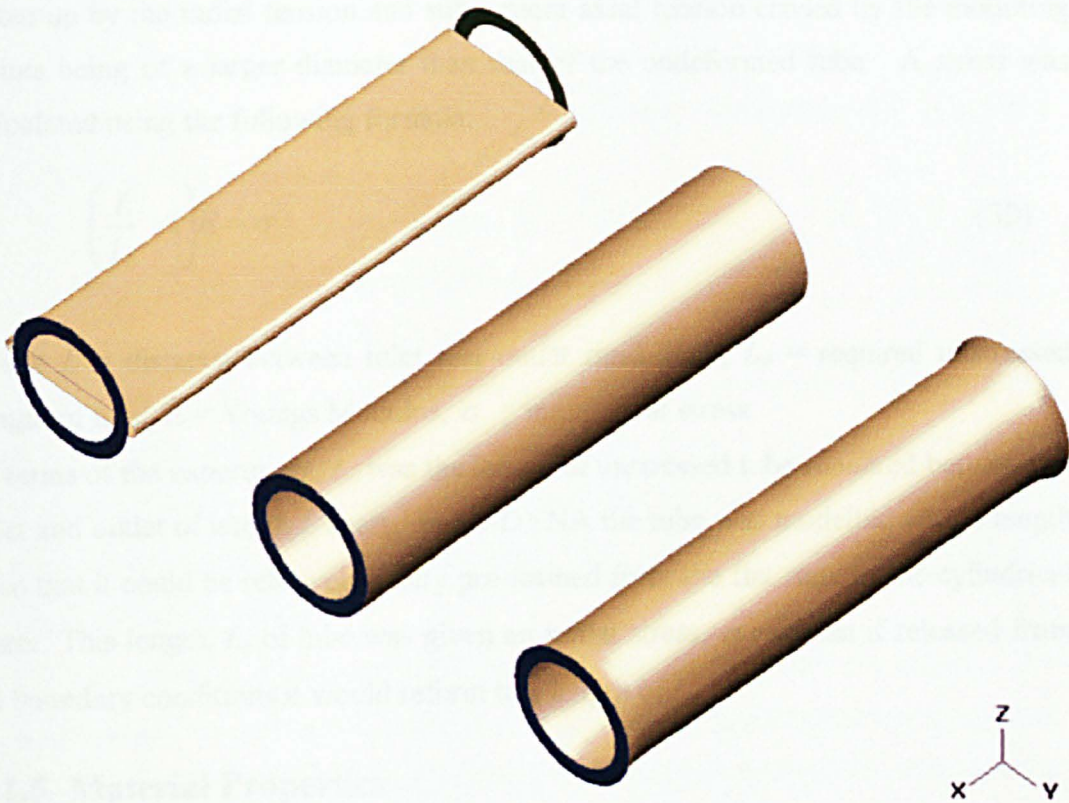
Figure 7.3. Preforming process for the collapsible tube. (a) shows the tube in its undeformed 'flat' state; (b) shows the tube after the nodes have been displaced to the surface of the imaginary circular cylinder; and (c) shows the tube just after the displacement loads were removed.
