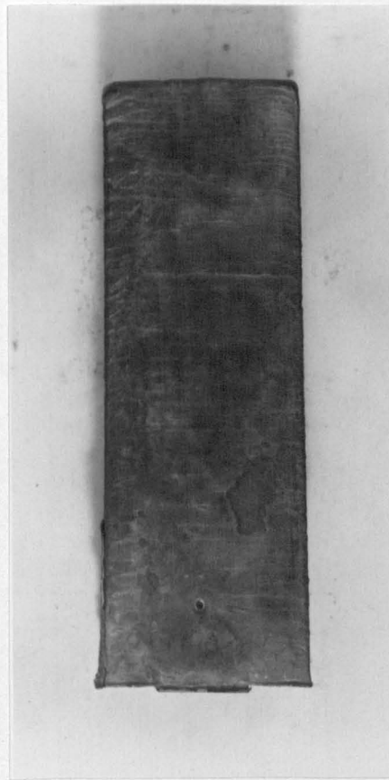
Figure 5.5 Influence of superheat on surface appearance of 18/14-alloys. (a) \Delta T = 10K (Cast 5203) (b) \Delta T = 28K (Cast 5298)
