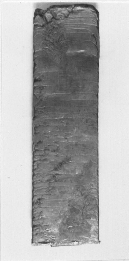
Figure 5.6 Influence of alloy content on surface appearance of fully ferritic grades (17%Cr-alloy, Cast 5275, c.f. Figure 5.1(c)).
