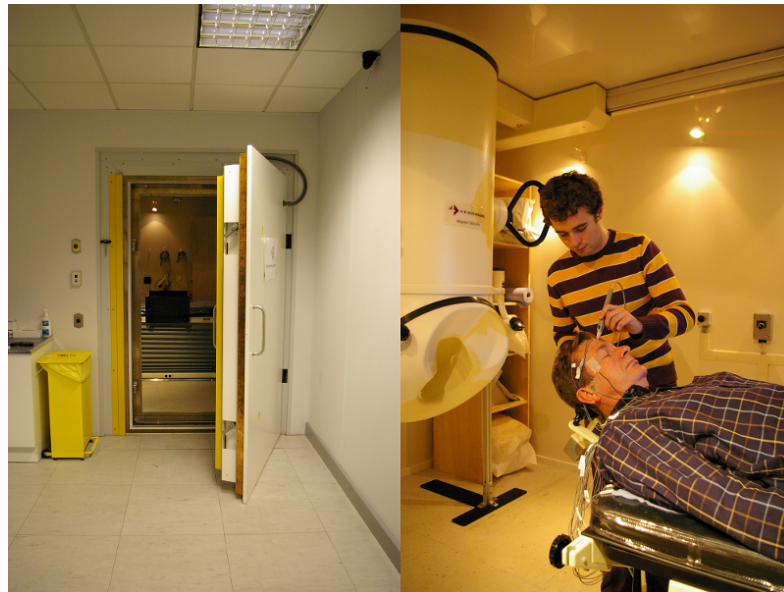
Figure 2.20. An MEG scanner. The left-hand panel shows outer door of the magnetically shielded room containing the scanner. The right-hand panel shows the scanner with a subject (the supervisor) and operator (the author). The cylinder on the left of the picture is the dewar containing the SQUIDS. The operator is marking locations on the subject's head with a Polhemus digitisation system, which provides information on the subject's head shape and position relative to the sensors.
