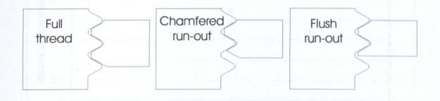
Figure 7.24 Different types of nut thread run-out
