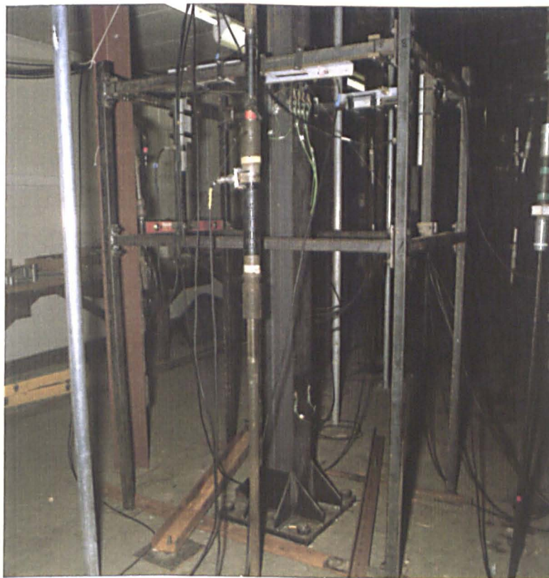
Figure 5.13: Three-dimensional measurement device used to monitor the deformations at the column centre.
