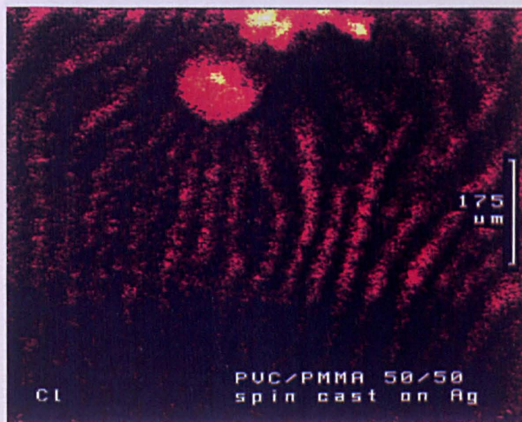
Figure 7.37: ToFSIMS Cl - image for an immiscible PVC/PMMA 50/50 blend spin cast onto Ag
