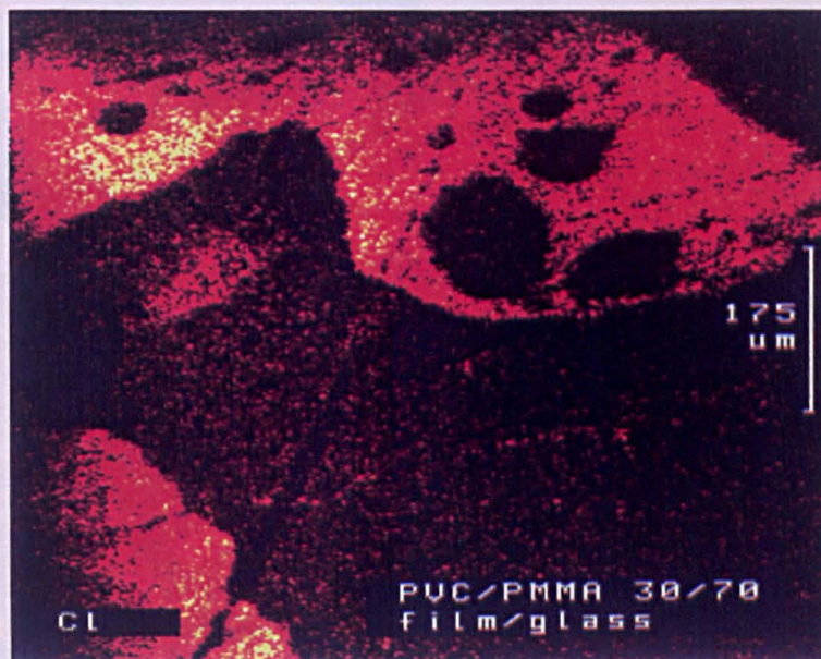
Figure 7.39: ToFSIMS Cl^{-} image for an immiscible PVC/PMMA 30/70 blend analysed at the film/glass interface
