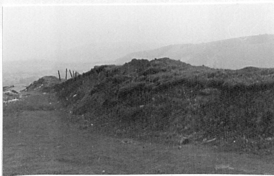
PLATE 3.4 Lifting of the foot of the rotational main unit, Mam Tor.
