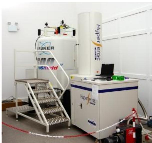
**Figure 2** 600 MHz NMR spectrometer and HyperSense Nuclear polariser.
