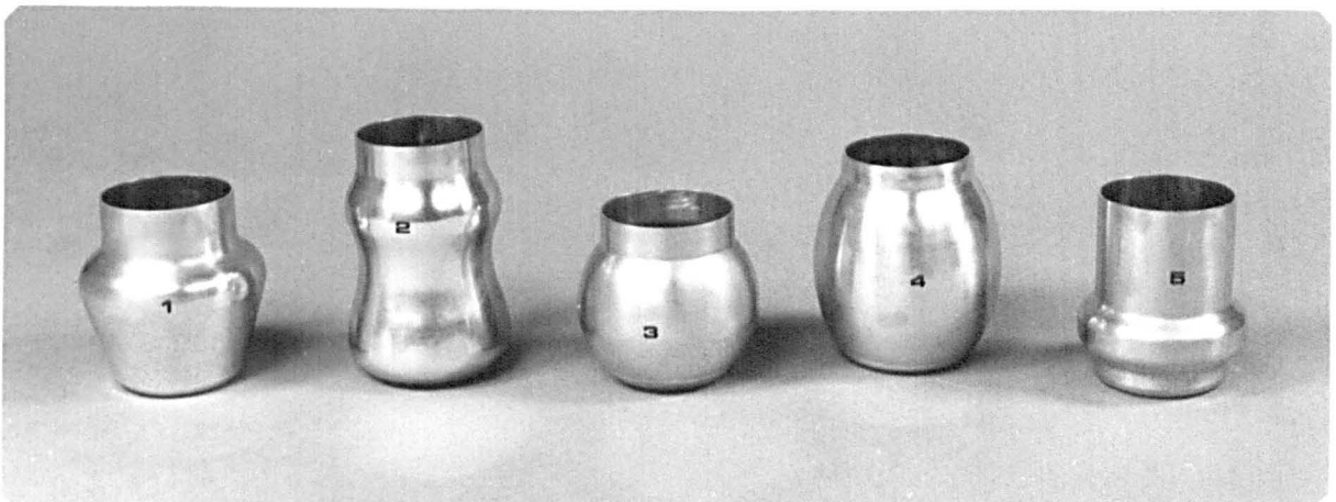
Axisymmetric components produced by hydraulic bulge forming.
