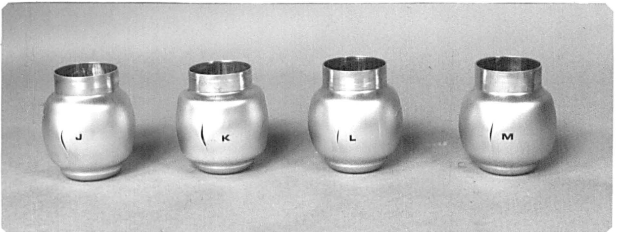
Effect of cup wall thickness on the bulge ratio of annealed cups.
