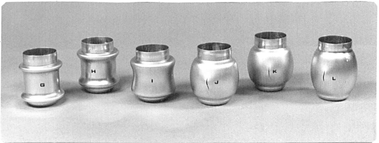
Free bulge forming of annealed cups, typical set of results.
