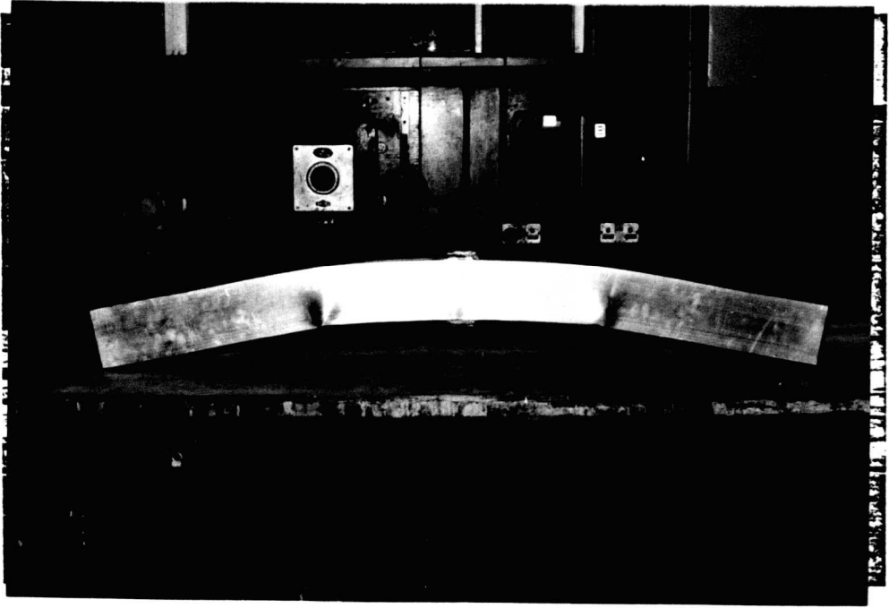
Plate 4.10 Beam Failed in Local Buckling (W-1000-L/2-2)
