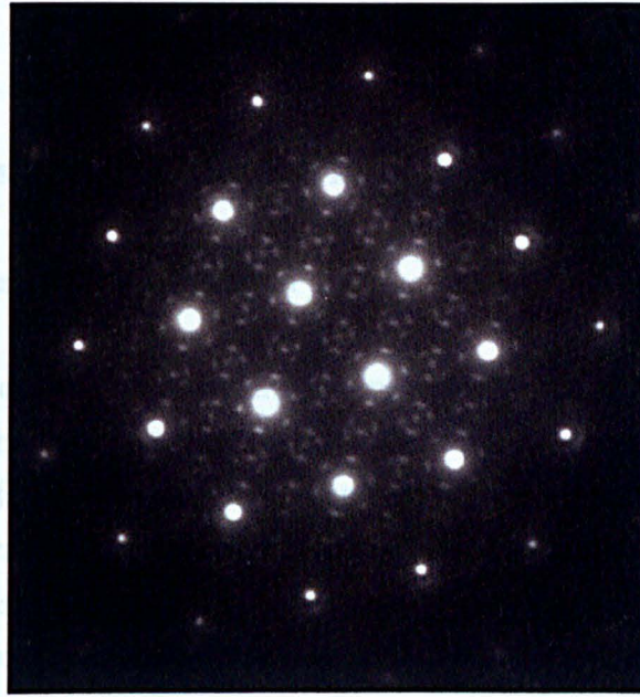
Figure 136 – TEM diffraction pattern along [0001] from a sample aged at 250°C for 12hrs (peak-aged condition). The large spots correspond to the magnesium lattice and the smaller spots correspond to the precipitates
