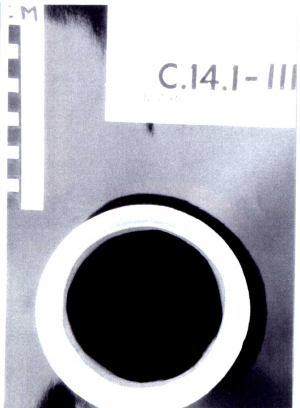
Plate 8.44. Sample C141-C after 12 months weathering.
