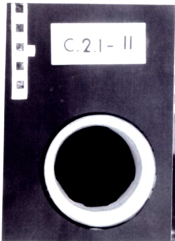
Plate 8.9. Sample C21-N after 6 months weathering.
