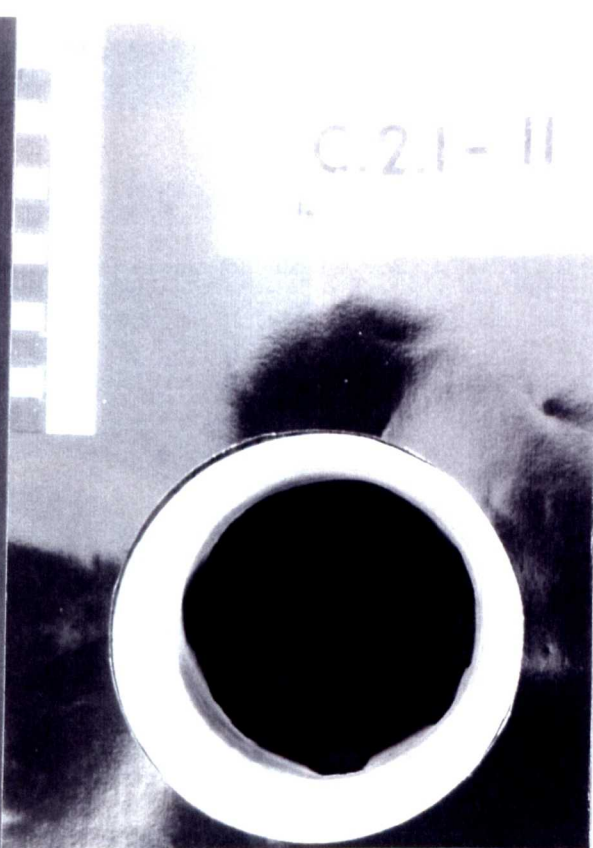
Plate 8.10. Sample C21-N after 12 months weathering.
