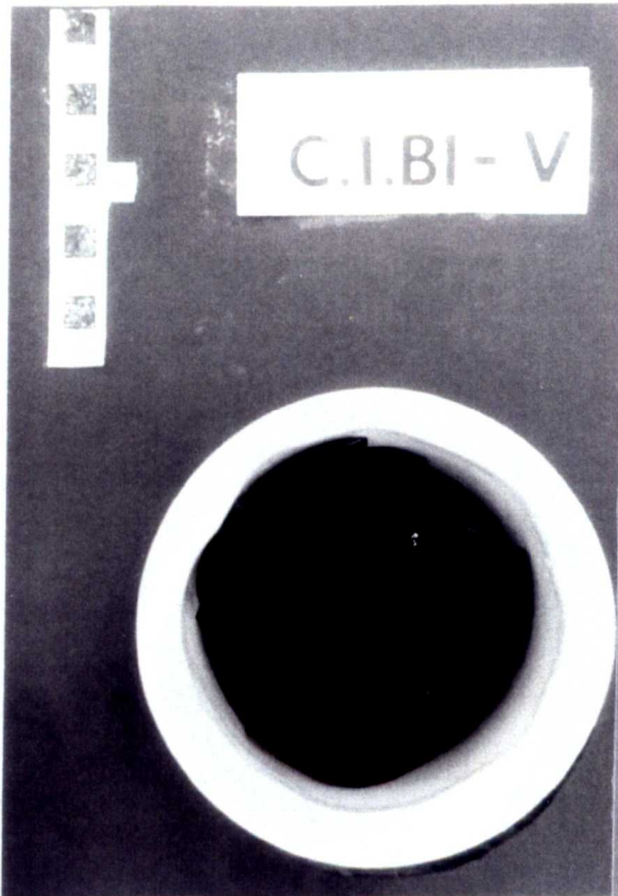
Plate 8.4. Sample CIBI-E after 6 months weathering.
