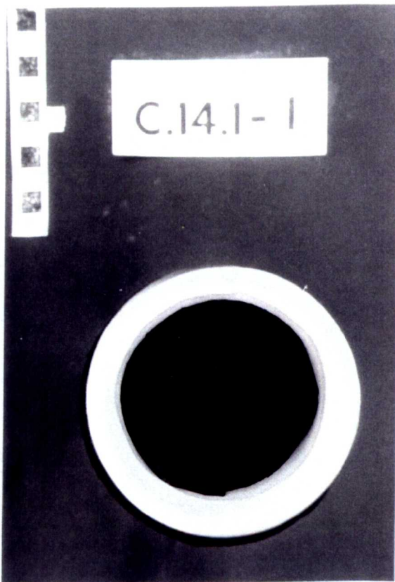
Plate 8.39. Sample C141-H after 6 months weathering.
