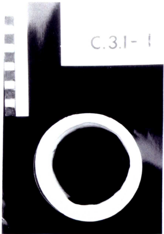
Plate 8.17. Sample C31-H after 12 months weathering.
