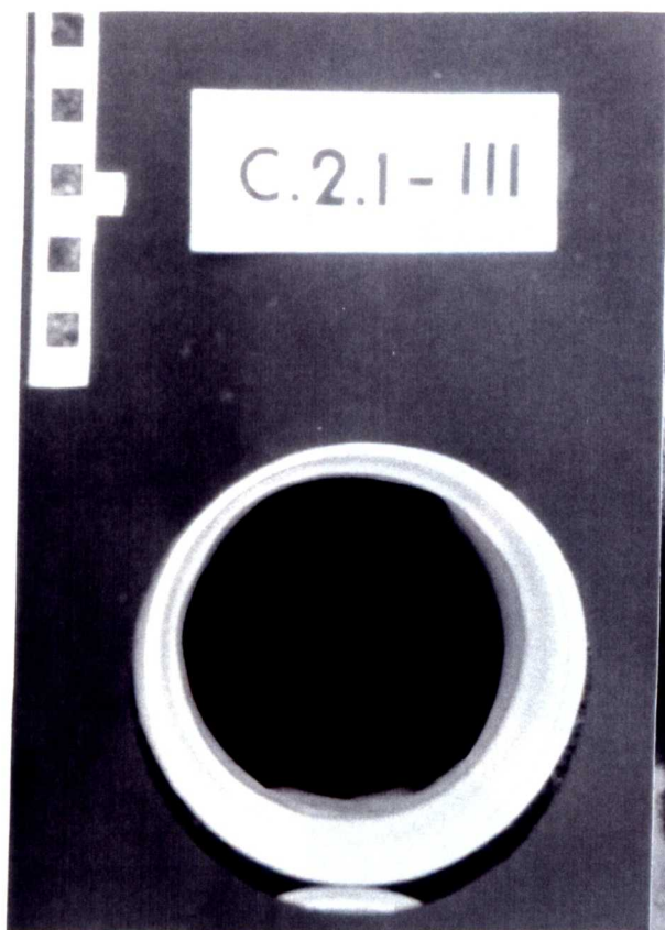
Plate 8.11. Sample C21-C after 6 months weathering.
