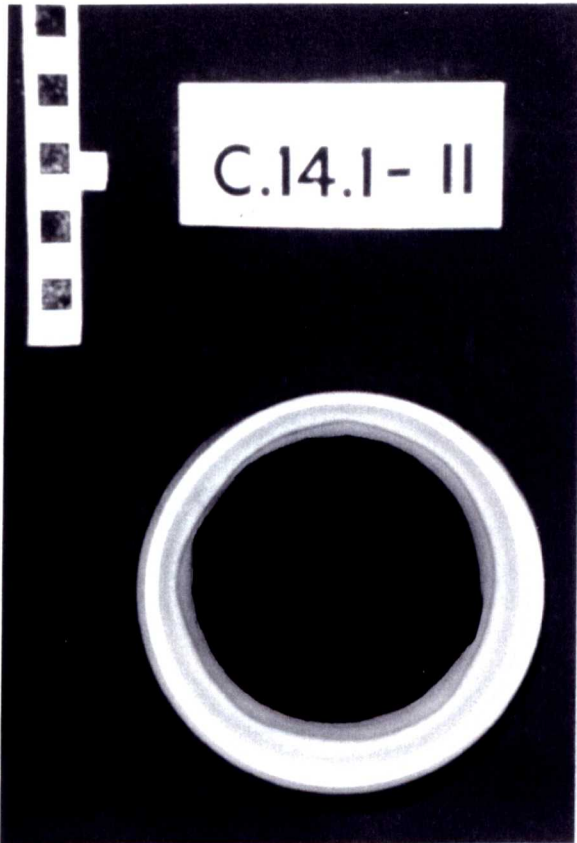
Plate 8.41. Sample C141-N after 6 months weathering.
