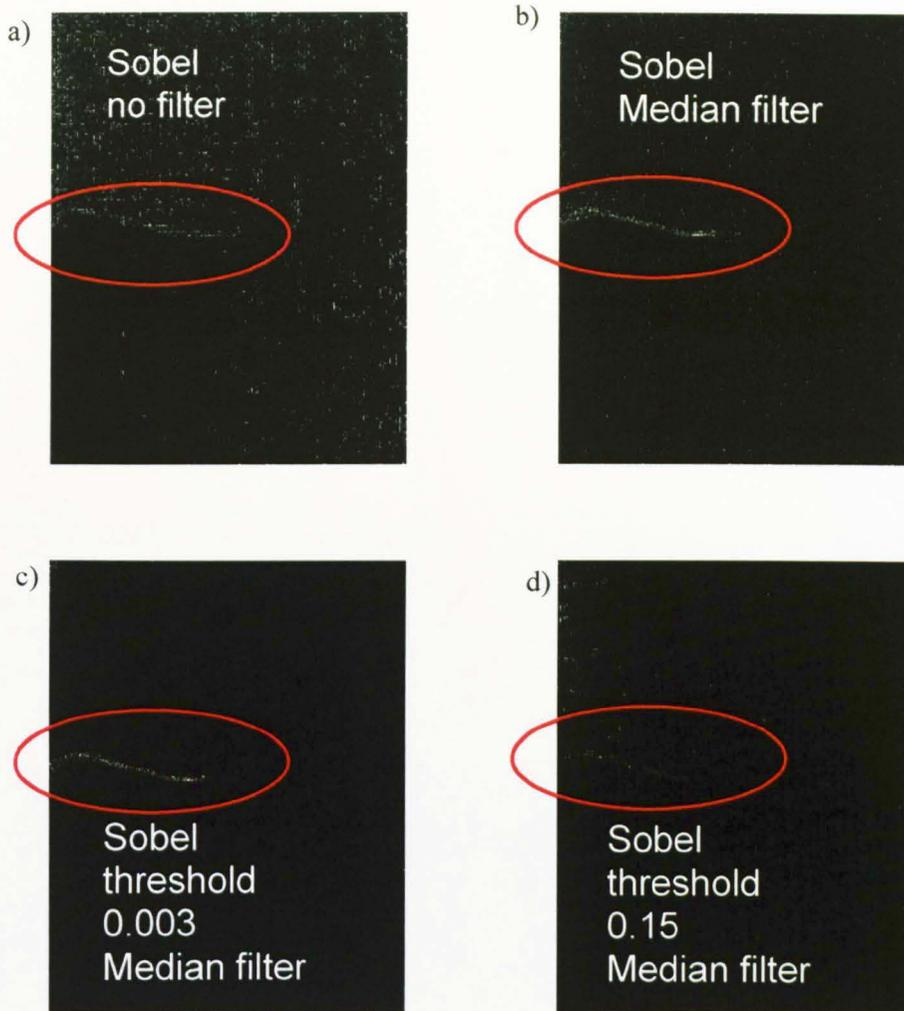
**Figure 5-13** Effects of filtering and threshold value on crack length a) no filter b) Median filter c) Median filter and 0.003 as the threshold value d) Median filter and 0.15 as the threshold value
