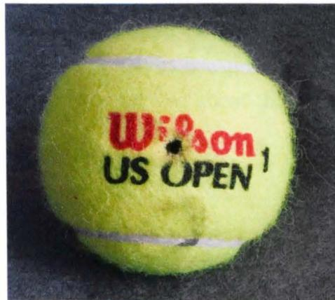
**Figure 6.4** Photograph showing the hole drilled in a tennis ball to test structural stiffness without internal pressure.
