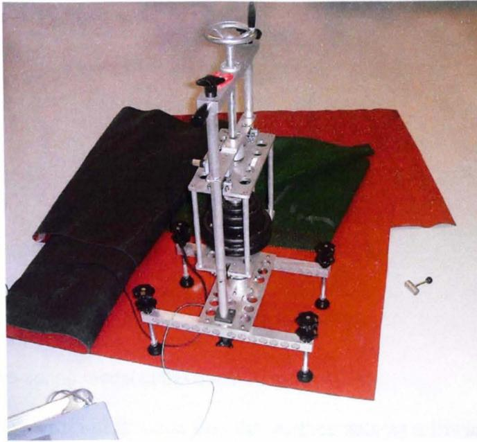
**Figure 5.11** The Berlin Artificial Athlete, used to test shock absorption properties of a surface.
