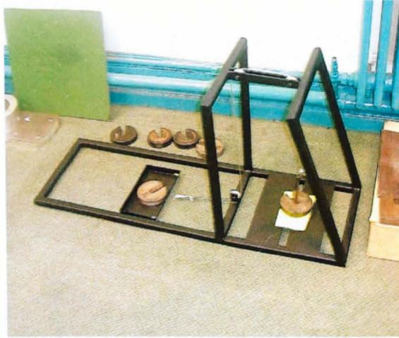
**Figure 5.3** A sled used to measure friction between tennis ball cloth and a surface.
