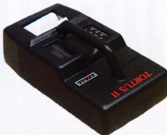
**Figure 5.7** The Tortus friction tester.
