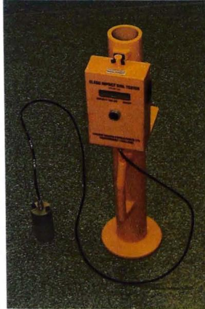
**Figure 5.13** The Clegg Soil Impact Tester, showing the 0.5 kg mass and handset as well as the guide tube
