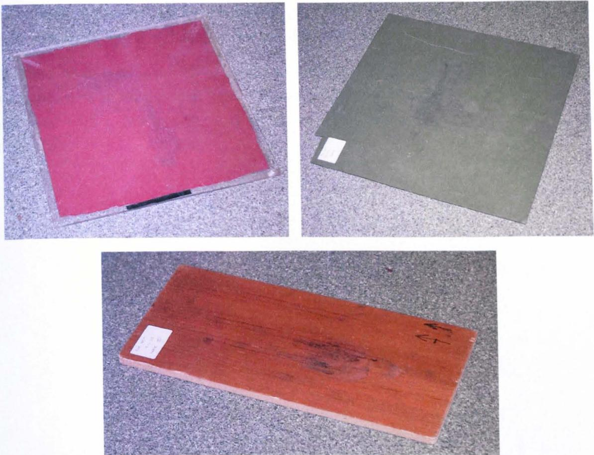
**Figure 9.2** The three surfaces used for the oblique testing: (a) slow acrylic surface (with sand included in the paint), (b) medium acrylic surface and (c) fast wooden surface.
