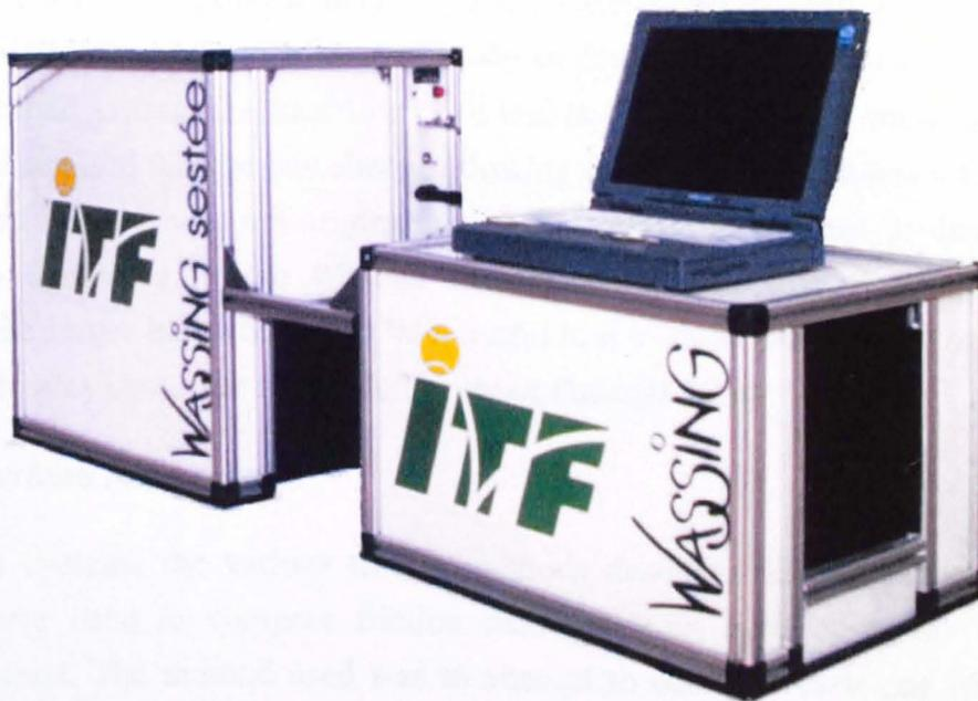
**Figure 5.1** The equipment used to measure surface pace rating.
