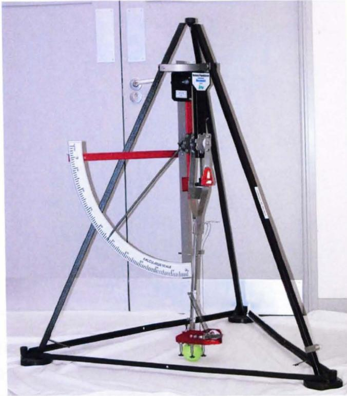
**Figure 5.5** The Haines pendulum for measuring friction, which uses a clamped ball.
