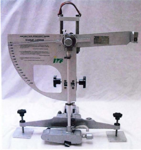
**Figure 5.4** The TRRL pendulum used to measure friction.
