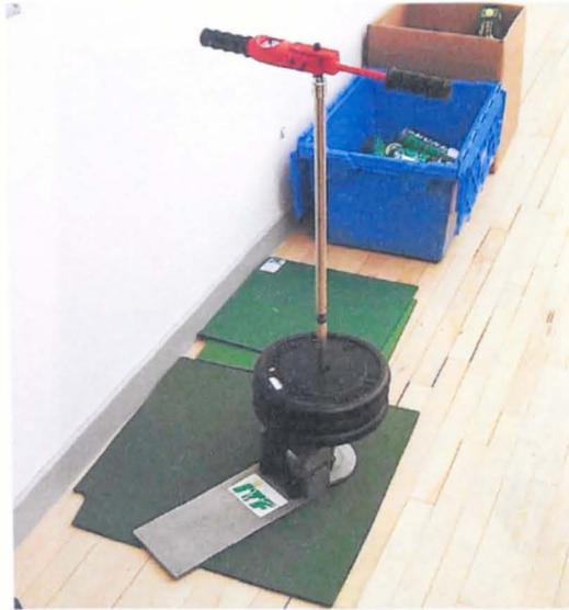
**Figure 5.6** Apparatus used to measure rotational friction.
