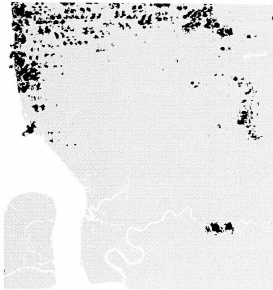
Figure 2.31: The combined cloud and cloud shadow mask for Landsat data from 2 April 1994; cloud and cloud shadow pixels are masked black, while cloud-free, cloud shadow-free and water body pixels are masked grey and white respectively.
