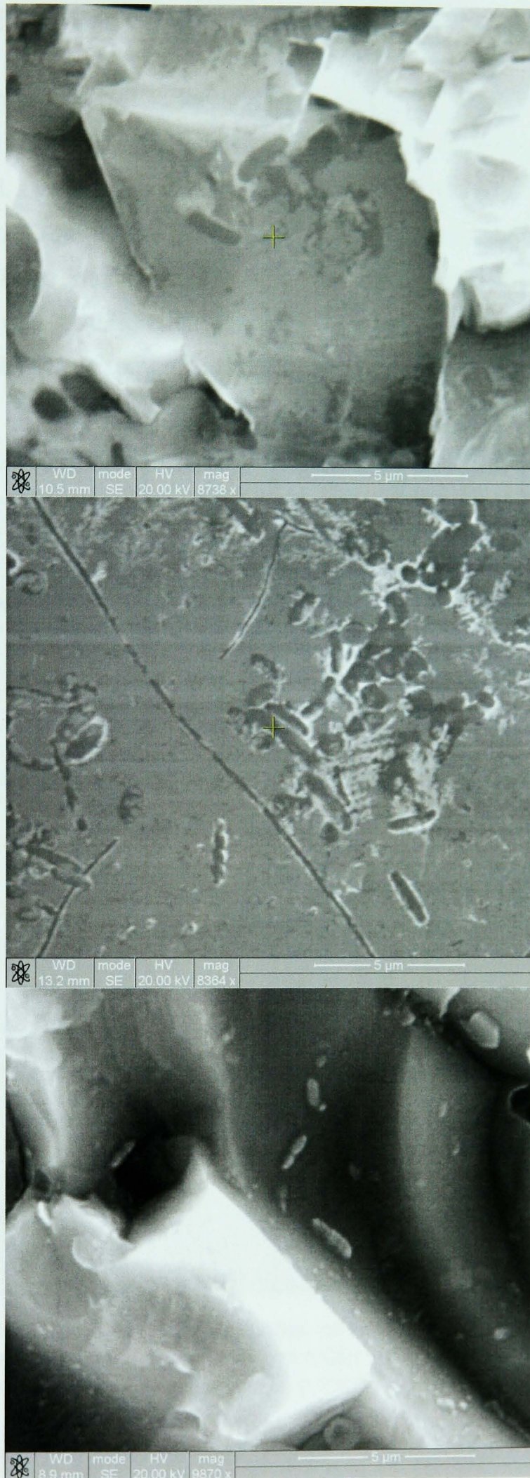
Figure 4-24 ESEM micrographs of microbes attached to orthoclase (top), apatite (centre) and Shap granite.
