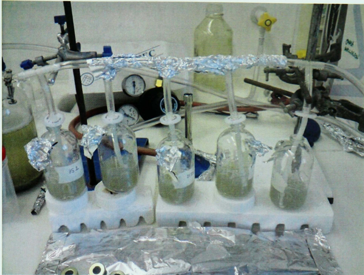
Figure 3-2 Gas manifold system used to degas media prior to cultivation. This method was an adaptation of the method used by Miller and Molin (1974).
