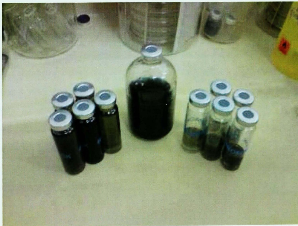
Figure 3-18 MPN cultivation of SRB showing black FeS precipitate characteristic of bacterial sulphate-reduction
