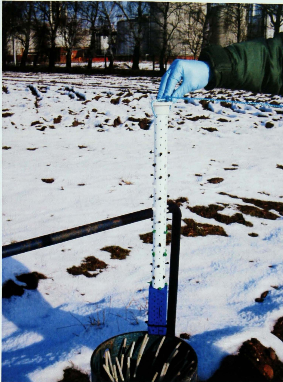
Figure 4-6 Final construction of vessels used to suspend surrogate substrata in borehole 59 at 30mbgl
