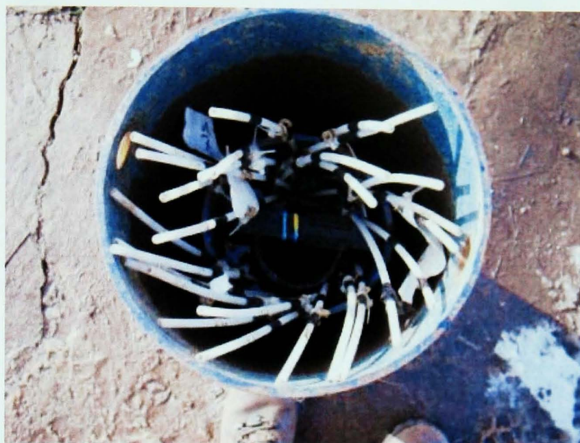
Figure 2-2 Aerial view of borehole 59 showing multiple sample tubes for each level, and inner well-casing, down which the well-screen is located and surrogate minerals were suspended.
