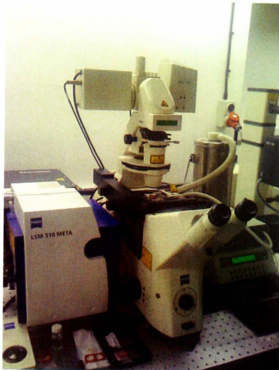
Figure 5.3: A photograph of the inverted confocal microscope, including FCS, used for diffusion measurements.
