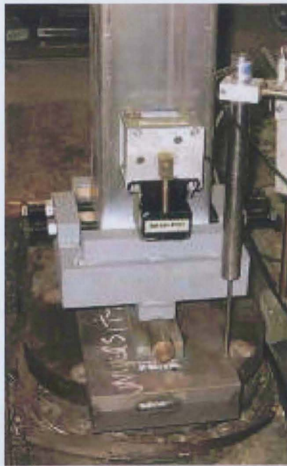
Figure 5.2 Shoe at bottom of test column
