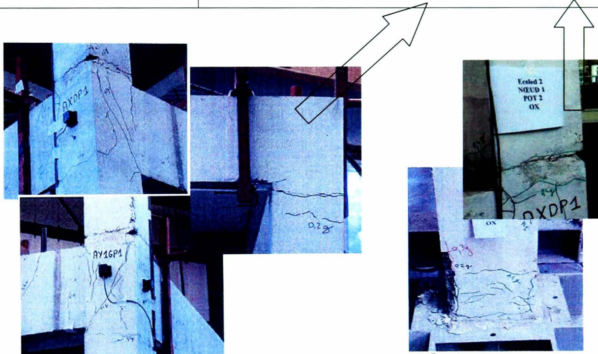
Figure 5.10. Damage at the column-joint interface and column length after the 0.2g and 0.4g tests (Chaudat, 2005).
