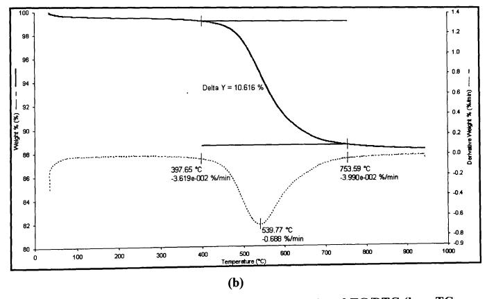
Figure 4.1 - DTA (a; — heating curve, --- cooling curve) and TG/DTG (b; — TG, --- DTG) of kaolin clay.
