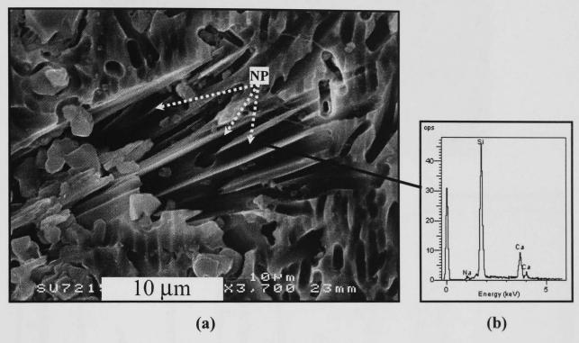
Figure 4.35 - SEM/SE image of cross-sectioned, etched SLS pellets fired 3h at 800°C showing traces of whisker-like wollastonite crystals (a) with their EDS (b). (NP = needle-like features with equiaxial pores)
