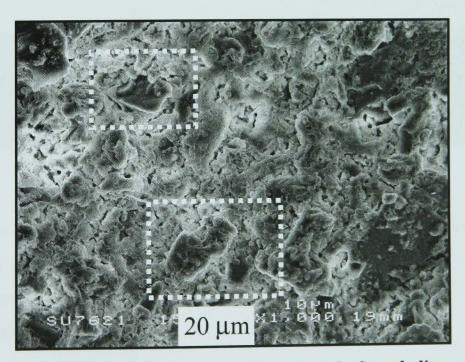
Figure 4.28 - SEM/SE image of a cross-sectioned, etched nepheline syenite pellet fired at 1000°C for 3h.
