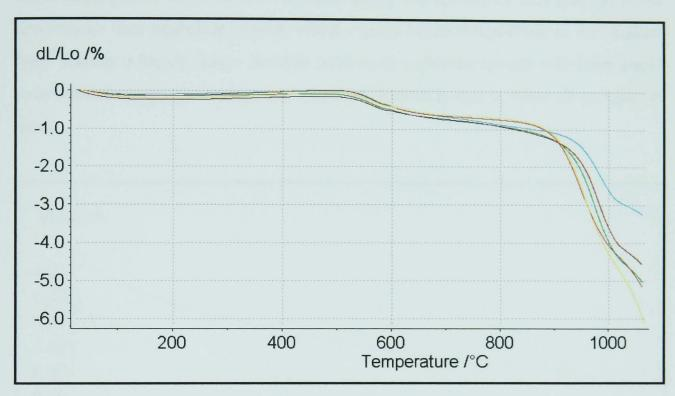
Figure 6.9 - Dilatometric curves of S0, S25, S50, S75 and S100 on heating at 10°C/min from room temperature to 1100°C.
