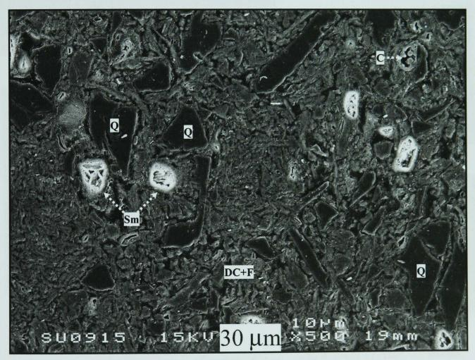
Figure 6.42 - SEM/SE images of polished cross-section of partial SLS-fluxed whiteware (S25) fired at 1000°C. (DC+F = feldspar penetrated clay relicts, Q = quartz, C = cristobalite, Sm = secondary mullite)
