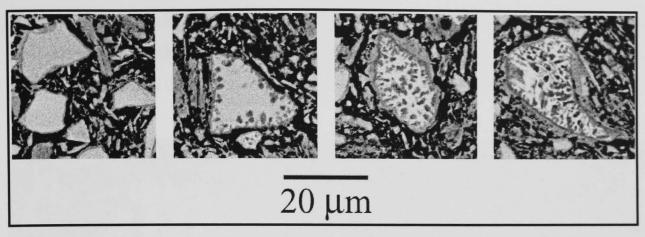
Figure 5.35 - SEM/BS images showing, from left to right, the transformation sequence of SLS glass devitrification in a sample of C-SLS fired at 800°C for 3h.
