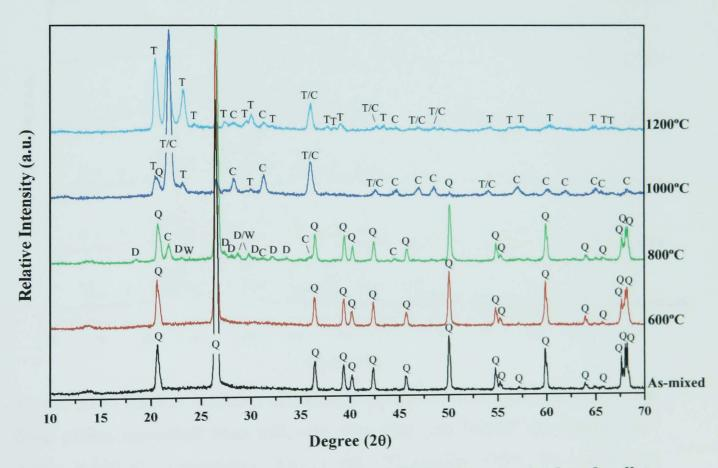
Figure 5.16 - XRD of mixtures of quartz and SLS glass; as-mixed and pellets fired 3h at 600, 800, 1000, and 1200°C and slow cooled are shown (C – Cristobalite, 82-512/39-1425, D – Devitrite, 77-410, Q –  $\alpha$ -quartz, 46-1045, T – Tridymite, 18-1170, W –  $\beta$ -wollastonite, 27-88).
