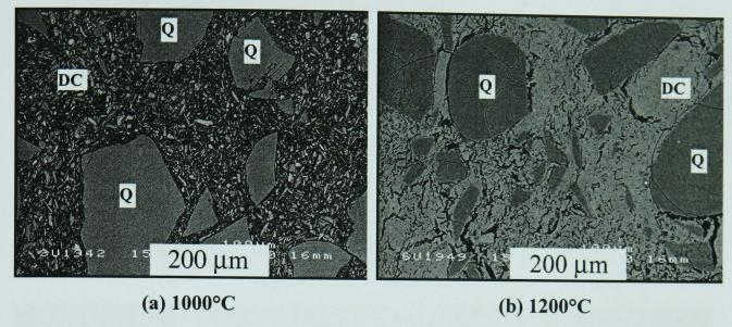
Figure 5.19 - SEM/BS images of cross-sectioned, polished C-Q pellets fired 3h at 1000°C (a) and 1200°C (b). (DC = decomposed clay, Q = quartz)
