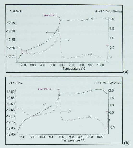
Figure 6.14 - Dilatometric curves (in detail) of S75 (a) and S100 (b) on cooling at 10°C/min from 1100°C to room temperature.
