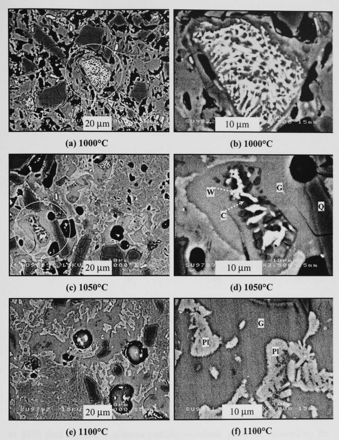
Figure 6.35 - SEM/BS images of polished cross-sections of SLS-fluxed whiteware (S100) fired at 1000, 1050 and  $1100^{\circ}$ C. (Q = quartz, G = glass, C = cristobalite, W = wollastonite, Pl = plagioclase)
