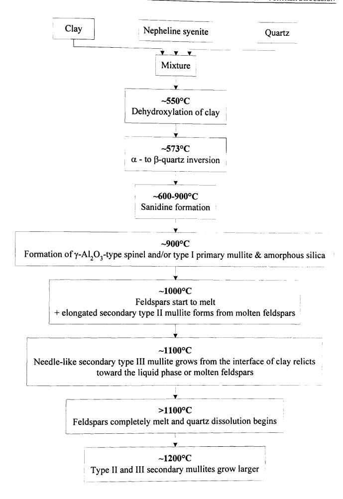
Figure 7.7 - Box diagram of phase evolution on firing standard (nepheline syenite-fluxed) whiteware at 10°C/min.
