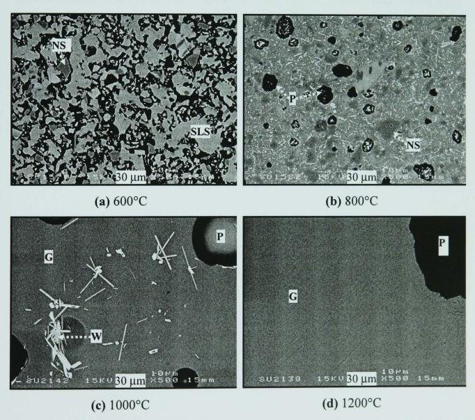
Figure 5.48 - SEM/BS images of cross-sectioned, polished NS-SLS pellets fired 3h at 600°C (a), 800°C (b), 1000°C (c) and 1200°C (d). (G = glassy phase, NS = nepheline syenite, P = pore, SLS = soda-lime-silica glass, W = wollastonite)
