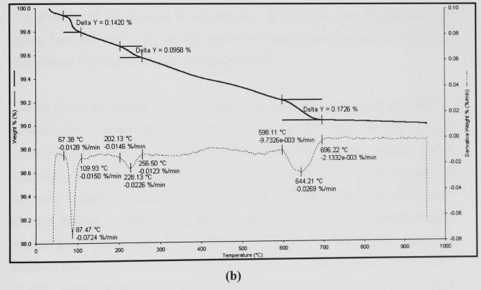
Figure 5.6 - DTA (a; — heating curve, --- cooling curve) and TG/DTG (b; — TG, --- DTG) of the nepheline syenite-SLS glass mixture.
