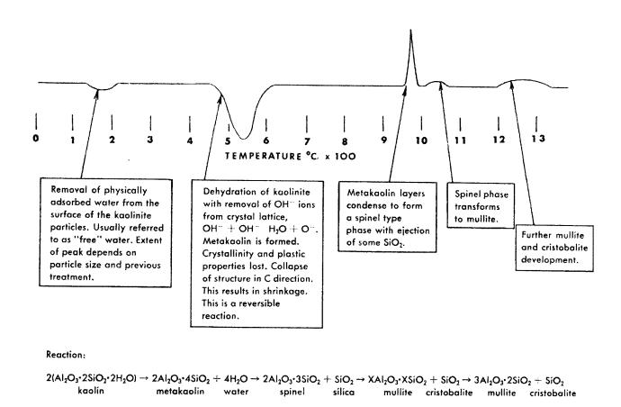
Figure 2.2 - Differential thermal analysis (DTA) curve of kaolinite. (Lawrence, 1972)
