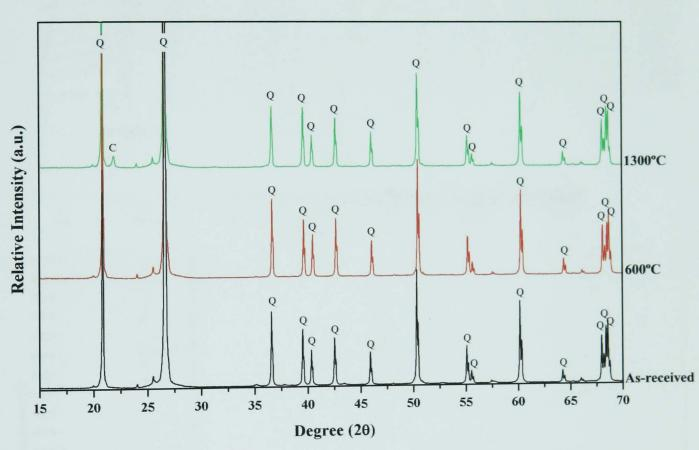
Figure 4.8 - XRD of as-received quartz and of fired quartz pellets quenched at 600 and 1300°C. (C – Cristobalite, 39-1425, Q – α-quartz, 46-1045)
