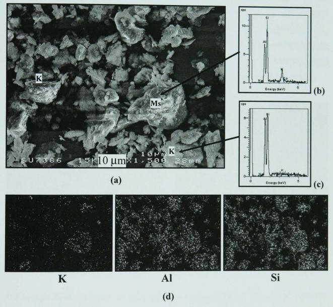
Figure 4.17 - SEM/SE image of the as-received kaolin clay (a). EDS traces of kaolinite (K) and muscovite (Ms) are shown in (b) and (c) respectively. X-ray dot mapping is shown in (d), where the brighter regions are higher in the corresponding element.
