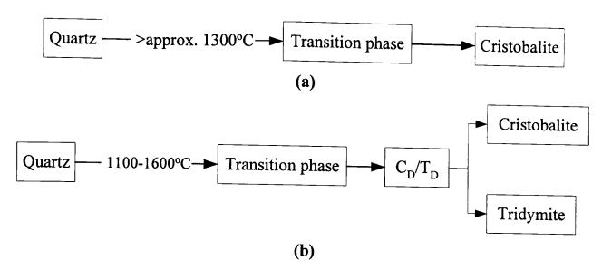
Figure 2.7 - Silica conversions in (a) pure silica system and (b) in the presence of alkali ions. (Stevens et al., 1997)
