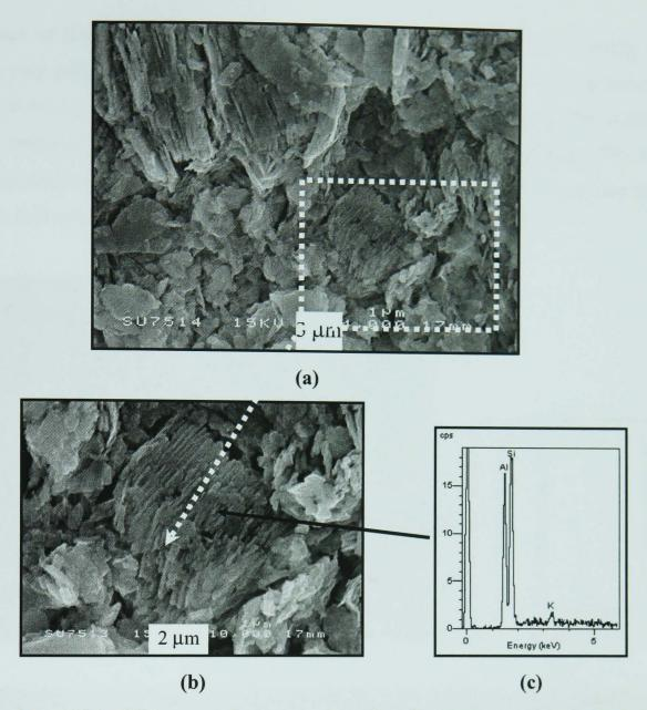
Figure 4.20 - SEM/SE images of cross-sectioned and etched samples made from kaolin clay pellets fired 3h at 800°C (a) and of a selected area at high magnification (b). (c) is EDS of metakaolin platelets shown in (b).
