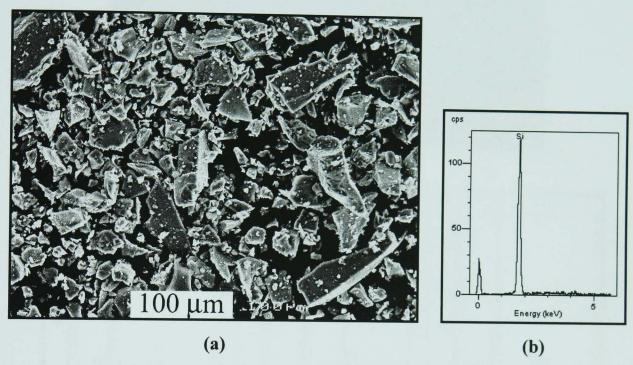
Figure 4.25 - SEM/SE image of the as-received Loch Aline quartz sand (a) and EDS of quartz (b).
