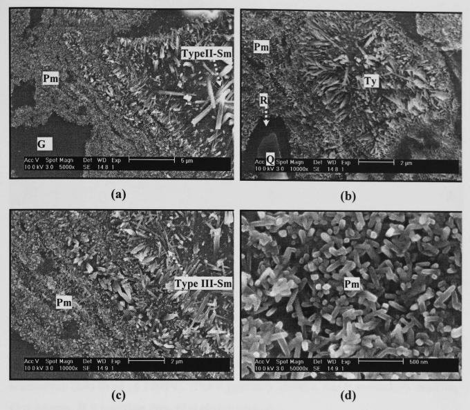
Figure 6.28 - SEM/SE images of polished and etched cross-section of S0 fired at  $1100^{\circ}$ C. (Pm = primary mullite, Sm = secondary mullite, Q = quartz, R = solution rim, G = glassy phase)
