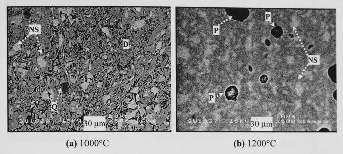
Figure 5.26 - SEM/BS images of cross-sectioned, polished C-NS pellets fired 3h at 1000°C (a), and 1200°C (b). (DC = decomposed clay, NS = nepheline syenite, P = pore, Q = quartz)
