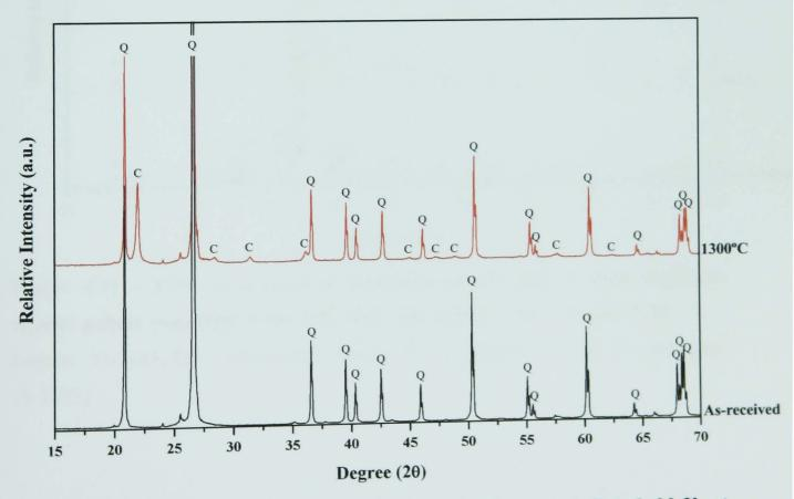
Figure 4.10 - XRD of as-received quartz and of fired quartz pellets held 3h at 1300°C and slowly cooled. (C – Cristobalite, 39-1425, Q – α-quartz, 46-1045)
