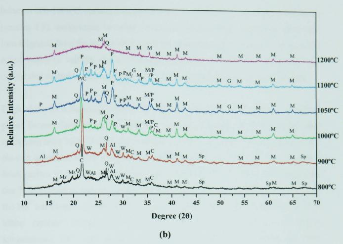
Figure 5.11 - (b) XRD of mixtures of kaolin clay and SLS glass; as-mixed and fired pellets quenched from 800, 900, 1000, 1050, 1100 and 1200°C. (Al – Albite, 71-1153, C – Cristobalite, 82-512, K – Kaolinite-1A, 14-164, M – Mullite, 15-776, Mi – Microcline, 19-926, Ms – Muscovite-2M#1, 6-263, P – Plagioclase, 20-528, Q –  $\alpha$ -quartz, 46-1045, Sp –  $\gamma$ -alumina spinel, 10-425, W – Wollastonite-2M, 27-88).
