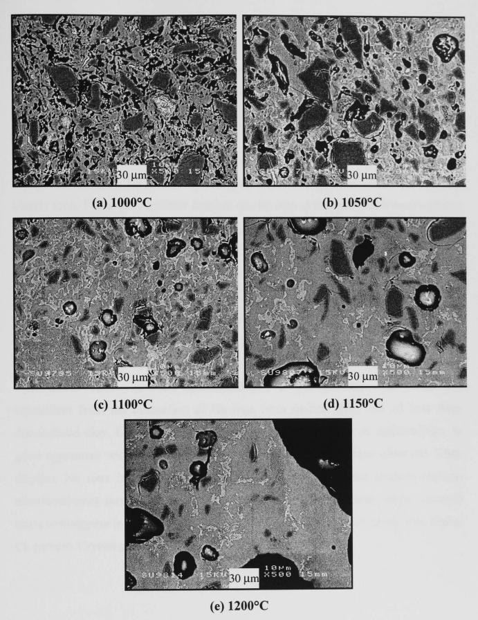
Figure 6.34 - SEM/BS images of polished cross-sections of SLS-fluxed whiteware (S100) fired for 3h at 1000 - 1200°C ((a)-(e), respectively).
