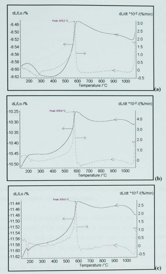
Figure 6.13 - Dilatometric curves (in detail) of S0 (a), S25 (b) and S50 (c) on cooling at 10°C/min from 1100°C to room temperature.
