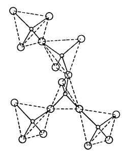
Figure 2.4 - Spiralled chains of SiO<sub>4</sub> in the structure of quartz. (Worrall, 1982)
