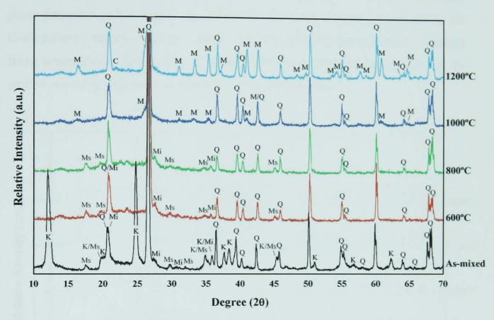
Figure 5.8 - XRD of mixtures of kaolin clay and quartz; as-mixed, fired 3h at 600, 800, 1000, and 1200°C and normally cooled (C – Cristobalite, 82-512, K – Kaolinite-1A, 14-164, M – Mullite, 15-776, Mi – Microcline, 19-926, Ms – Muscovite-2M#1, 6-263,  $\mathbf{Q} - \alpha$ -quartz, 46-1045).
