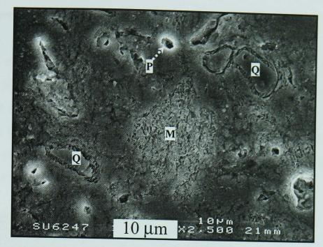
Figure 4.23 - SEM/SE image of a cross-sectioned, polished and etched kaolin clay pellet fired 3h at  $1200^{\circ}$ C. (M = mullite, P = pore, Q = quartz)
