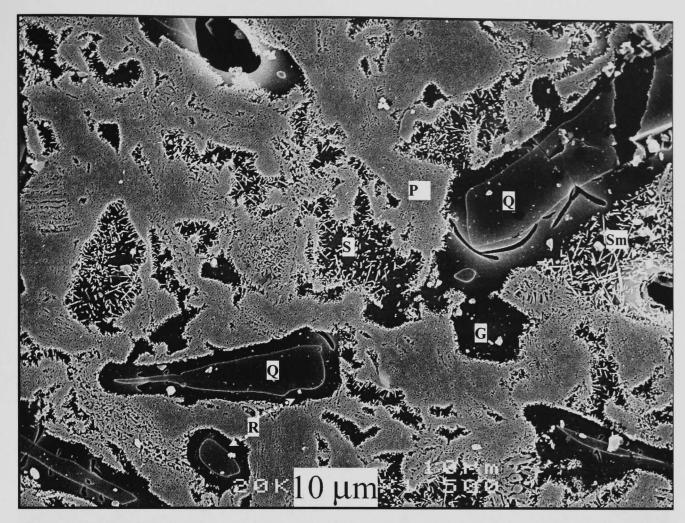
Figure 6.29 - SEM/SE image of polished and etched cross-section of standard whiteware (S0) fired at 1200°C. (Pm = primary mullite, Sm = secondary mullite, Q = quartz, R = solution rim, G = glassy phase)
