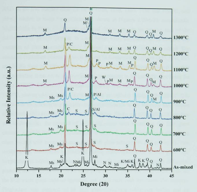
Figure 6.19 - XRD of S75; as-mixed and fired pellets quenched from 600 - 1300°C. (Al – Albite, 71-1153, C – Cristobalite, 82-512, K – Kaolinite-1A, 14-164, M – Mullite, 15-776, Mi – Microcline, 19-926, Ms – Muscovite-2M#1, 6-263, N – Nepheline, 35-424, P – Plagioclase, 20-528, Q – α-quartz, 46-1045, S – Sanidine, 19-1227, W – Wollastonite-2M, 27-88).
