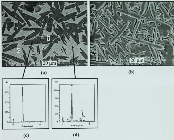
Figure 5.47 - SEM/BS image of a cross-sectioned, unetched (a) and etched sample (b) made from Q-SLS fired 3h at 1200°C. EDS traces of elongated tridymite (T) and glassy phase (G) are shown in (c) and (d), respectively.
