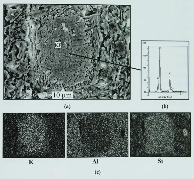
Figure 4.22 - (a) SEM/SE image of cross-sectioned, etched kaolin clay pellet fired at 1000°C showing a K-feldspar particle denoted 'KF' and its EDS (b). EDS element maps are shown in (c), where the brighter regions are high in the corresponding elements.
