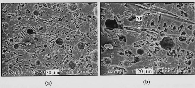
Figure 4.34 - SEM/SE image of cross-sectioned, etched pelletised SLS glass fired 3h at 800°C. (NP = needle-like features with equiaxial pores)
