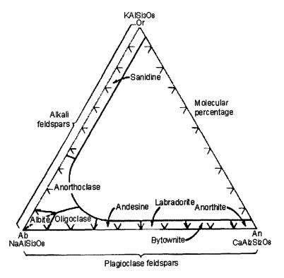
Figure 2.8 - Solid solutions of feldspars. (Deer et al., 1992)
