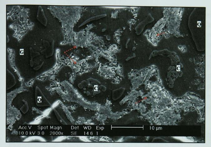
Figure 6.37 - SEM/SE image of SLS-fluxed whiteware (S100) fired at 1100°C. (Q = quartz, C = cristobalite, G = glassy phase)
