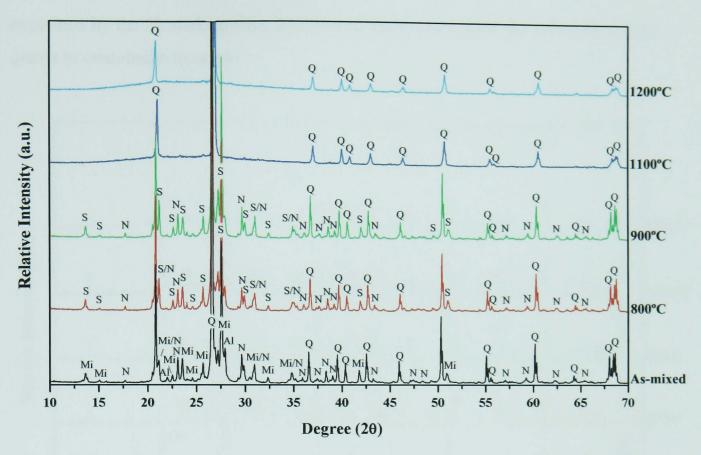
Figure 5.13 - XRD of mixtures of quartz and nepheline syenite; as-mixed and fired pellets quenched from 800, 900, 1100, and 1200°C are shown (Al – Albite, 9-466, C – Cristobalite, 39-1425, Mi – Microcline, 19-932, N – Nepheline, 35-424, S – Sanidine, 19-1227, Q – α-quartz, 46-1045).
