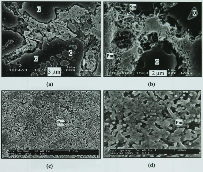
Figure 6.38 - SEM/SE images of SLS-fluxed whiteware (S100) fired at 1100°C, showing clusters of mullite. (Pm = primary mullite, Sm = secondary mullite, Q = quartz, C = cristobalite, G = glassy phase)
