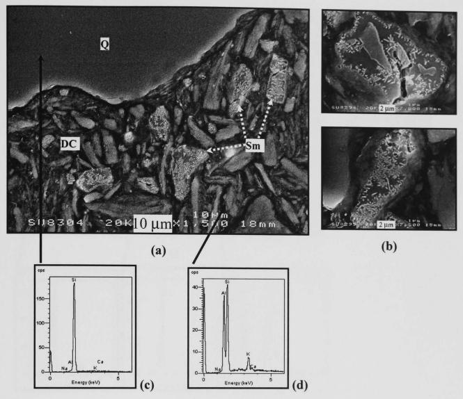
Figure 5.21 - SEM/BS images of a cross-sectioned, etched sample made from C-Q fired 3h at 1000°C (a) and of primary mullite present in this sample (b). EDS traces for quartz and decomposed clay relicts are shown in (c) and (d) respectively. (DC = decomposed clay, Sm = Secondary mullite, Q = quartz)
