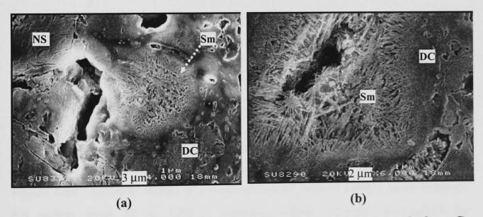
Figure 5.29 - SEM/SE image of a cross-sectioned, etched sample made from C-NS pellets fired 3h at 1000°C (a) and (b). (DC = decomposed clay, NS = nepheline syenite, Sm = secondary mullite)
