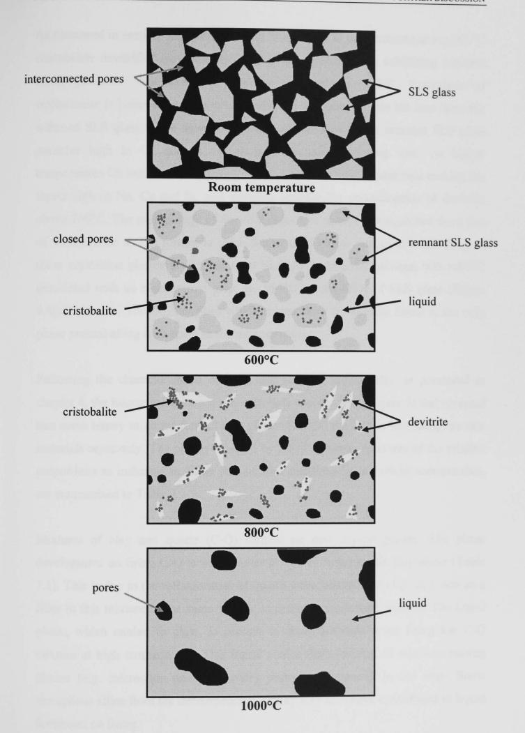
Figure 7.2 - Schematic diagram of the microstructural evolution in SLS glass for firing at 10°C/min.
