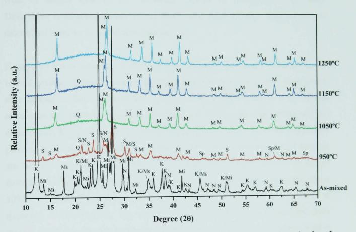
Figure 5.9 - XRD of mixtures of kaolin clay and nepheline syenite. As-mixed and fired pellets quenched from 950, 1050, 1150, and 1250°C are shown (K – Kaolinite-1A, 14-164, M – Mullite, 15-776, Mi – Microcline, 19-926, Ms – Muscovite-2M#1, 6-263, N – Nepheline, 35-424, Q –  $\alpha$ -quartz, 46-1045, S – Sanidine, 19-1227, Sp –  $\gamma$ -alumina spinel, 10-425).
