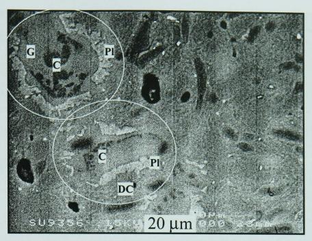
Figure 6.45 - SEM/BS images of polished cross-section of partial SLS-fluxed whiteware (S25) fired at 1100°C showing cristobalite particles (C) embedded in glass (G) which originally consisted of SLS grains, as well as plagioclase (Pl) formed at the outer edges of molten SLS glass in contact with decomposed clay (DC).
