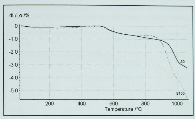
Figure 6.8 - Dilatometric curves of S0 and S100 on heating at 10°C/min from room temperature to 1100°C.
