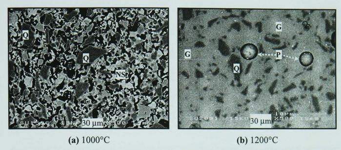
Figure - 5.42 SEM/BS images of cross-sectioned, polished Q-NS pellets fired 3h at 1000°C (a), and 1200°C (b). (G = glassy phase, NS = nepheline syenite, P = pore, Q = quartz)
