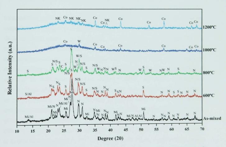
Figure 5.18 - XRD of mixtures of nepheline syenite and SLS glass; as-mixed, and pellets fired 3h at 600, 800, 1000, and 1200°C and slow cooled are shown (Al – Albite, 9-466, C – Cristobalite, 82-512, Co – Corundum, 46-1212, Mi – Microcline, 19-932, N – Nepheline, 35-424, NK – Nepheline, 9-338, S – Sanidine, 19-1227, W – β-wollastonite, 27-88).
