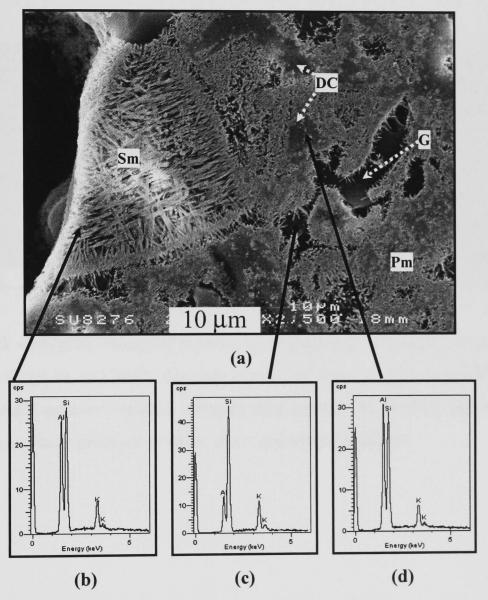
Figure 5.30 - SEM/SE image of a cross-sectioned, etched sample made from C-NS pellets fired 3h at 1200°C showing mullite crystals surrounded by decomposed clay (a). EDS traces of mullite particles, glassy phase and decomposed clay from corresponding areas are shown in (b)-(d). (DC = decomposed clay, G = glassy phase, Pm = primary mullite, Sm = secondary mullite)
