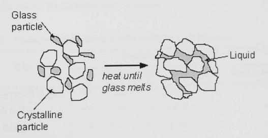
Figure 2.18 - The sintering mechanism of ceramic composites of glass and crystalline compounds
