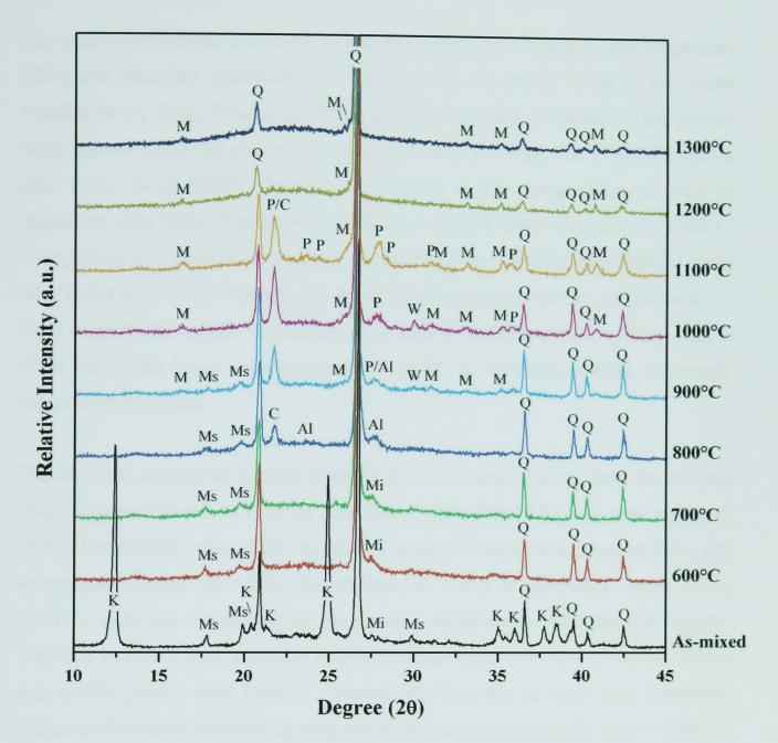
Figure 6.16 - XRD of SLS-based porcelain (S100); as-mixed and fired pellets quenched from 600-1300°C. (Al – Albite, 71-1153, C – Cristobalite, 82-512, K – Kaolinite-1A, 14-164, M – Mullite, 15-776, Mi – Microcline, 19-926, Ms – Muscovite-2M#1, 6-263, P – Plagioclase, 20-528, Q – α-quartz, 46-1045, W – Wollastonite-2M, 27-88).
