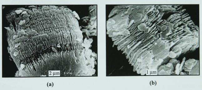
Figure 4.18 - SEM/SE images of as-received kaolin clay show well crystallized stacks of pseudo-hexagonal kaolinite platelets.
