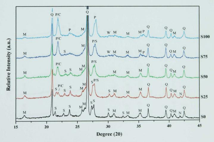
Figure 6.20 - XRD of each batch fired at 1000°C for 3h.
