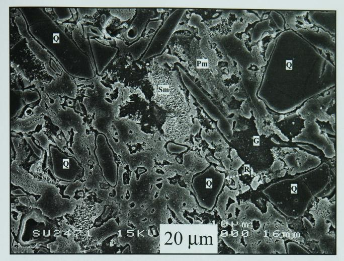
Figure 6.46 - SEM/SE image of polished and etched cross-section of partial SLS-fluxed whiteware (S25) fired at 1100°C. (Pm = primary mullite, Sm = secondary mullite, Q = quartz, G = glassy phase, R = solution rim)
