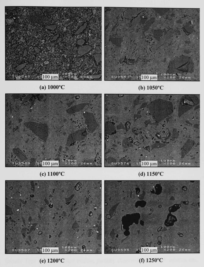
Figure 6.27 - SEM/BS images of polished cross-sections of standard whiteware (S0) fired at 1000 - 1250°C (a)-(f).
