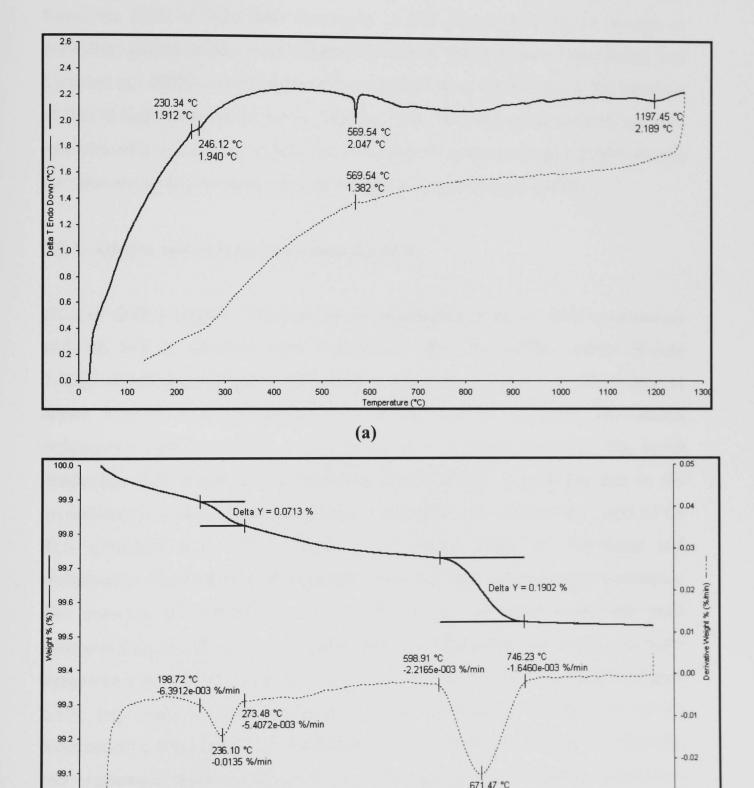
Figure 5.4 - DTA (a; — heating curve, --- cooling curve) and TG/DTG (b; — TG, --- DTG) of quartz-nepheline syenite mixture.
