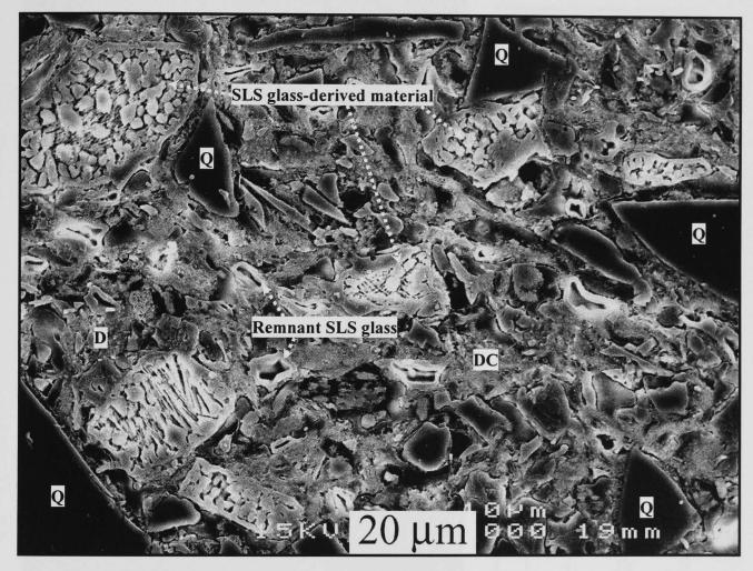
Figure 6.30 - SEM/SE image of polished and etched cross-section of SLS-fluxed whiteware (S100) fired at 1000°C. (DC = decomposed clay, Q = quartz)
