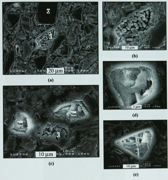
Figure 6.43 - SEM/SE images of polished and etched cross-section of partial SLS-fluxed whiteware (S25) fired at 1000°C showing cristobalite particles (C) devitrified from molten SLS glass particles (b) and elongated secondary (Type II) mullite (Sm) formed from molten feldspar particles ((d) and (e)).
