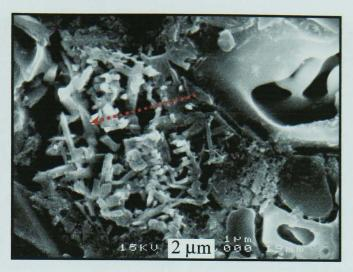
Figure 6.33 - SEM/SE image of polished and etched SLS-fluxed whiteware (S100) fired 3h at 1000°C, showing lath-like plagioclase particles (arrowed).
