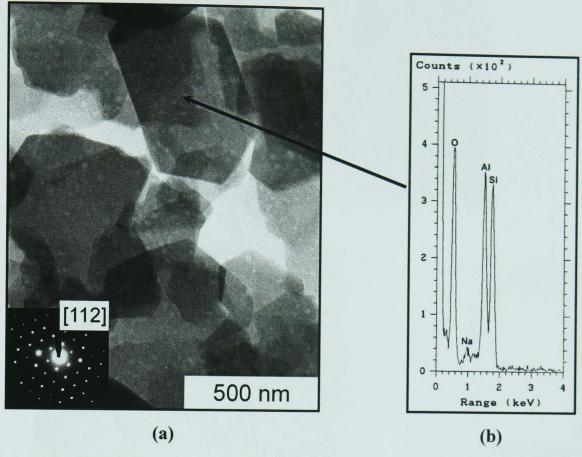
Figure 4.19 - TEM/BF image of kaolinite crystals in the clay (a). Inset in (a) is a [112] zone axis diffraction pattern of a kaolinite crystal. (b) is EDS of kaolinite.
