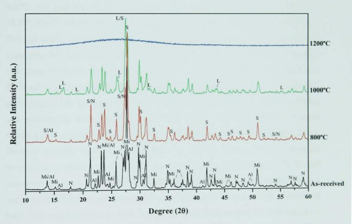
Figure 4.13 - XRD of as-received nepheline syenite and of fired nepheline syenite pellets held for 3h at 800, 1000, 1200°C. (Al – Albite, 9-466, L – Leucite, 85-1419, Mi – Microcline, 19-932, N – Nepheline, 35-424, S – Sanidine, 19-1227).
