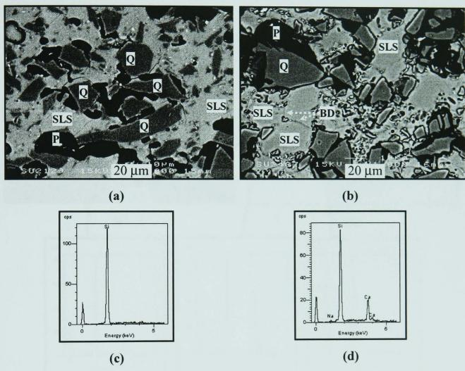
Figure 5.44 - SEM/BS image of a cross-sectioned, unetched (a) and etched samples (b) of Q-SLS fired 3h at 600°C. EDS traces of quartz and SLS glass are shown in (c) and (d). (BD = boundary between particles, P = pore, Q = quartz, SLS = soda-lime-silica glass)
