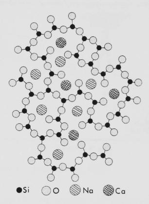
Figure 2.13 - Atomic structure of a soda-lime-silica glass. (Lawrence, 1972)
