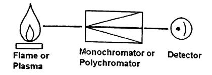
Figure 3.2 - Schematic of Atomic Emission Spectroscopy system. (Boss and Fredeen, 1997)
