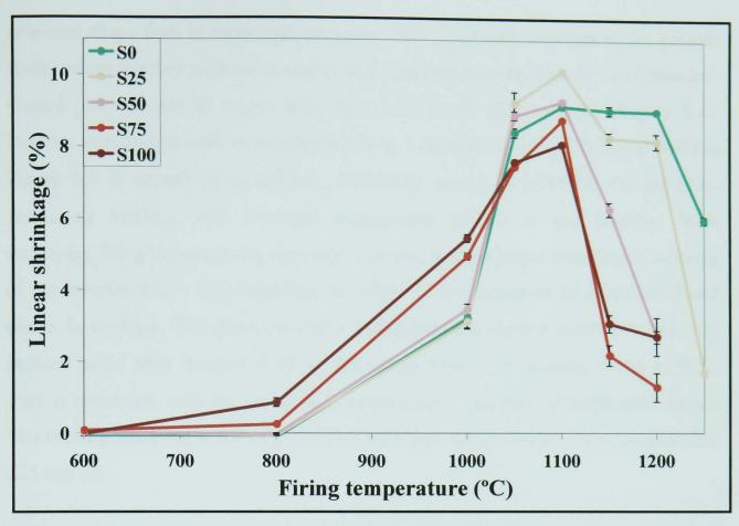
Figure 6.3 - Linear shrinkage of as-fired specimens from all batches. (Heating at 10°C/min, holding time 3h and cooling at 10°C/min).
