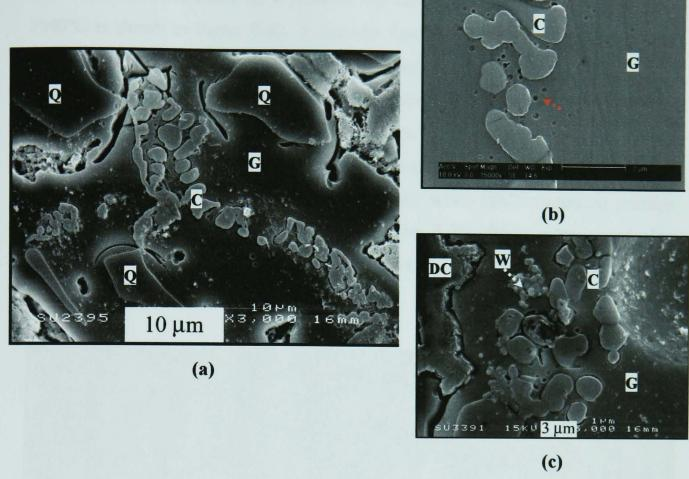
Figure 6.41 - SEM/SE images of SLS-fluxed whiteware (S100) fired at 1100°C showing cristobalite particles embedded in glassy phase. Cristobalite with bubbles and with wollastonite are shown in (b) and (c) respectively. (DC = decomposed clay, Q = quartz, C = cristobalite, W = wollastonite, G = glassy phase)
