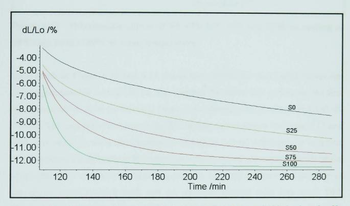
Figure 6.11 - Dilatometric curves of S0, S25, S50, S75 and S100 during the 3h soaking (isotherm) at 1100°C.
