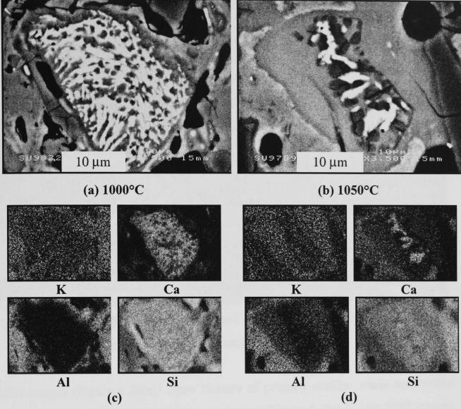
Figure 6.36 - SEM/BS images of polished cross-sections of SLS-fluxed whiteware (S100) showing the change occurring in SLS and its surroundings after firing 3h at 1000°C (a) and 1050°C (b). EDS maps of features in (a) and (b) are shown in (c) and (d) respectively.
