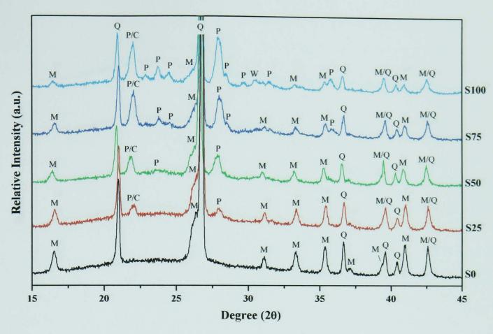
Figure 6.21 - XRD of each batch fired at 1050°C for 3h.
