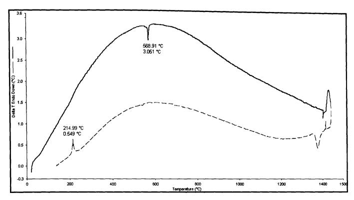
Figure 4.2 - DTA of quartz. (—heating curve, --- cooling curve)
