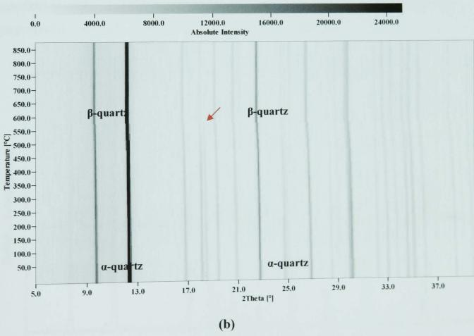
Figure 4.9 - In situ HTXRD of as-received quartz as a function of temperature (a). (b) is a top view perspective of the traces in (a), showing higher peak intensities with darker shades. (Red arrow shows the disappearance of 18.4° α-quartz peak).
