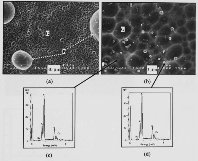
Figure 4.32 - SEM/SE image of cross-sectioned, etched nepheline syenite pellets fired 3h at 1200°C (a), and area at high magnification (b). (c) is EDS from glassy phase, and (d) is EDS of rounded crystals shown in (b). (G = glassy phase, P = pore)
