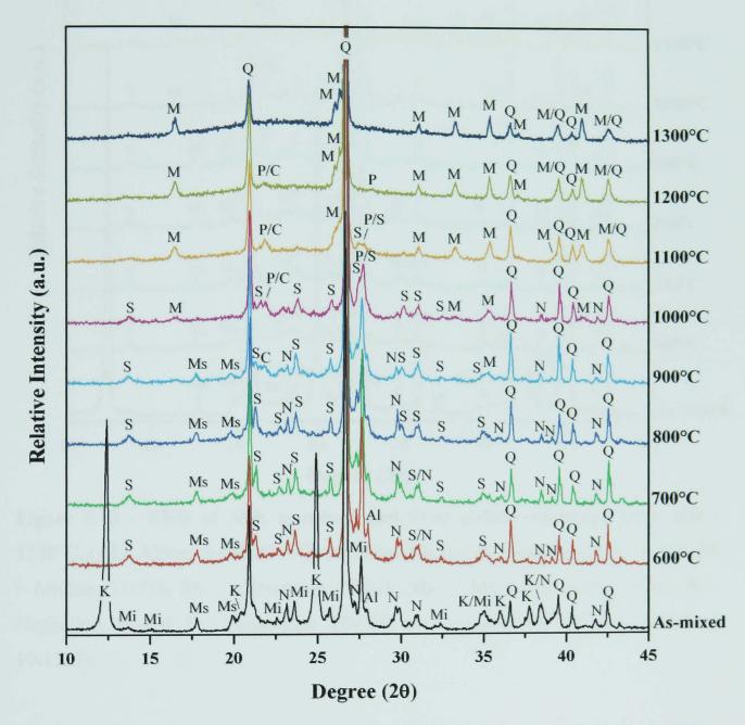
Figure 6.17 - XRD of S25; as-mixed and fired pellets quenched from 600 - 1300°C. (Al – Albite, 9-466, C – Cristobalite, 82-512, K – Kaolinite-1A, 14-164, M – Mullite, 15-776, Mi – Microcline, 19-926, Ms – Muscovite-2M#1, 6-263, N – Nepheline, 35-424, P – Plagioclase, 20-528, Q – α-quartz, 46-1045, S – Sanidine, 19-1227).
