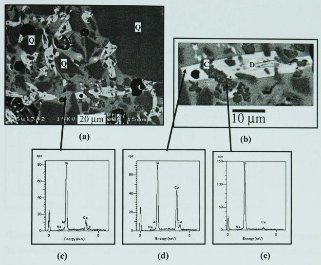
Figure 5.45 - SEM/BS image of a cross-sectioned, polished sample made from Q-SLS fired 3h at 800°C (a). Close up image of individual particles is shown in (b). EDS traces of glassy phase, devitrite particle (D) and cristobalite (C) are shown in (c), (d) and (e).
