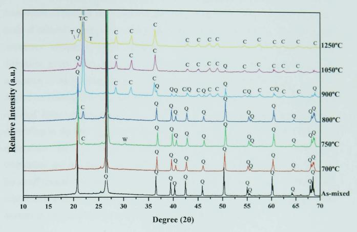
Figure 5.15 - XRD of mixtures of quartz and SLS glass; as-mixed and fired pellets quenched from 700, 750, 800, 900, 1050, and 1250°C are shown (C – Cristobalite, 82-512/39-1425,  $\mathbf{Q}$  –  $\alpha$ -quartz, 46-1045,  $\mathbf{T}$  – Tridymite, 18-1170,  $\mathbf{W}$  –  $\beta$ -wollastonite, 27-88).
