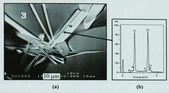
Figure 5.51 - SEM/BS image of a cross-sectioned, polished sample made from NS-SLS fired 3h at 1000°C showing elongated particles (a) and its EDS trace high in Ca and Si (b). (G = glassy phase, W = wollastonite)
