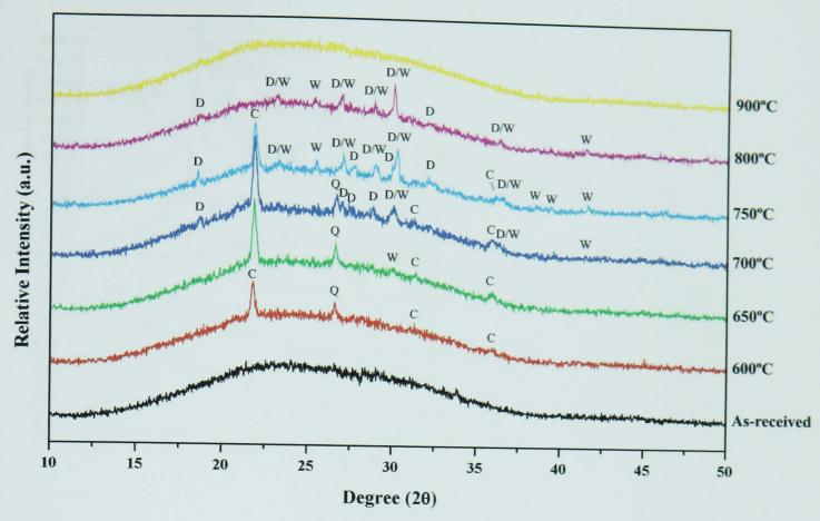
Figure 4.14 - XRD of as-received/powdered SLS glass and of fired SLS pellets quenched from 600, 650, 700, 750, 800 and 900°C. (C – Cristobalite, 82-512, D – Devitrite, 77-410, W – Wollastonite-2M, 27-88)
