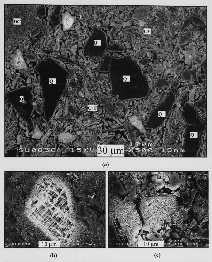
Figure 6.25 - SEM/SE images of polished and etched cross-section of standard whiteware (S0) fired at 1000°C. (a) is the overall microstructure of S0, (b) and (c) show in detail elongated crystals present in S0, which are possibly sillimanite and secondary mullite, respectively. (DC = decomposed clay, C+F = feldsparpenetrated clay relicts, Q = quartz)
