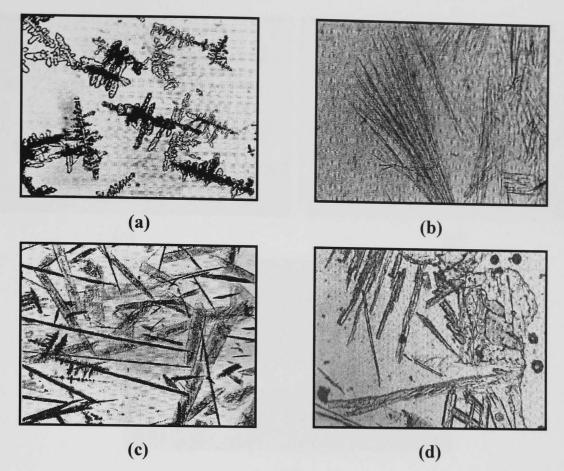
Figure 2.16 - Morphology of crystal phases formed from devitrification of SLS glass; (a) dendrite cristobalite (x50), (b) radiating needle-shaped devitrite (x50), (c) lath-like tridymite (x15), and (d) lath-like α-wollastonite (x48). ((a) and (c) from Taylor and Hill (1952), (b) and (d) from Clark-Monks and Parker (1980))
