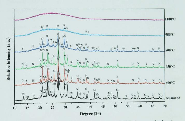
Figure 5.17 - XRD of mixtures of nepheline syenite and SLS glass; as-mixed and fired pellets quenched from 600, 650, 800, 950, and 1100°C are shown (Al - Albite, 9-466, C – Cristobalite, 82-512, Mi – Microcline, 19-932, N – Nepheline, 35-424, S – Sanidine, 19-1227, W – β-wollastonite, 27-88).
