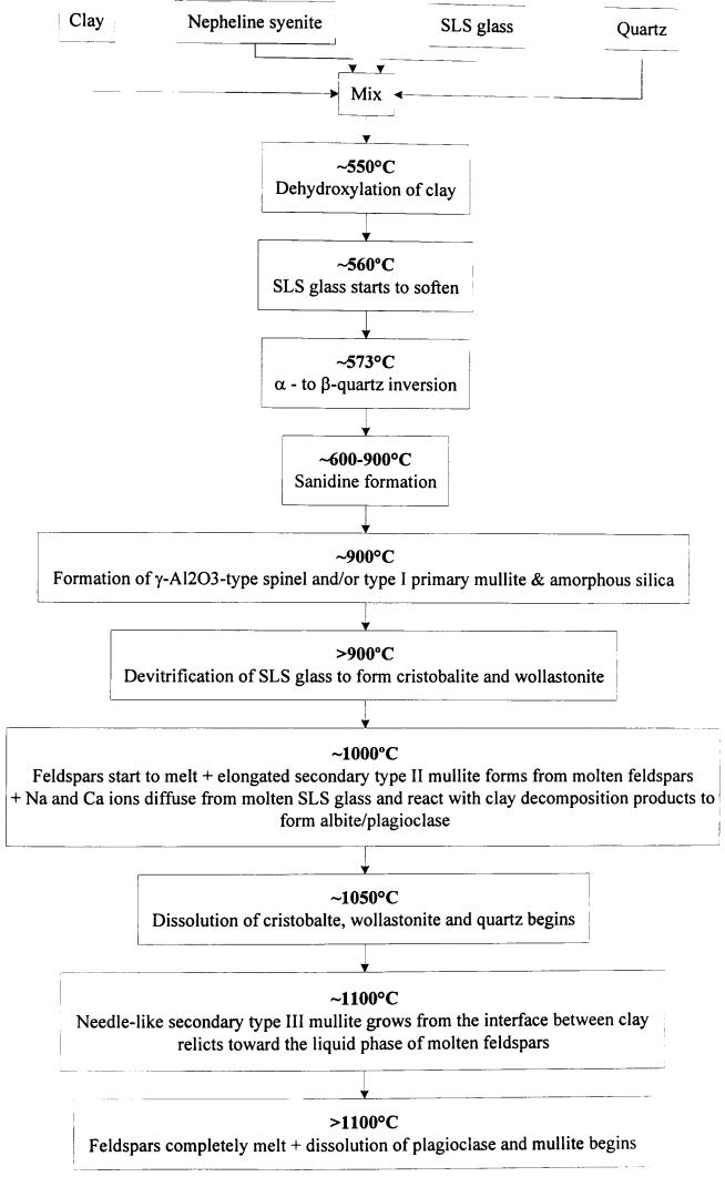
Figure 7.11 - Box diagram of phase evolution on firing partially SLS-fluxed (18.25wt% nepheline syenite and 6.75wt% SLS glass) whiteware at 10°C/min.
