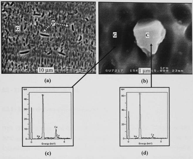
Figure 4.39 - SEM/SE image of cross-sectioned, etched SLS pellets fired 3h at  $1000^{\circ}$ C (a) and (c). EDS of glassy phase and an isolated and irregular particle, near glassy phase are shown in (b) and (d), respectively. (C = cristobalite, G = glassy phase, P = pore)
