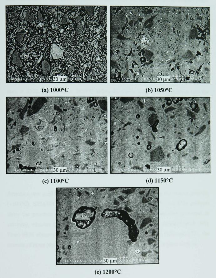
Figure 6.44 - SEM/BS images of polished cross-sections of partially SLS-fluxed whiteware (S25) fired at 1000 - 1200°C ((a)-(e)).
