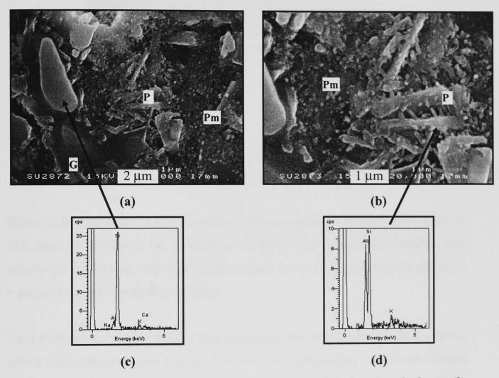
Figure 5.39 - SEM/SE images of a cross-sectioned, polished and etched sample made from C-SLS fired 3h at 1000°C (a), and of a selected area with higher magnification (b). EDS traces from corresponding areas are shown in (c) and (d). (G = glassy phase, Pm = primary mullite)
