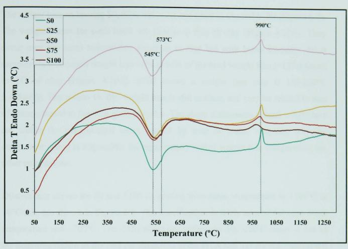
Figure 6.6 - DTA of S0, S25, S50, S75 and S100 with a heating rate of 10°C/min.
