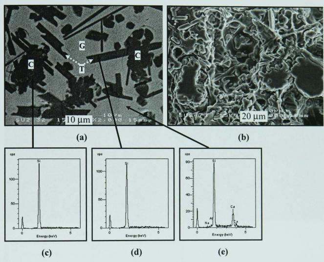
Figure 5.46 - SEM/BS image of a cross-sectioned, unetched (a) and etched sample (b) made from Q-SLS fired 3h at 1000°C. EDS traces of rounded cristobalite (C), elongated tridymite (T) and glassy phase (G) are shown in (c), (d) and (e), respectively.
