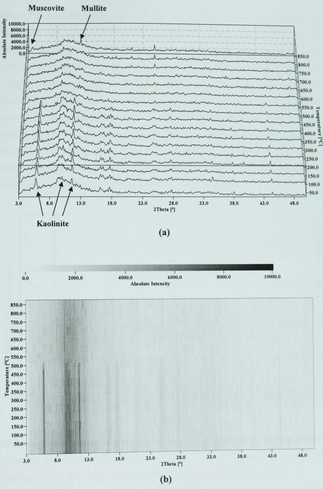
Figure 4.6 - In situ HTXRD of as-received kaolin clay as a function of temperature (a). (b) is a top view perspective of the traces in (a), showing higher peak intensities with darker shades.
