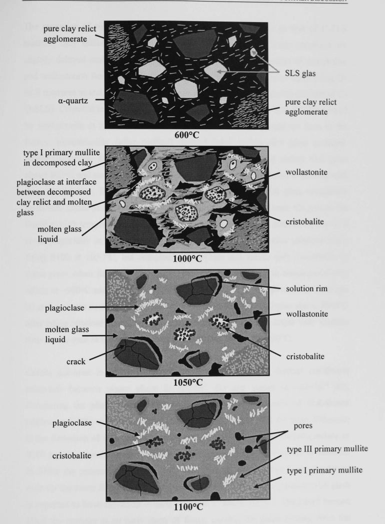
Figure 7.10 - Schematic diagram of the microstructural evolution on firing SLS-fluxed whiteware at 10°C/min.
