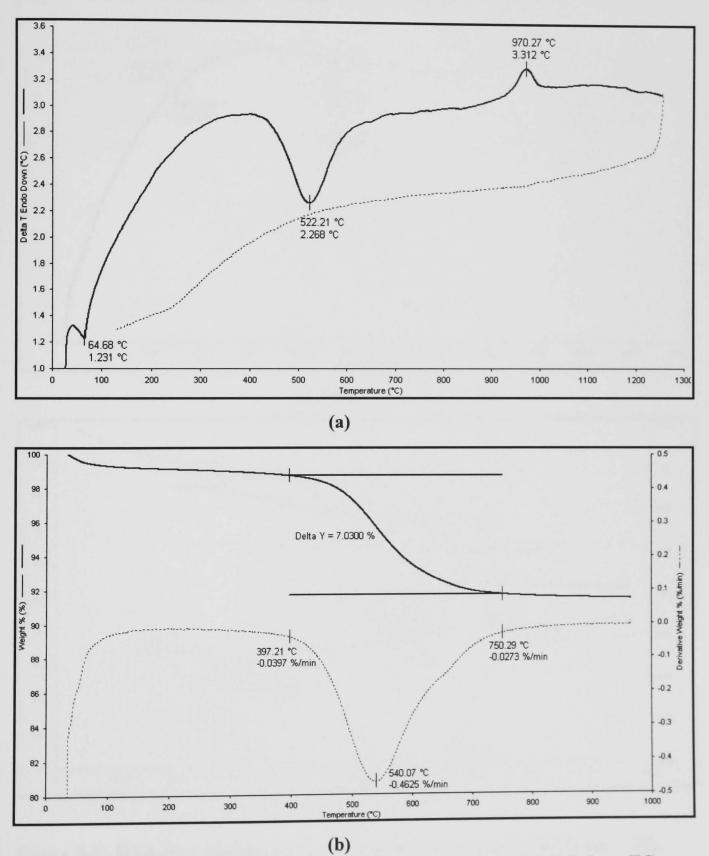
Figure 5.3 - DTA (a; — heating curve, --- cooling curve) and TG/DTG (b; — TG, --- DTG) of the kaolin-SLS glass mixture.
