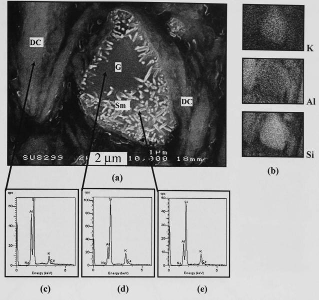
Figure 5.22 - SEM/SE image of cross-sectioned, etched sample made from C-Q pellets fired 3h at 1000°C showing mullite crystals surrounded by decomposed clay (a). X-ray dot mapping is shown in (b), where the brighter regions are higher in the corresponding element. EDS traces from decomposed clay, glassy phase and mullite particles from corresponding areas are shown in (c)-(e). (DC = decomposed clay, G = glassy phase, Sm = secondary mullite)
