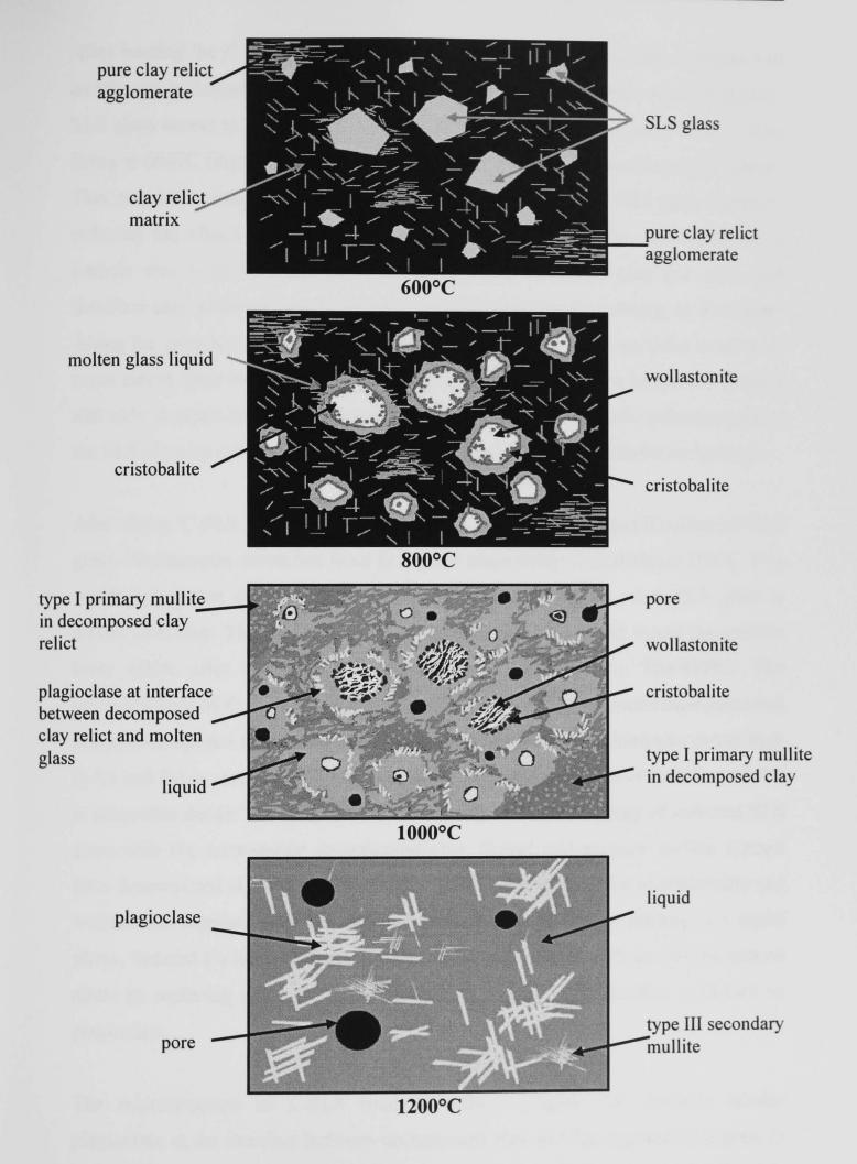
Figure 7.4 - Schematic diagram of microstructural evolution on firing the kaolin clay-SLS glass mixture at 10 °C/min.
