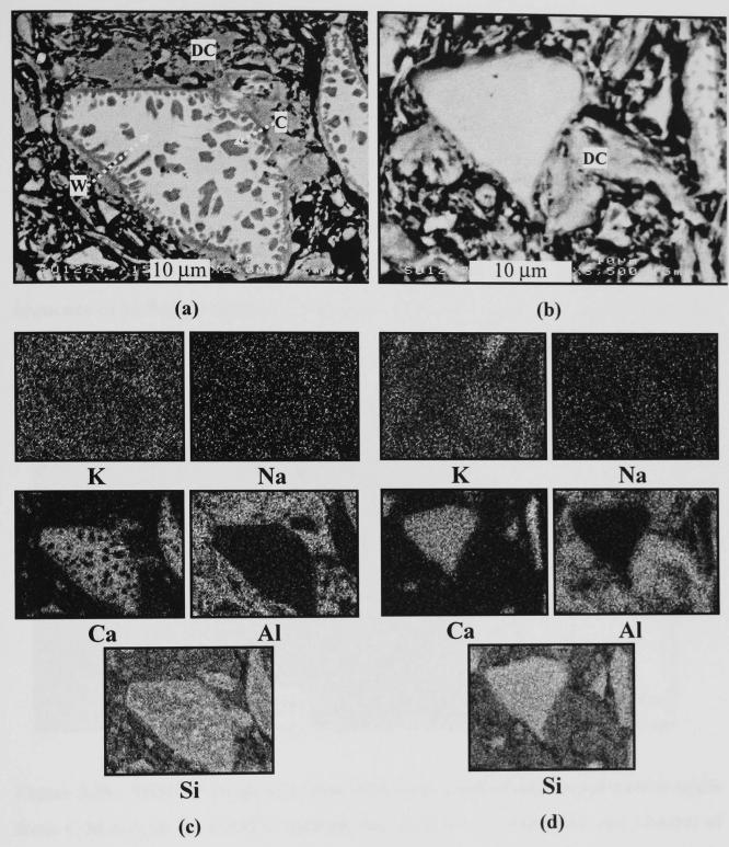
Figure 5.34 - SEM/BS images of cross-sectioned, polished pellets made from C-SLS fired 3h at 800°C showing changes occurring in the SLS (a) and (b). X-ray dot mapping of features (a) and (b) is shown in (c) and (d), respectively. (C = cristobalite, DC = decomposed clay, W = wollastonite)
