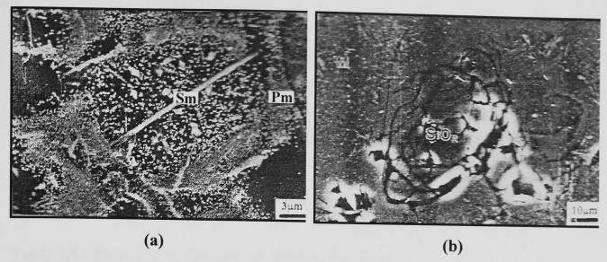
Figure 2.12 – SEM/SE images showing (a) primary mullite (Pm), and secondary mullite (Sm) and (b) cracks within and around quartz (SiO<sub>2</sub>) grain. (Iqbal and Lee, 2000)
