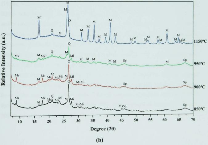
Figure 4.5 - XRD of as-received kaolin clay and of fired pellets quenched from 500, 600, 800 (a) and from 850, 900, 950 and 1150°C (b). (K – Kaolinite-1A, 14-164,  $\mathbf{Q}$  –  $\alpha$ -quartz, 46-1045,  $\mathbf{M}$  – Mullite, 15-776,  $\mathbf{Mi}$  – Microcline, 19-932,  $\mathbf{Ms}$  – Muscovite-2M#1, 6-263,  $\mathbf{Sp}$  –  $\gamma$ -alumina spinel, 10-425).
