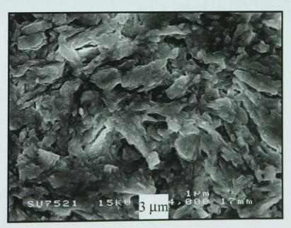
Figure 4.21 - SEM/SE images of cross-sectioned and etched kaolin clay pellets fired 3h at 1000°C.
