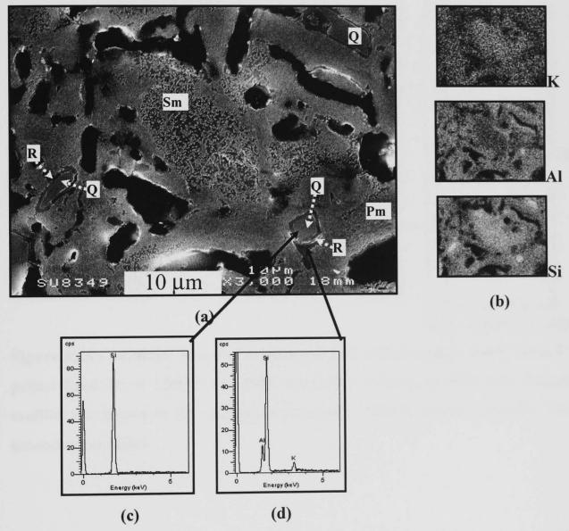
Figure 5.24 - SEM/SE image of cross-sectioned, etched sample made from C-Q pellets fired 3h at 1200°C (a). X-ray dot mapping is shown in (b), where the brighter regions are higher in the corresponding element. EDS traces from quartz particles and glassy phase surrounding quartz from corresponding areas are shown in (c) and (e) respectively. (Pm = primary mullite, Sm =secondary mullite, Q = quartz, R = solution rim)
