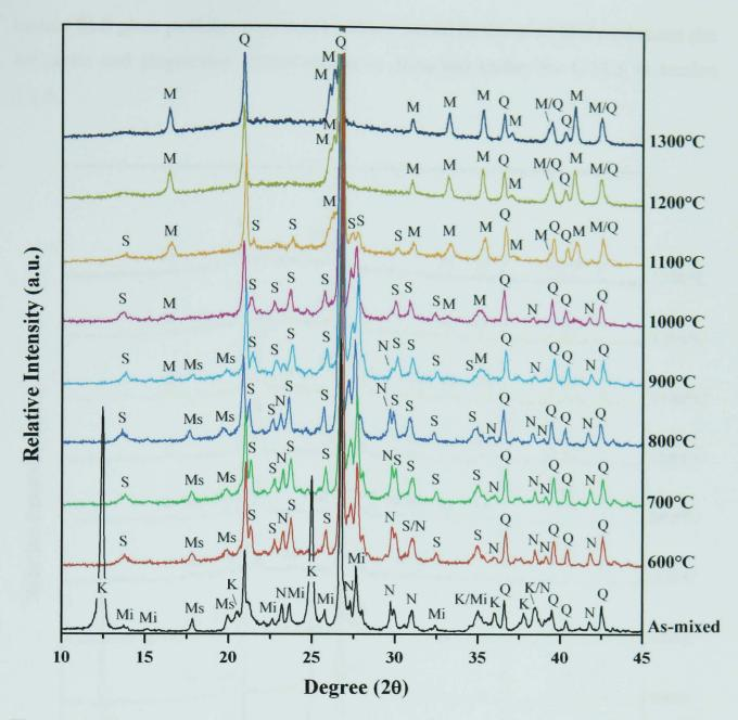
Figure 6.15 - XRD of standard porcelain (S0); as-mixed and fired pellets quenched from 600 -1300°C. (K – Kaolinite-1A, 14-164, M – Mullite, 15-776, Mi – Microcline, 19-926, Ms - Muscovite-2M#1, 6-263, N – Nepheline, 35-424,  $\mathbf{Q} - \alpha$ -quartz, 46-1045,  $\mathbf{S}$  – Sanidine, 19-1227).
