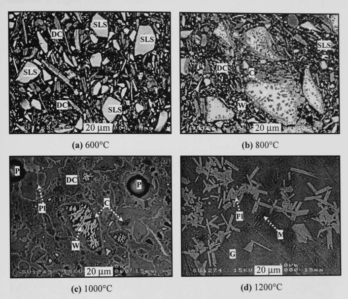
Figure 5.32 - SEM/BS images of cross-sectioned, polished C-SLS pellets fired 3h at 600°C (a), 800°C (b), 1000°C (c), and 1200°C (d). (C = cristobalite, DC= decomposed clay, G = glassy phase, M = mullite, P = pore, Pl = plagioclase, SLS = soda-lime-silica glass, W = wollastonite)
