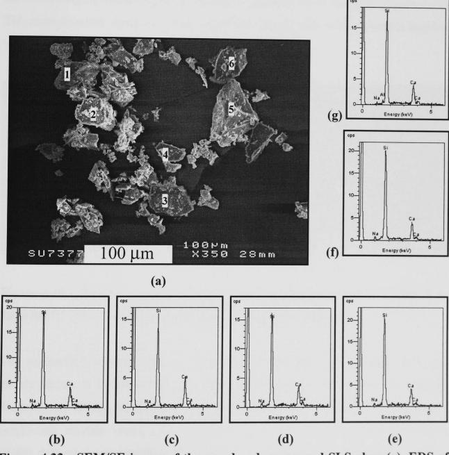
Figure 4.33 - SEM/SE image of the powdered, as-ground SLS glass (a). EDS of randomly selected SLS particles labelled "1", "2", "3", "4", "5" and "6" are shown in (b) - (g) respectively.
