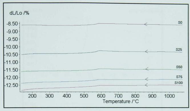
Figure 6.12 - Dilatometric curves of S0, S25, S50, S75 and S100 on cooling at 10°C/min from 1100°C to room temperature.
