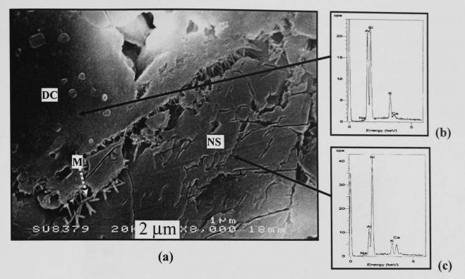
Figure 5.28 - SEM/SE image of a cross-sectioned, etched sample made from C-NS pellets fired 3h at 1000°C (a). EDS traces from decomposed clay and nepheline syenite particles are shown in (b) and (c), respectively. (DC = decomposed clay, M = mullite, NS = nepheline syenite)
