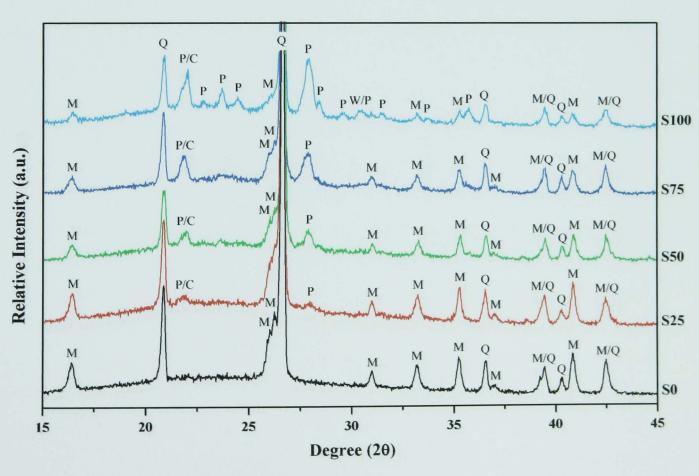
Figure 6.22 - XRD of each batch fired at 1100°C for 3h.
