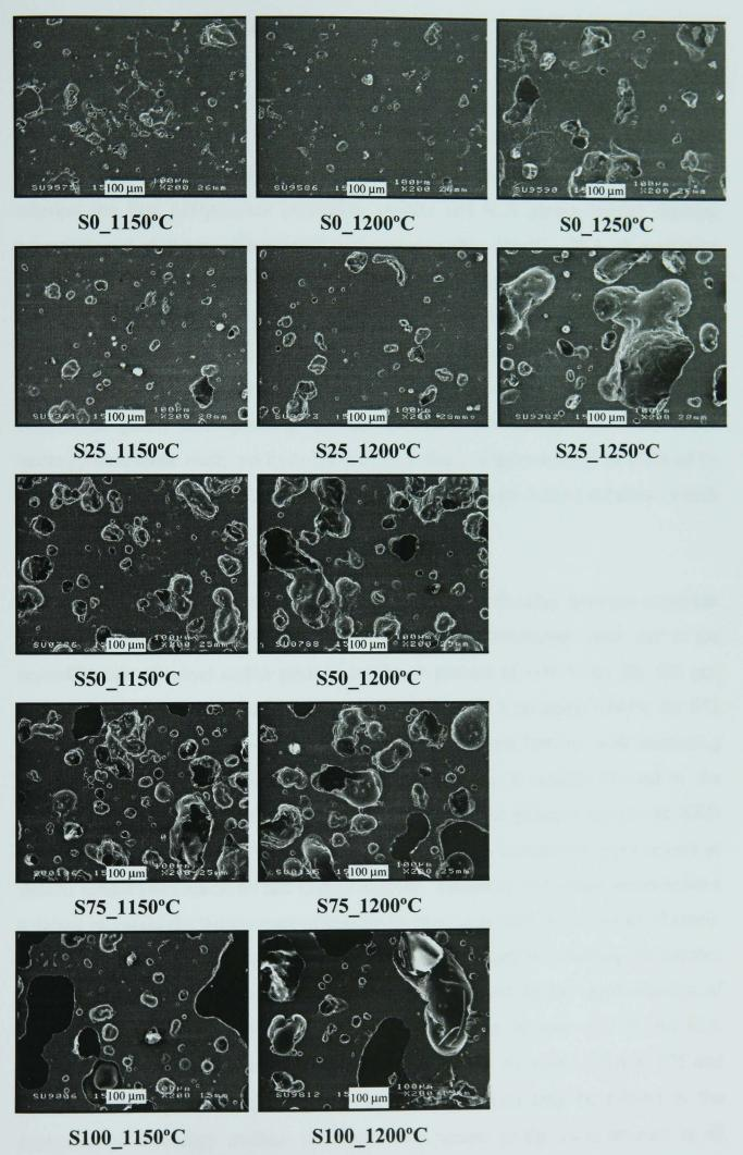
Figure 6.5 - SEM/SE images of S0 and S25 fired at 1150, 1200 and 1250°C and that of S50, S75 and S100 fired at 1150 and 1200°C.
