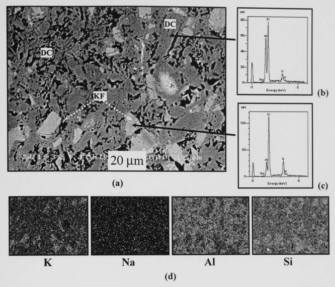
Figure 5.27 - SEM/BS image of a cross-sectioned, polished pellet made from C-NS fired at 1000°C. (b) and (c) are EDS traces of decomposed clay relicts (dark grey) and of the irregular K-feldspar crystals (brighter grey particles) shown in (a), respectively. X-ray dot mapping is shown in (d), where the brighter regions are higher in the corresponding element. (DC = decomposed clay, KF = K-feldspar)
