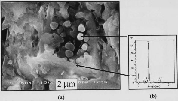
Figure 5.36 - SEM/SE image of a cross-sectioned, polished and etched sample made from C-SLS fired 3h at 800°C showing the presence of cristobalite and absence of wollastonite after etching (a). EDS trace of cristobalite and edge of a glass particle is shown in (b).
