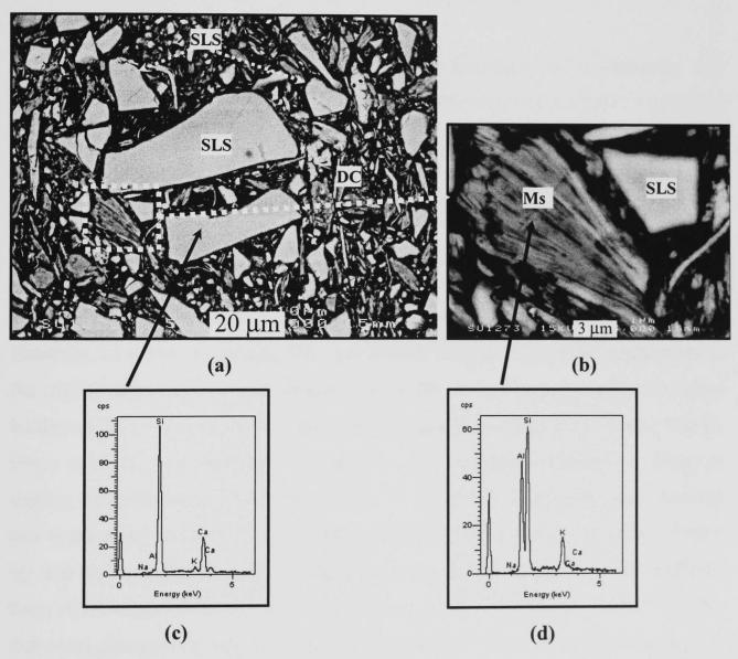
Figure 5.33 - SEM/BS images of a cross-sectioned, polished sample made from C-SLS fired 3h at 600°C (a), and of muscovite relict present in this sample (b). (c) is an EDS trace for the irregular SLS crystals shown in (a), and (d) is an EDS trace for the muscovite crystal in (b). (DC = decomposed clay, Ms = muscovite, SLS = soda-lime-silica glass)
