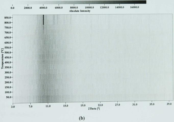
Figure 4.15 - In situ HTXRD of ground SLS waste glass as a function of temperature (a). (b) is a top view perspective of the traces in (a), showing higher peak intensities with darker shades.
