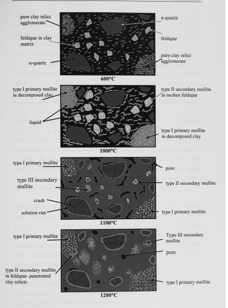
Figure 7.8 - Schematic diagram of the microstructural evolution on firing standard (nepheline syenite-fluxed) whiteware at 10°C/min.
