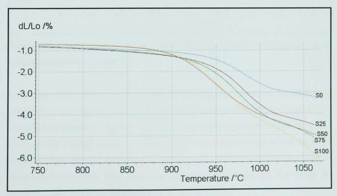
Figure 6.10 - Dilatometric curves of S0, S25, S50, S75 and S100 on heating at 10°C/min from 750 to 1100°C.
