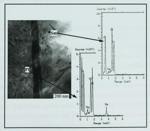
Figure 6.40 - TEM/BF image together with EDS traces from areas within the plagioclase crystal (Pl) and the secondary mullite crystal (Sm).
