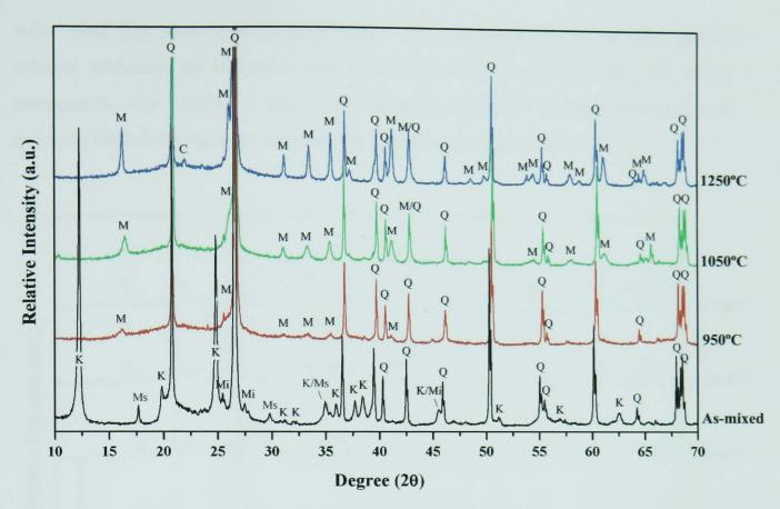
Figure 5.7 - XRD of mixtures of kaolin clay and quartz; as-mixed and fired pellets quenched from 950, 1050, and 1250°C (C – Cristobalite, 82-512, K – Kaolinite-1A, 14-164, M – Mullite, 15-776, Mi – Microcline, 19-926, Ms – Muscovite-2M#1, 6-263,  $\mathbf{Q} - \alpha$ -quartz, 46-1045).
