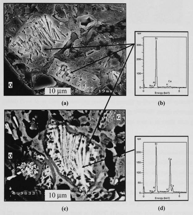
Figure 6.31 - SEM/SE image of etched sample (a) and SEM/BS image of unetched sample from SLS-fluxed whiteware (S100) fired 3h at 1000°C. EDS of the corresponding areas are shown in (b) and (c).
