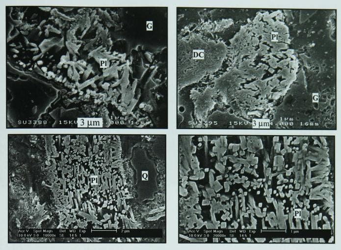
Figure 6.39 - SEM/SE images of SLS-fluxed whiteware (S100) fired at 1100°C, showing tabular plagioclase. (Pl = plagioclase, Q = quartz, G = glassy phase, DC = decomposed clay)
