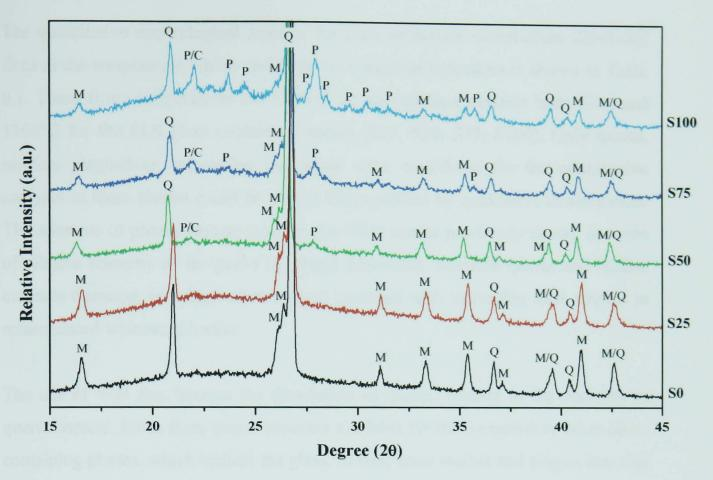
Figure 6.23 - XRD of each batch fired at 1150°C for 3h.
