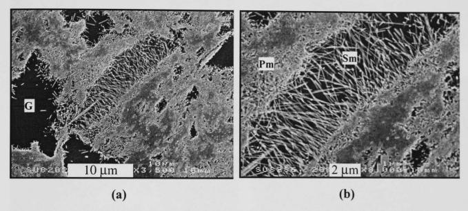
Figure 5.31 - SEM/SE image of a cross-sectioned, etched sample made from C-NS pellets fired 3h at 1200°C (a) and of selected area in high magnification (b) showing small primary mullite crystals and needle-like mullite crystals. (G = glassy phase, Pm = primary mullite, Sm = secondary mullite)
