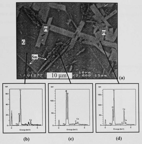
Figure 5.40 - SEM/BS image of a cross-sectioned, polished sample made from C-SLS fired 3h at 1200°C (a). EDS traces of glassy phase, needle-like mullite and tabular plagioclase are shown in (b), (c) and (d), respectively. (G = glassy phase, Pl = plagioclase, Sm = secondary mullite)
