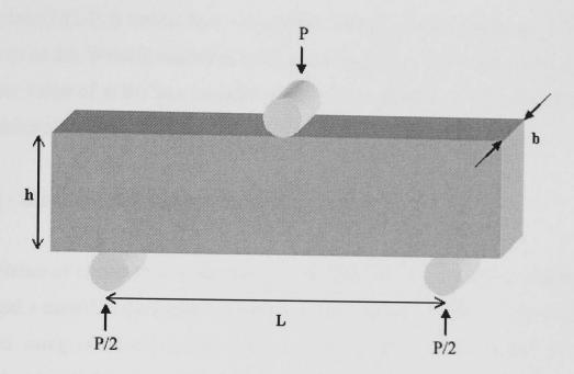
Figure 3.3 - Schematic illustration of three-point bending configuration.
