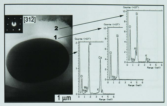
Figure 6.49 - BF-TEM image from S25 fired at 1100°C. SADP is from wollastonite, and EDS spectra are from the wollastonite particle and the surrounding glass.
