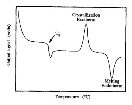
Figure 2.14 - DSC curve of a glass. (Shelby, 2005)
