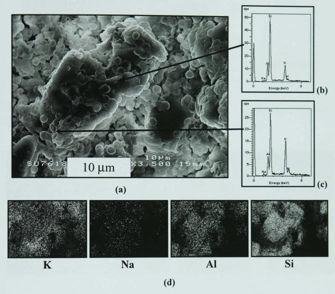
Figure 4.30 - SEM/SE image of cross-sectioned, etched nepheline syenite fired at 1000°C. EDS of a large particle in the centre and rounded particles on top of it are shown in (b) and (c), respectively. X-ray dot maps are shown in (d), where the brighter regions are higher in the corresponding elements.
