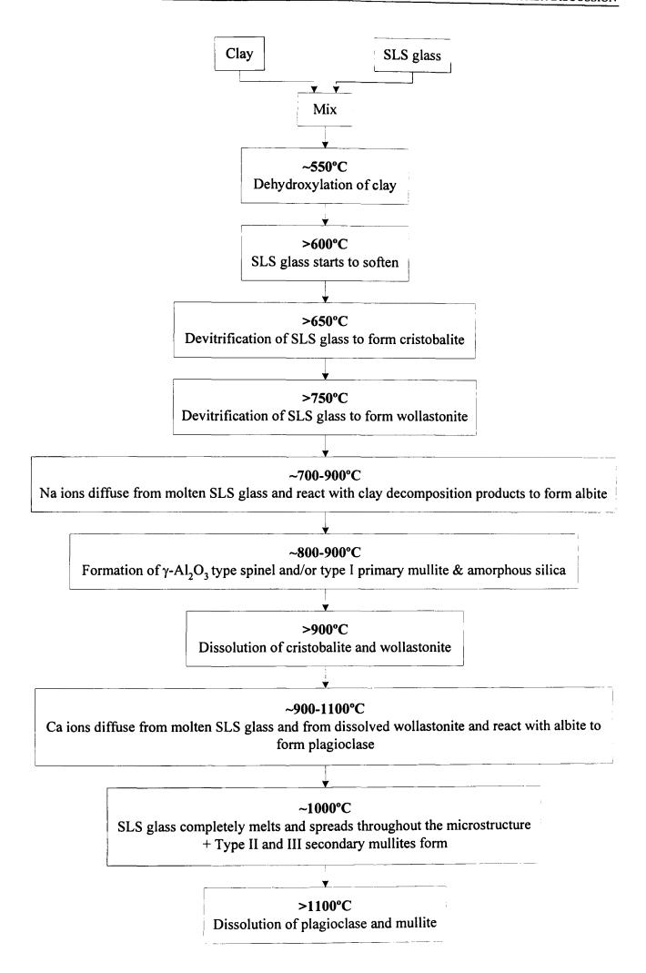
Figure 7.3 - Box diagram of phase evolution in the kaolin clay-SLS glass mixture for firing at 10°C/min.
