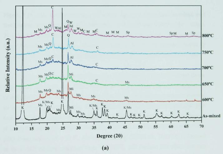
Figure 5.11 - (a) XRD of mixtures of kaolin clay and SLS glass; as-mixed and fired pellets quenched from 600, 650, 700, 750 and 800°C. (Al – Albite, 71-1153, C – Cristobalite, 82-512, K – Kaolinite-1A, 14-164, M – Mullite, 15-776, Mi – Microcline, 19-926, Ms – Muscovite-2M#1, 6-263, P – Plagioclase, 20-528, Q –  $\alpha$ -quartz, 46-1045, Sp –  $\gamma$ -alumina spinel, 10-425, W – Wollastonite-2M, 27-88).
