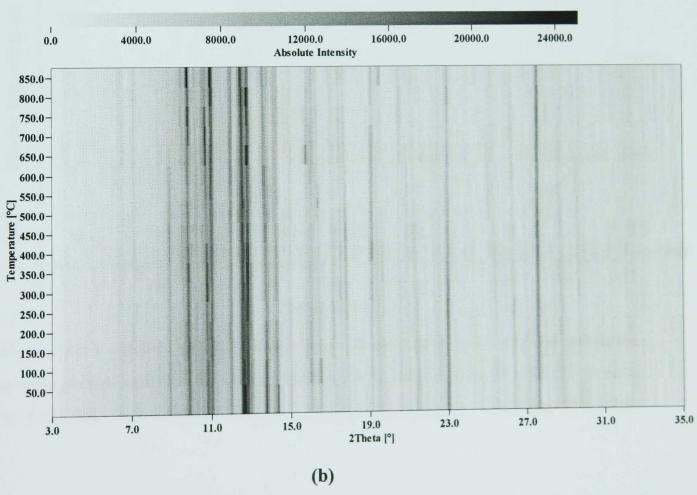
Figure 4.12 - In situ HTXRD of as-received nepheline syenite as a function of temperature (a). (b) is a top view perspective of the traces in (a), showing higher peak intensities with darker shades.
