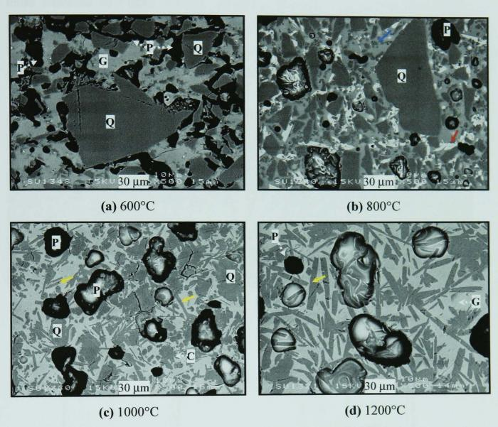
Figure 5.43 - SEM/BS images of Q-SLS fired 3h at 600°C (a), 800°C (b), 1000°C (c) and 1200°C (d). (C= cristobalite, G = glassy phase, P = pore, Q = quartz)
