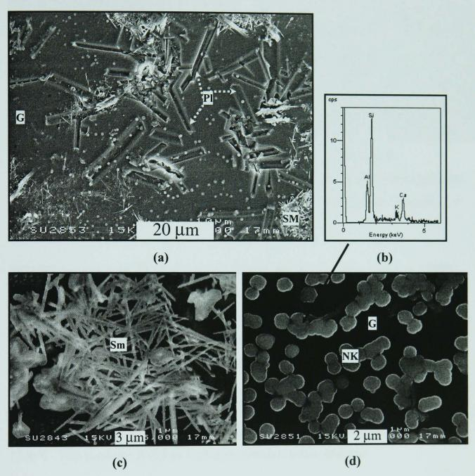
Figure 5.41 - SEM/SE image of a cross-sectioned, polished and etched sample made from C-SLS fired 3h at 1200°C (a). Aggregated acicular mullite crystals are shown in (c), and spheroidal nepheline (NK) crystals are shown in (d) with their EDS (b). (G = glassy phase, Pl = plagioclase, NK = nepheline, Sm = secondary mullite)
