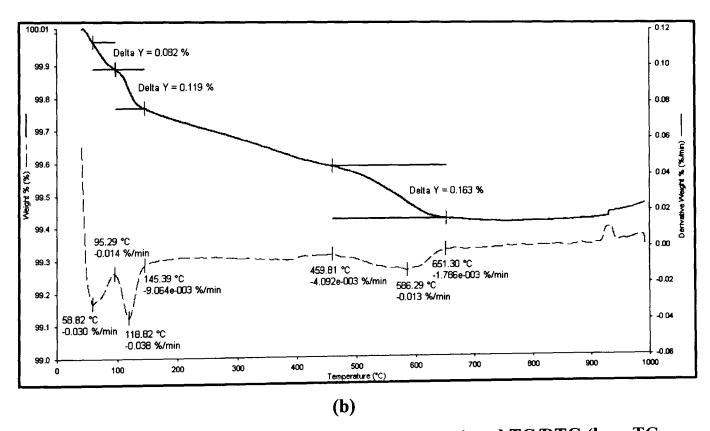
Figure 4.4 - DTA (a; — heating curve, --- cooling curve) and TG/DTG (b; — TG, --- DTG) of SLS glass mix.
