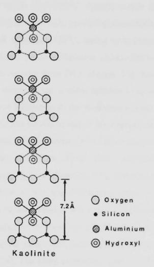
Figure 2.1 - a-b projection of the layer structure of kaolinite; the c axis spacing is 7.2 Å. (Rice, 1987)
