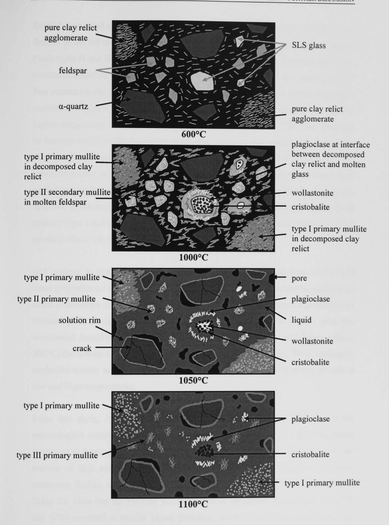
Figure 7.12 - Schematic diagram of the microstructural evolution on firing partially SLS-fluxed (18.25wt% nepheline syenite and 6.75wt% SLS glass) whiteware at 10°C/min.
