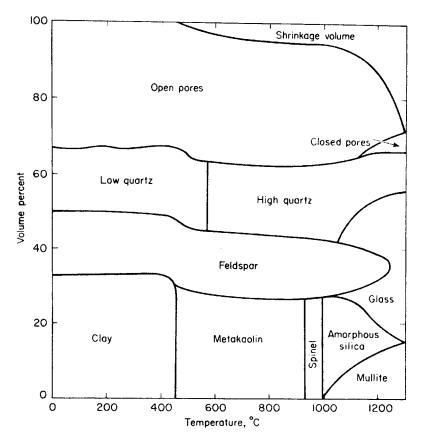
Figure 2.10 - Constituents in a triaxial body on firing. (Norton, 1970)
