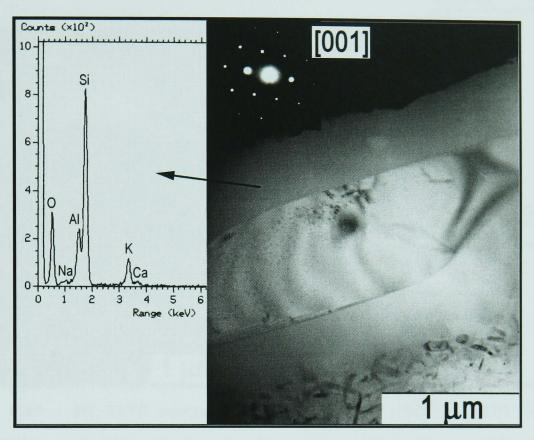
Figure 6.48 - BF-TEM image of S25 fired at 1100°C. The SADP is from the partially dissolved quartz particle and the EDS spectrum from the solution rim.
