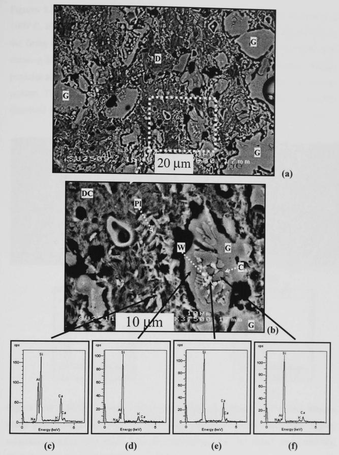
Figure 5.38 - SEM/BS images of a cross-sectioned, polished and etched sample made from C-SLS fired 3h at 1000°C (a) and of a selected area with higher magnification (b). EDS traces from corresponding areas are shown in (c)-(f). (C = cristobalite, DC = decomposed clay, G = glassy phase, Pl = plagioclase, W = wollastonite)
