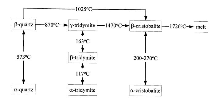
Figure 2.6 - Polymorphic transformations of silica. (Hlavac, 1983) Horizontal arrows are reconstructive transformations (conversions), and vertical arrows are displacive transformations (inversions).
