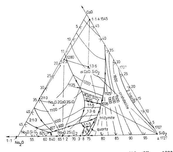
Figure 2.15 - Phase diagram of the system Na<sub>2</sub>O-CaO-SiO<sub>2</sub>. (Hlavac, 1983)
