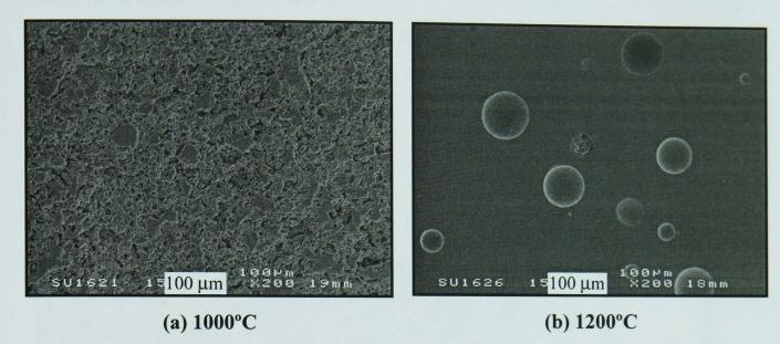
Figure 4.27 - SEM/SE images of cross-sectioned nepheline syenite pellets fired at (a) 1000°C, and (b) 1200°C for 3h.
