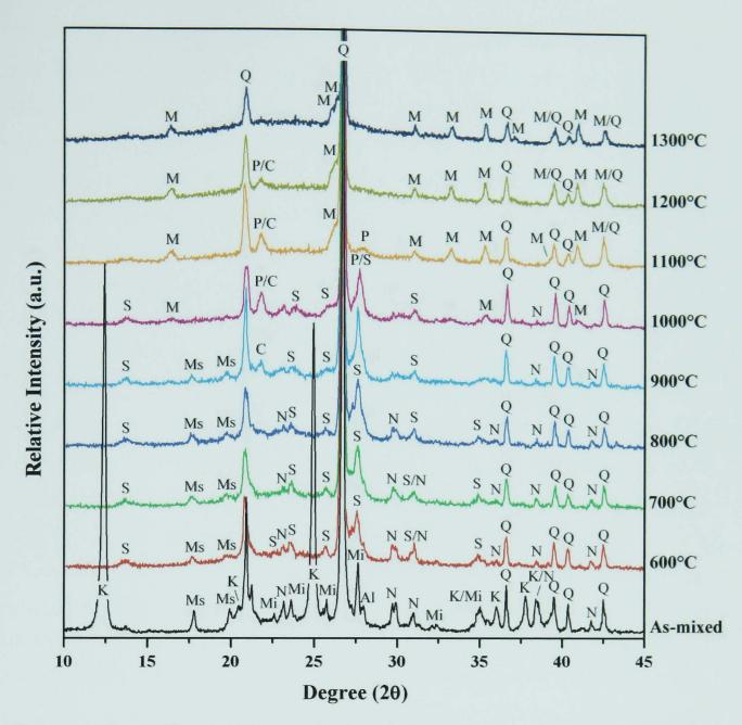
Figure 6.18 - XRD of S50; as-mixed and fired pellets quenched from 600 - 1300°C. (Al – Albite, 9-466, C – Cristobalite, 82-512, K – Kaolinite-1A, 14-164, M – Mullite, 15-776, Mi – Microcline, 19-926, Ms – Muscovite-2M#1, 6-263, N – Nepheline, 35-424, P – Plagioclase, 20-528, Q – α-quartz, 46-1045, S – Sanidine, 19-1227).
