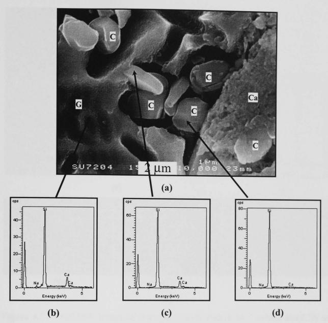
Figure 4.36 - SEM/SE image of cross-sectioned, etched SLS glass pellets fired 3h at 800°C (a). EDS of glassy phase, cristobalite particle near glassy phase and the cristobalite particle are shown in (b), (c) and (d), respectively. (C = cristobalite, Ca = calcium-bearing phase, G = glassy phase)
