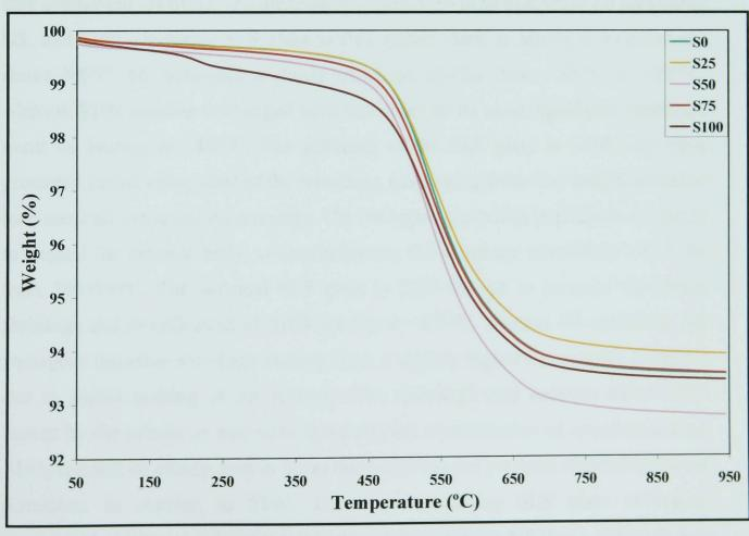
Figure 6.7 - TG traces of S0, S25, S50, S75 and S100 with a heating rate of 10°C/min.
