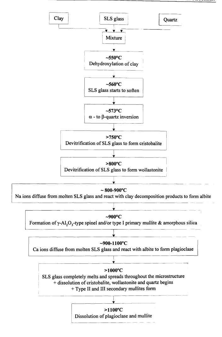
Figure 7.9 - Box diagram of phase evolution on firing SLS-fluxed whiteware at 10°C/min.
