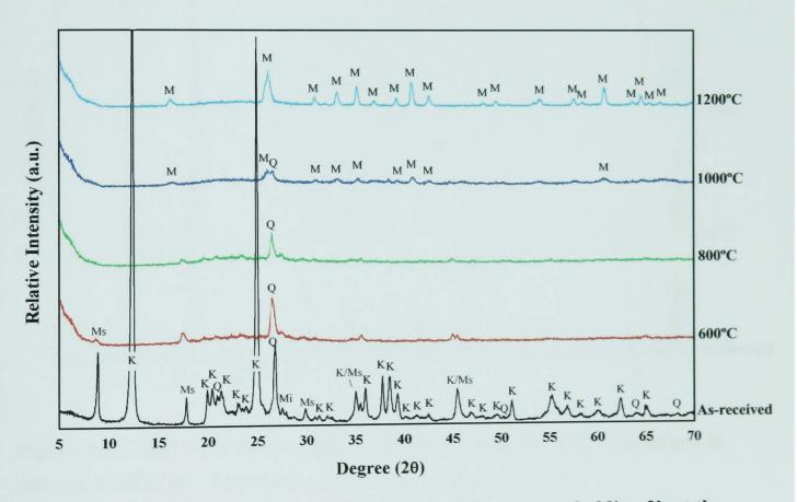
Figure 4.7 - XRD of as-received kaolin clay and of fired pellets holding 3h at the indicated temperatures. (K – Kaolinite-1A, 14-164, Q – α-quartz, 46-1045, M – Mullite, 15-776, Mi – Microcline, 19-932, Ms – Muscovite-2M#1, 6-263)
