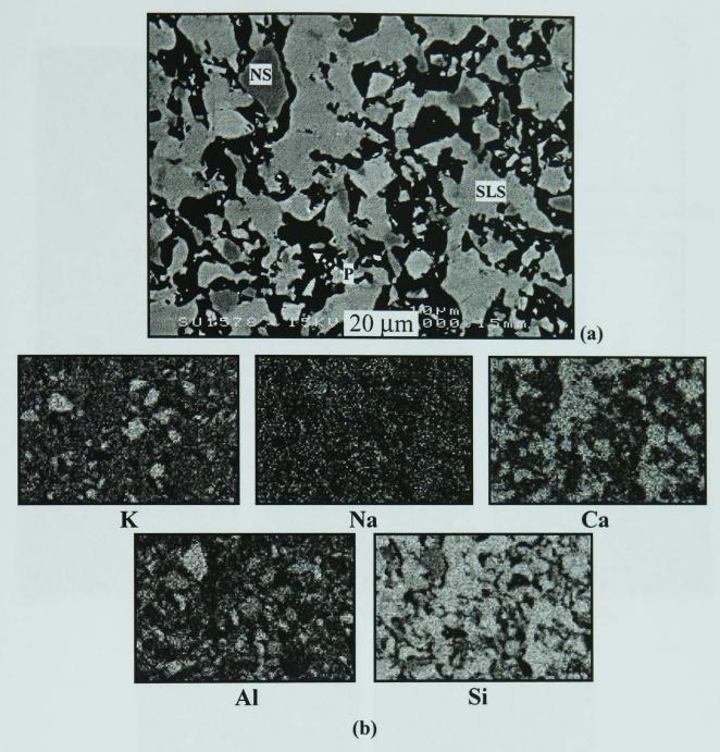
Figure 5.49 - SEM/BS image of a cross-sectioned, polished pellet made from NS-SLS fired 3h at 600°C. X-ray dot mapping is shown in (b), where the brighter regions are higher in the corresponding element.
