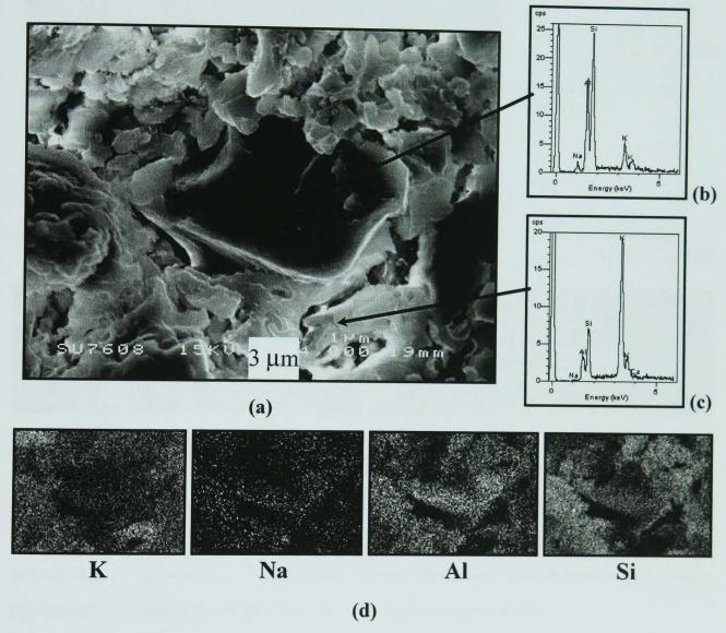
Figure 4.29 - SEM/SE image of cross-sectioned, etched nepheline syenite fired at 1000°C (a). (b) and (c) are EDS of particles in the middle and in the right bottom corner of (a), respectively. X-ray dot maps are shown in (d), where the brighter regions are higher in the corresponding elements.
