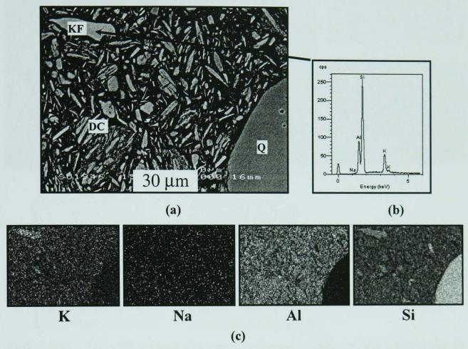
Figure 5.20 - SEM/BS image of a cross-sectioned, polished pellet made from C-Q fired 3h at 1000°C (a). (b) is an EDS trace for the irregular K-feldspar crystal shown in the top left corner of (a). X-ray dot mapping is shown in (c), where the brighter regions are higher in the corresponding element. (DC = decomposed clay, KF = K-feldspar, Q = quartz)
