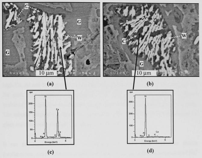
Figure 5.37 - SEM/BS images of a cross-sectioned, polished and etched sample made from C-SLS fired 3h at 1000°C showing the formation of wollastonite (bright features) and cristobalite (dark rounded particles in the background) in both (a) and (b). EDS traces of wollastonite and cristobalite are shown in (c) and (d), respectively. (C = cristobalite, G = glassy phase, W = wollastonite)
