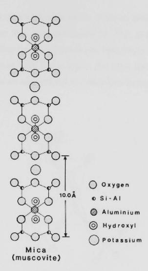
Figure 2.3 - a-b projection of the layer structure of muscovite; the c axis spacing is 10 Å. (Rice, 1987)
