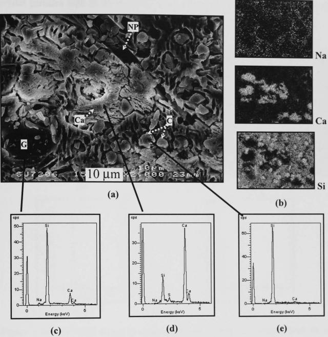
Figure 4.38 - SEM/SE image of cross-sectioned, etched SLS pellets fired 3h at 800°C showing high a Ca-bearing phase surrounded by cristobalite and glassy phase (a). X-ray dot maps are shown in (b), where the brighter regions are higher in the corresponding element. EDS from corresponding areas are shown in (c)-(e). (C = cristobalite, Ca = calcium-bearing phase, G = glassy phase, NP = needle-like pore)
