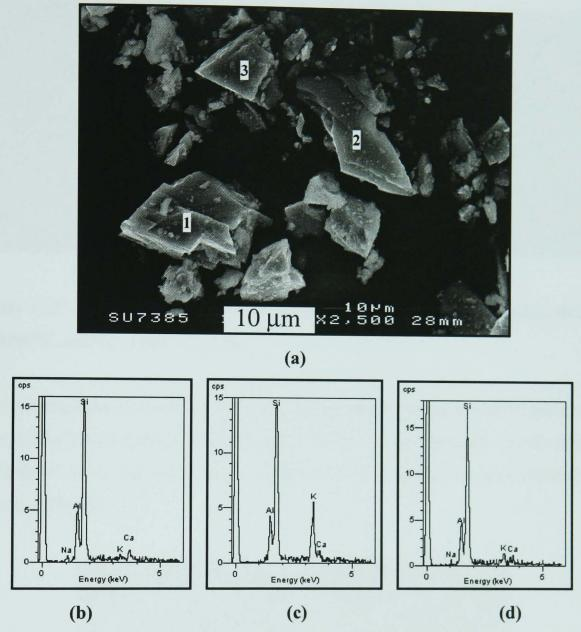
Figure 4.26 - SEM/SE image of as-received nepheline syenite (a). EDS of selected nepheline syenite particles labelled "1", "2" and "3" are shown in (b) - (d), respectively.
