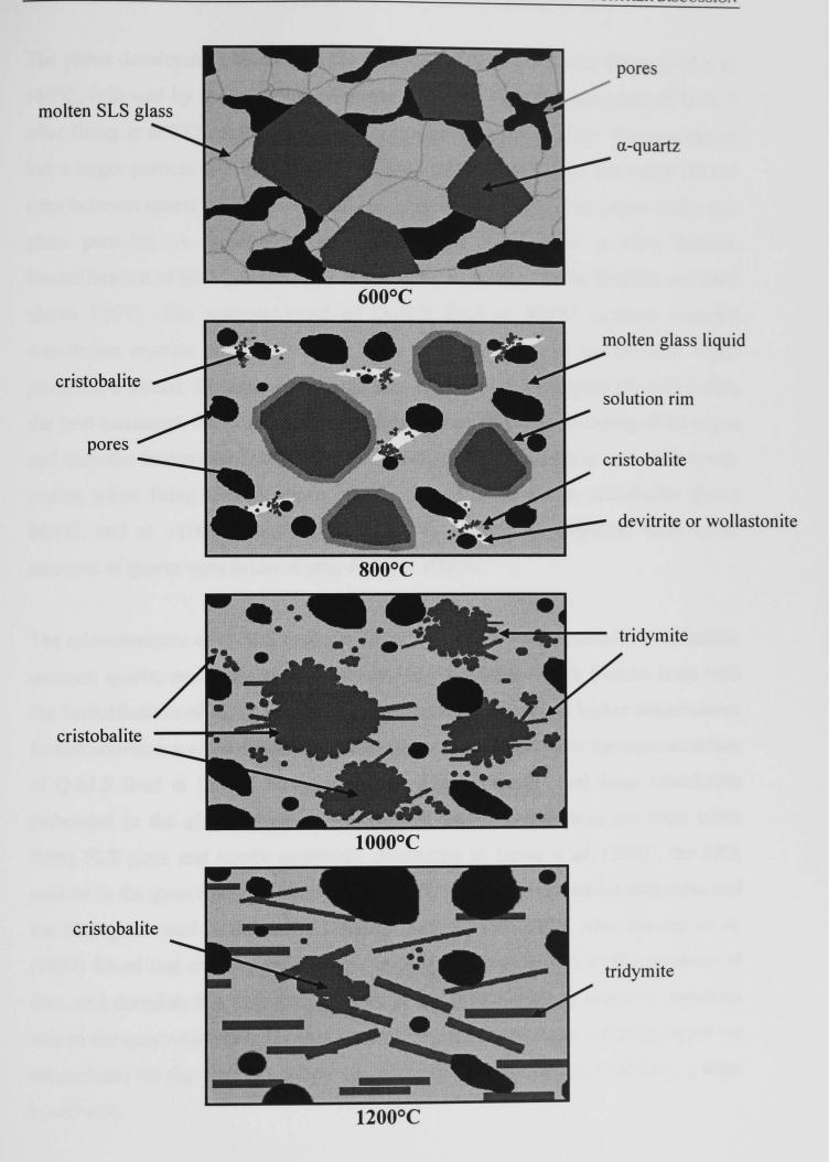
Figure 7.6 - Schematic diagram of the microstructural evolution on firing the quartz-SLS glass mixture at 10°C/min.
