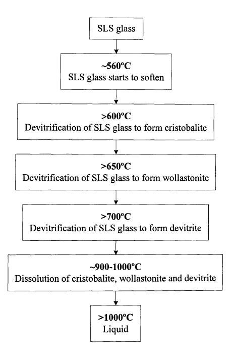
Figure 7.1 - Box diagram of phase evolution on firing SLS glass at 10°C/min.
