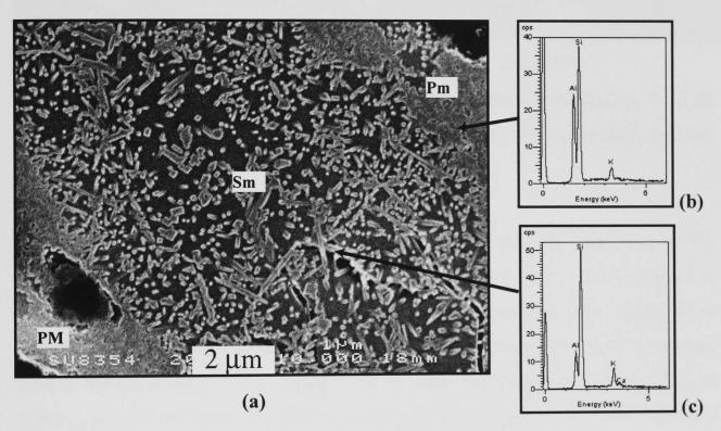
Figure 5.25 - SEM/SE image of cross-sectioned, etched sample made from C-Q pellets fired 3h at 1200°C (a). EDS traces for primary mullite and elongated mullite are shown in (b) and (c), respectively. (Pm = primary mullite, Sm = secondary mullite)
