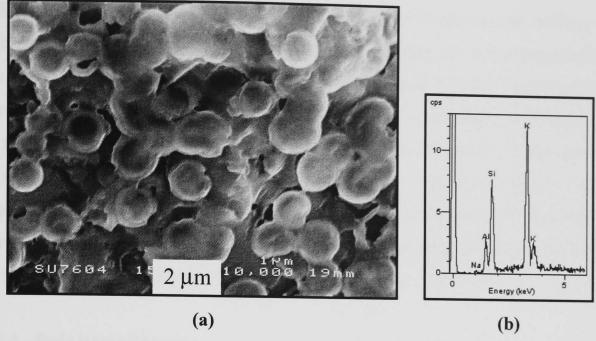
Figure 4.31 - SEM/SE image of cross-sectioned, etched nepheline syenite pellets fired at 1000°C, showing rounded particles (a) and their EDS (b).
