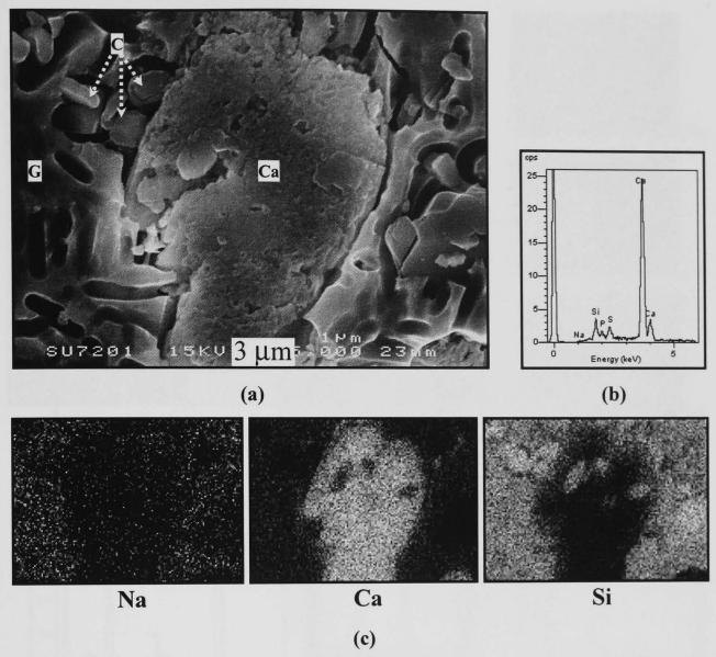
Figure 4.37 - SEM/SE image of cross-sectioned, etched SLS pellets fired 3h at 800°C showing a high Ca-bearing phase (a). EDS from this Ca-bearing phase is shown in (b) and X-ray dot maps are shown in (c), where the brighter regions are higher in the corresponding element. (C = cristobalite, Ca = calcium-bearing phase, G = glassy phase)
