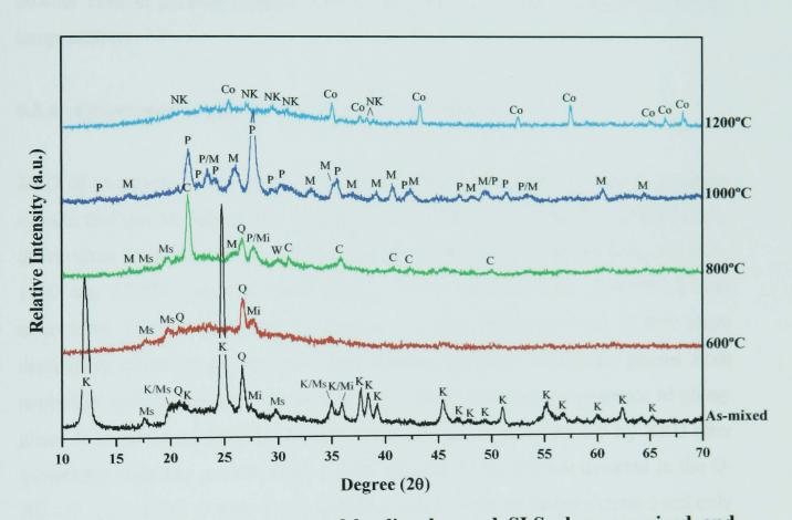
Figure 5.12 - XRD of mixtures of kaolin clay and SLS glass; as-mixed and pellets fired 3h at 600, 800, 1000, and 1200°C and normally cooled are shown (Al – Albite, 71-1153, C – Cristobalite, 82-512, Co – Corundum, 46-1212, K – Kaolinite-1A, 14-164, M – Mullite, 15-776, Mi – Microcline, 19-926, Ms – Muscovite-2M#1, 6-263, NK – Nepheline, 9-338, P – Plagioclase, 20-528, Q – α-quartz, 46-1045, W – Wollastonite-2M, 27-88).
