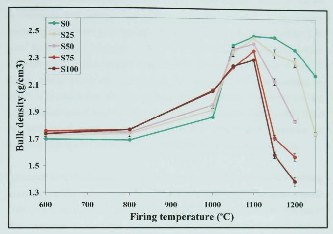
Figure 6.1 - Bulk densities of as-fired specimens from all batches. (Heating at 10°C/min, holding time 3h and cooling at 10°C/min).
