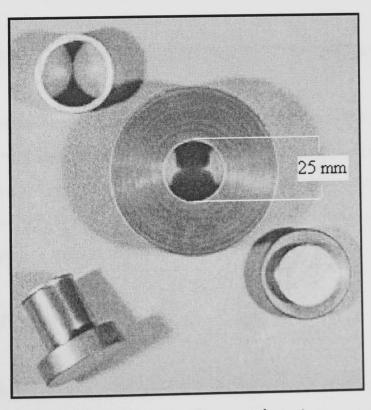
Figure 3.1 - Cylindrical steel die used in the pressing step.
