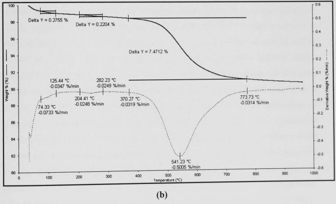
Figure 5.2 - DTA (a; — heating curve, --- cooling curve) and TG/DTG (b; — TG, --- DTG) of the kaolin-nepheline syenite mixture.
