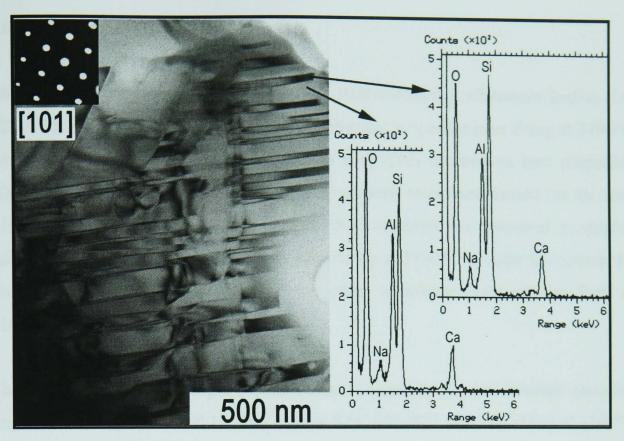
Figure 6.50 - BF TEM image and a corresponding SADP of plagioclase, together with EDS spectra of regions within the crystal.
