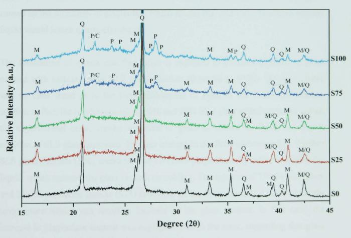
Figure 6.24 - XRD of each batch fired at 1200°C for 3h.
