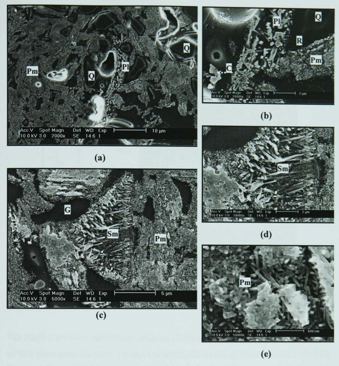
Figure 6.47 - SEM/SE images of polished and etched cross-sections of partial SLS-fluxed whiteware (S25) fired at 1100°C showing main features present. (Pm = primary mullite, Sm = secondary mullite, Q = quartz, Pl = plagioclase, C = cristobalite, G = glassy phase, R = solution rim)
