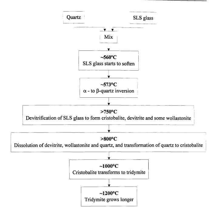
Figure 7.5 - Box diagram of phase evolution on firing the quartz-SLS glass mixture at 10°C/min.
