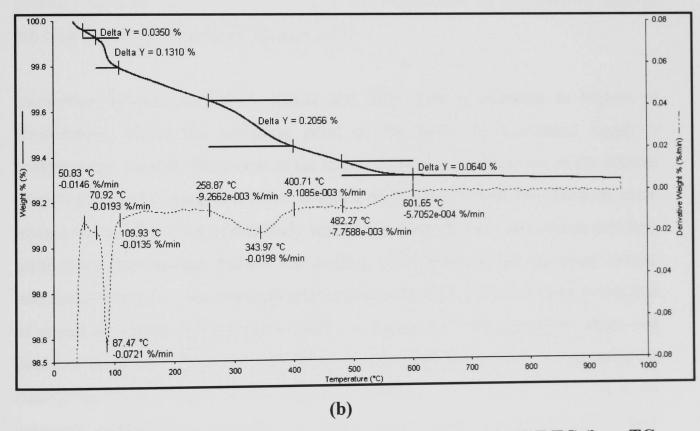
Figure 5.5 - DTA (a; — heating curve, --- cooling curve) and TG/DTG (b; — TG, --- DTG) of the quartz-SLS glass mixture.
