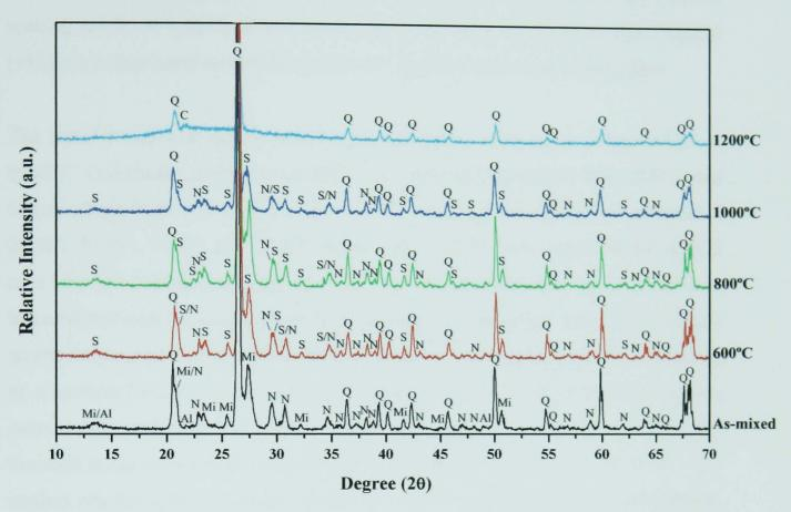
Figure 5.14 - XRD of mixtures of quartz and nepheline syenite; as-mixed, fired 3h at 600, 800, 1000, and 1200°C and normally cooled are shown (Al – Albite, 9-466, C – Cristobalite, 39-1425, Mi – Microcline, 19-932, N – Nepheline, 35-424, S – Sanidine, 19-1227,  $\mathbf{Q} - \alpha$ -quartz, 46-1045).
