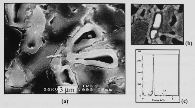
Figure 6.32 - SEM/SE image of polished and etched SLS-fluxed whiteware (S100) fired 3h at 1000°C, showing remnants (mostly in the rims) of melted SLS glass particles rich in Si (a) and their EDS trace (c). SEM/BS image of unetched sample (b) showing Ca-rich (brighter) areas in the centre of small SLS glass particle.
