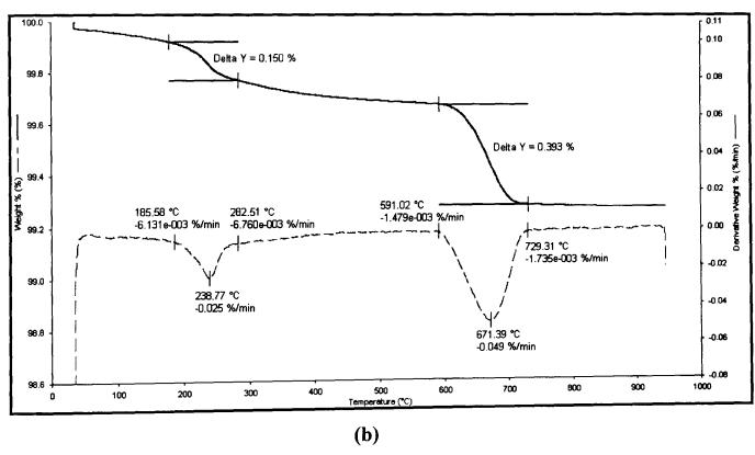
Figure 4.3 - DTA (a; - heating curve, --- cooling curve) and TG/DTG (b; - TG, --- DTG) of nepheline syenite.
