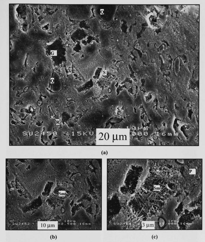
Figure 6.26 - SEM/SE images of polished and etched cross-sections of standard whiteware (S0) fired at  $1100^{\circ}$ C. (a) is the overall microstructure of S0, (b) and (c) show in detail needle-like secondary mullite and cuboidal primary mullite crystals presented in S0. (Pm = primary mullite, Sm = secondary mullite, Q = quartz, R = solution rim, G = glassy phase)
