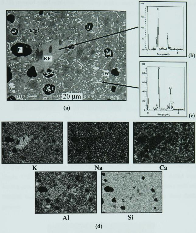
Figure 5.50 - SEM/BS image of a cross-sectioned, polished pellet made from NS-SLS fired at 800°C. (b) is an EDS trace for the irregular light grey K-feldspar crystal shown in the centre of (a). X-ray dot mapping is shown in (c), where the brighter regions are higher in the corresponding element. (KF = K-feldspar, P = pore, W = wollastonite)
