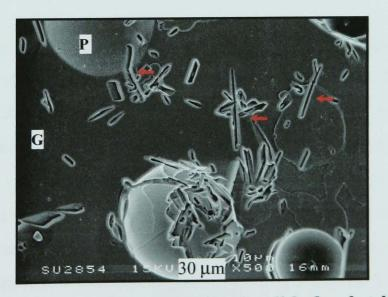
Figure 5.52 - SEM/BS image of a cross-sectioned, polished and etched sample made from NS-SLS fired 3h at 1000°C showing elongated particles. (G = glassy phase, P = pore)
