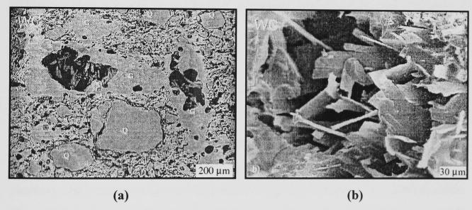
Figure 2.19 - SEM/SE images of polished SLS-containing roofing tiles (WC) fired at 1000°C showing softened glass grains adhering to surrounding matrix (a), quartz (Q) grains and glass (G) grains. (b) Plate-like wollastonite crystals in the glass grain centre. (Pontikes et al., 2005)
