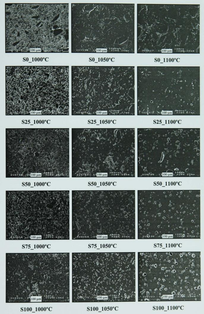
Figure 6.4 - SEM/SE images of the cross-sectioned compacts made of S0, S25, S50, S75 and S100 fired at 1000, 1050 and 1100°C.
