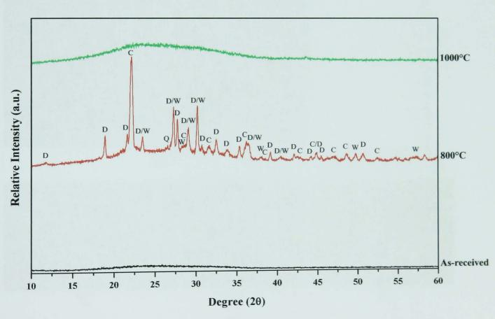
Figure 4.16 - XRD of as-received SLS glass and fired SLS glass pellets held for 3h at the indicated temperatures (C – Cristobalite, 82-512, D – Devitrite, 77-410, W – Wollastonite-2M, 27-88).
