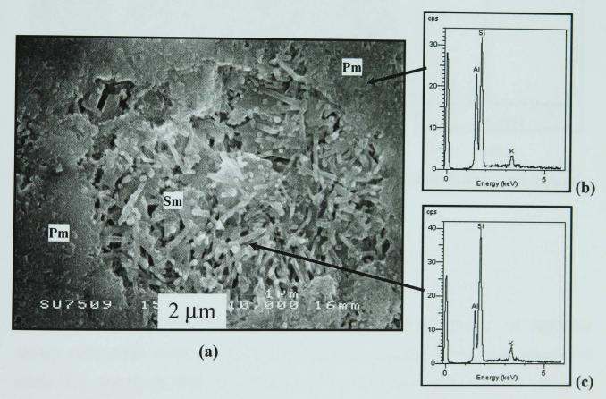
Figure 4.24 - SEM/SE image of cross-sectioned, etched kaolin clay pellets fired 3h at 1200°C. (a) shows mullite particles. (b) is EDS of scale-like crystals, and (c) is EDS of rod-like crystals shown in (a). (Pm = primary mullite, Sm = secondary mullite)
