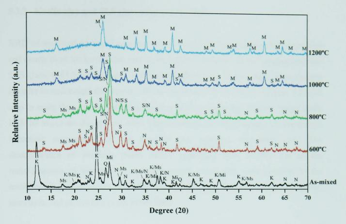
Figure 5.10 - XRD of mixtures of kaolin clay and nepheline syenite; as-mixed and fired 3h at 600, 800, 1000, and 1200°C and normally cooled are shown (K – Kaolinite-1A, 14-164, M – Mullite, 15-776, Mi – Microcline, 19-926, Ms – Muscovite-2M#1, 6-263, N – Nepheline, 35-424,  $\mathbf{Q}$  –  $\alpha$ -quartz, 46-1045,  $\mathbf{S}$  – Sanidine, 19-1227).
