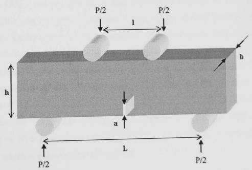
Figure 3.4 - Four-point bending fixture and notched specimen for fracture toughness  $(K_{IC})$  measurements.
