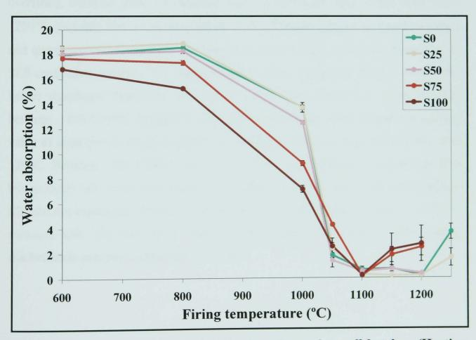
Figure 6.2 - Water absorption of as-fired specimens from all batches. (Heating at 10°C/min, holding time 3h and cooling at 10°C/min).
