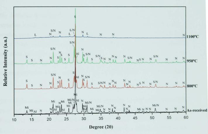
Figure 4.11 - XRD of as-received nepheline syenite and of fired nepheline syenite pellets quenched from 800, 950 and 1100°C. (Al – Albite, 9-466, L – Leucite, 71-1147, Mi – Microcline, 19-932, N – Nepheline, 35-424, S – Sanidine, 19-1227)
