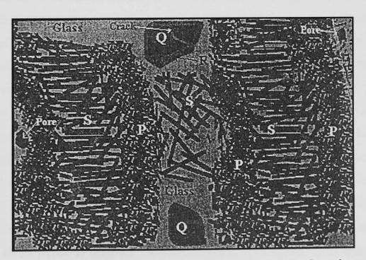
Figure 2.11 - Schematic of the general features observed in the microstructure of a whiteware body. (P = primary mullite, S = secondary mullite, Q =  $\alpha$ -quartz, R = solution rim) (Iqbal and Lee, 1999)
