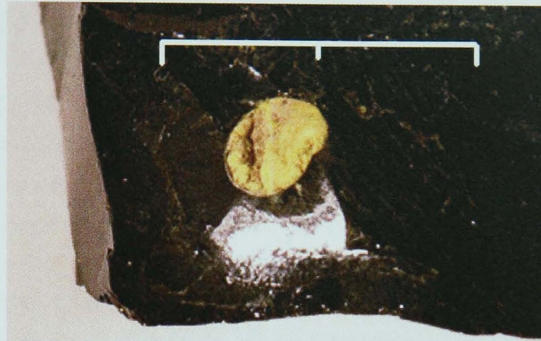
Figure 1.7 – Yellow Phase peanut found in a full scale simulated HLW glass Scale bar = 2cm
