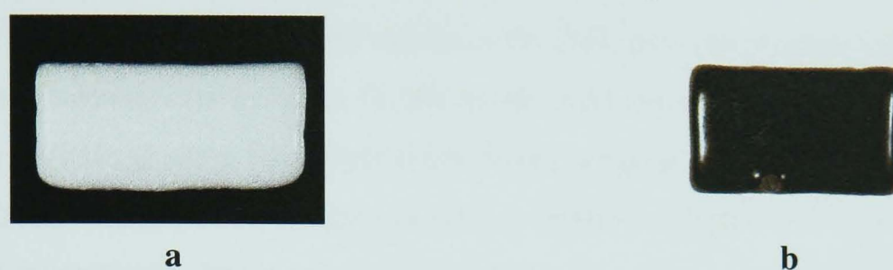
Figure 6.11 – (a)Glass 14(air) as cast, (b)Glass 14(red) as cast
