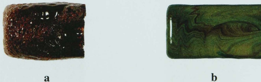
Figure 4.16 – As cast samples of (a) glass 9(air) and (b) glass 9(red)
