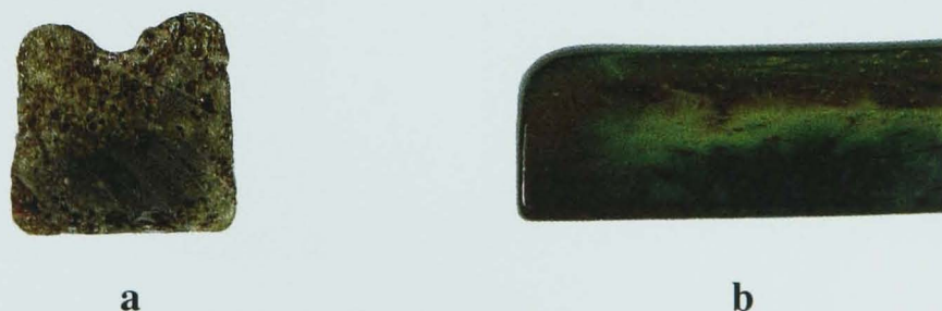
Figure 4.11 – As cast samples of (a)glass 7(air), (b)glass 7(red)
