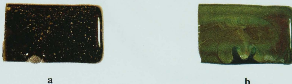
Figure 4.14 – As cast samples of (a) glass 8(air) and (b) glass 8(red)
