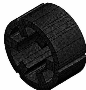
(d) coils removed, but their mass uniformly distributed over stator
