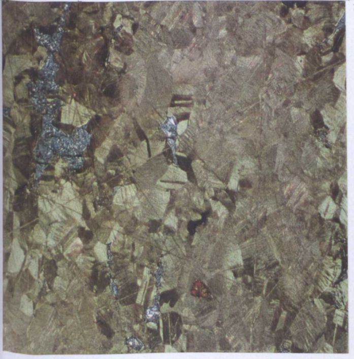
Bottom: Grain Size Groups d, e & f (WR 1, LM 135, Ex 28)
