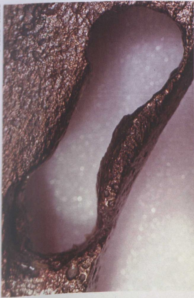
(i) 'Slot' between rivet holes (Museum of London O 1347)
