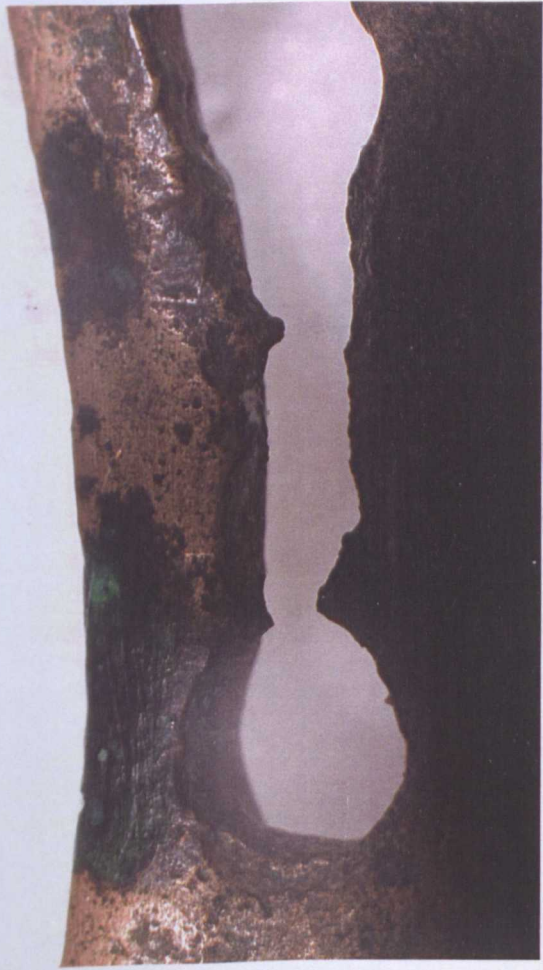
(ii) 'Slot' between rivet holes (Cambridge Museum Z 46784)
