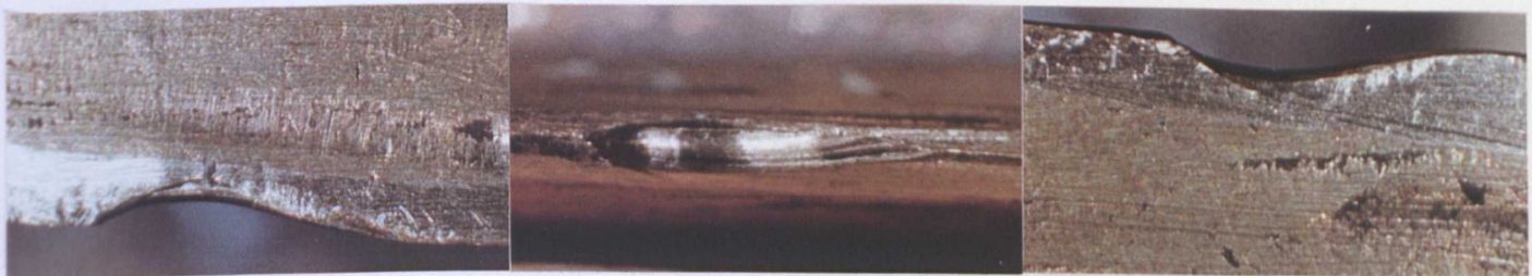
(ii) Chipped (bowed and chipped)
