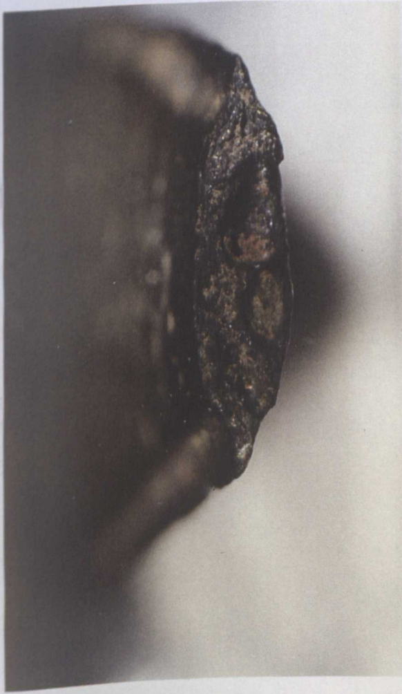
(i) Broken sword tip showing porosity (CMAA 83.161)
