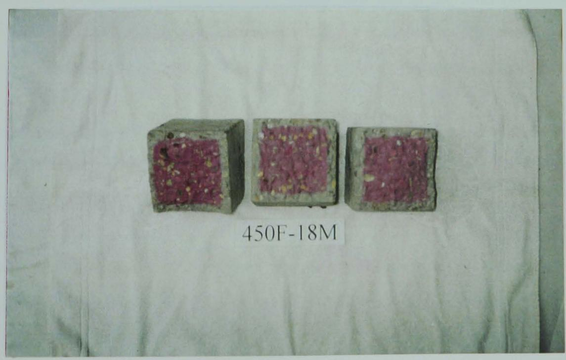
Figure 4-48 Carbonation of specimens stored in the laboratory-540 days
