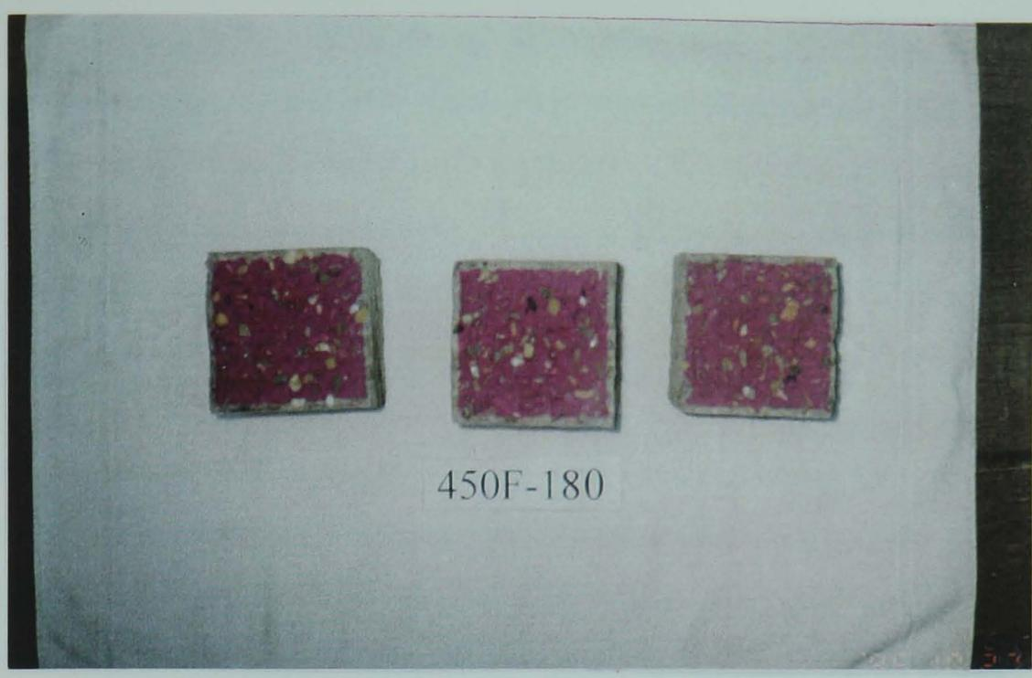
Figure 4-47 Carbonation of specimens stored in the laboratory-180 days
