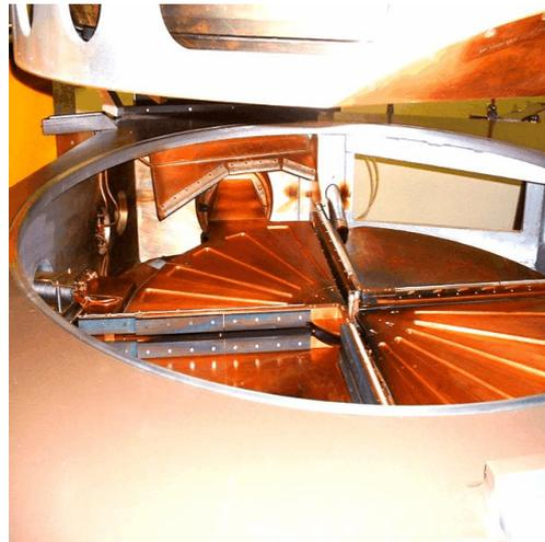
Figure 8.1: Four hollow metal dees at the MC40 Birmingham Cyclotron with two grounded and two which apply radio frequency (RF) voltage. The dees alternate between grounded and RF [93].
