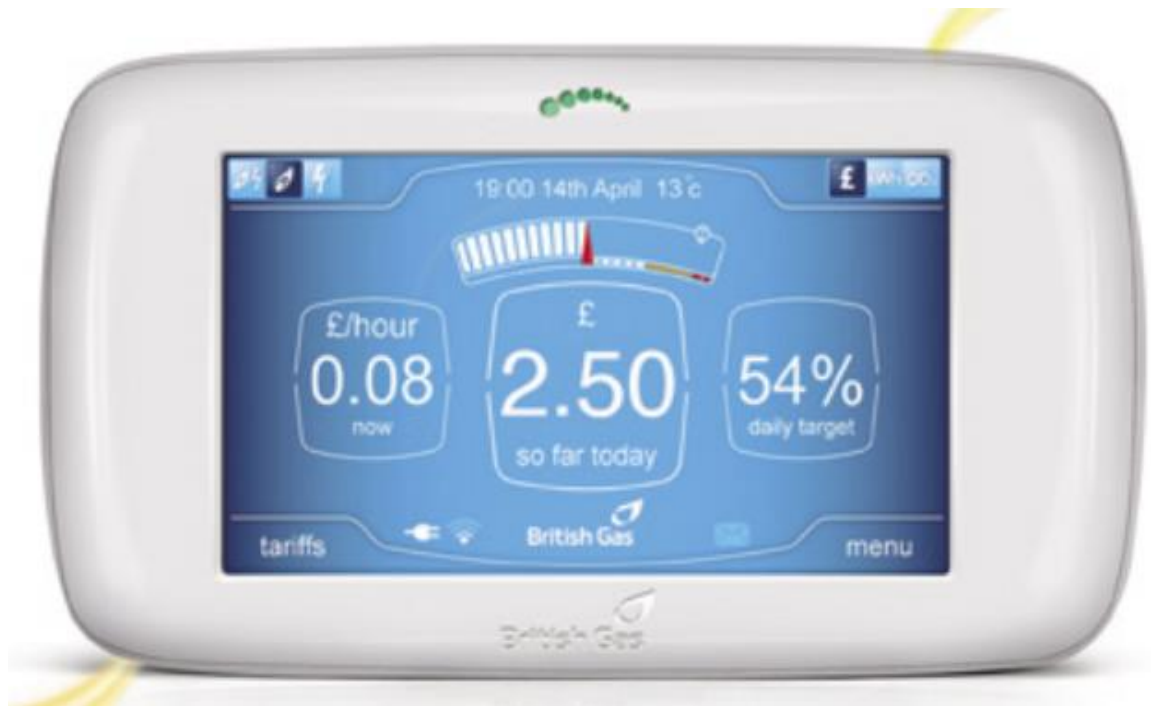
Figure 2.13. Pictorial example of an in home display connected to a smart meter showing current energy usage. (BritishGas, 2015).
