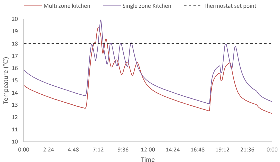
Figure 6.47 Comparison of kitchen temperature performance for the multi zone kitchen compared to single zone kitchen
